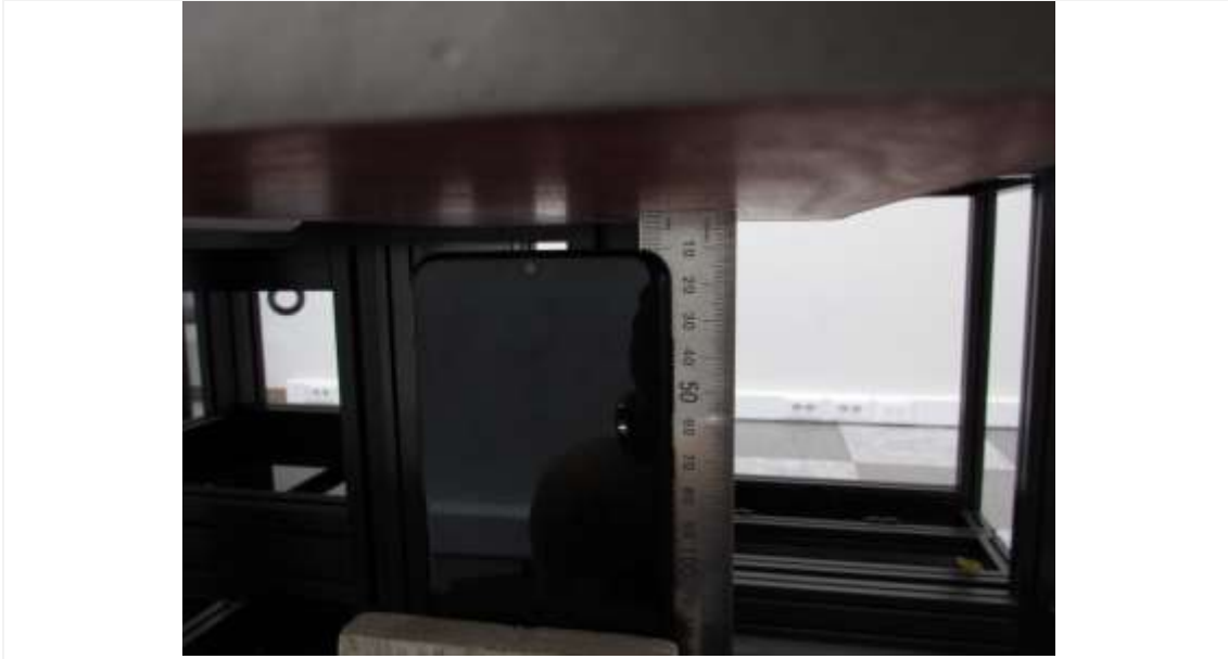
Distance of 10 mm from the EUT
