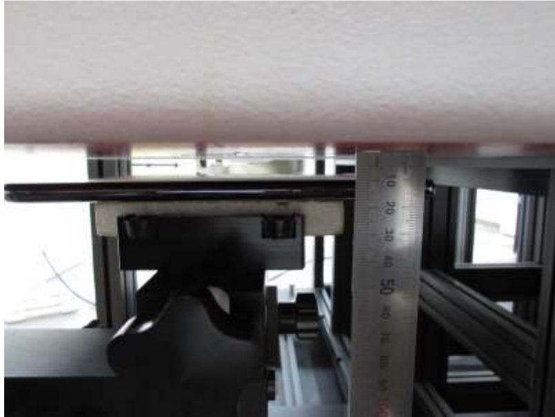
Distance of 10 mm from the EUT
