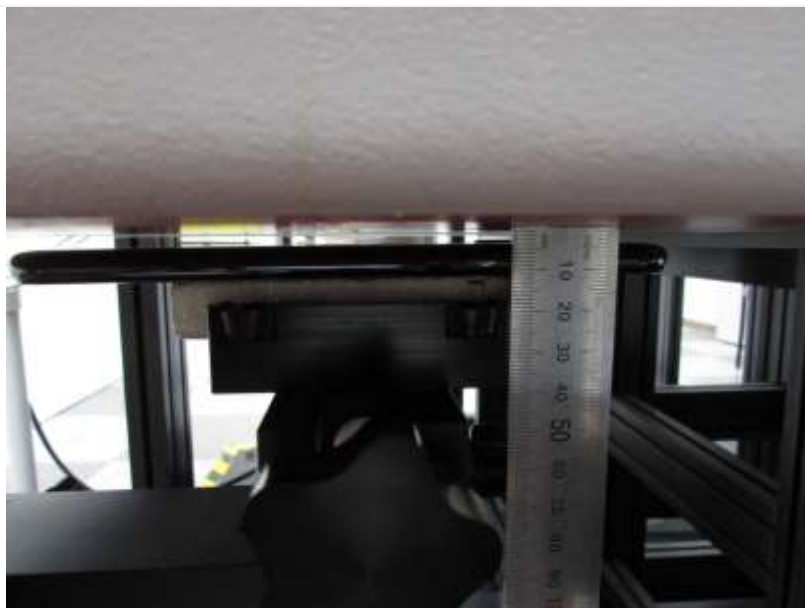
Distance of 4 mm from the EUT
