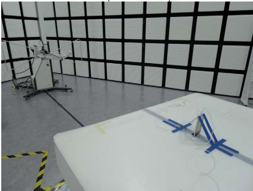
RADIATED BACK PHOTO (BELOW 1 GHz)
