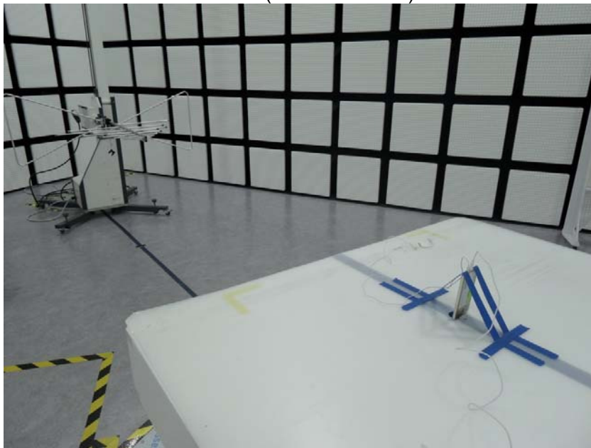
RADIATED FRONT PHOTO (BELOW 1 GHz)
