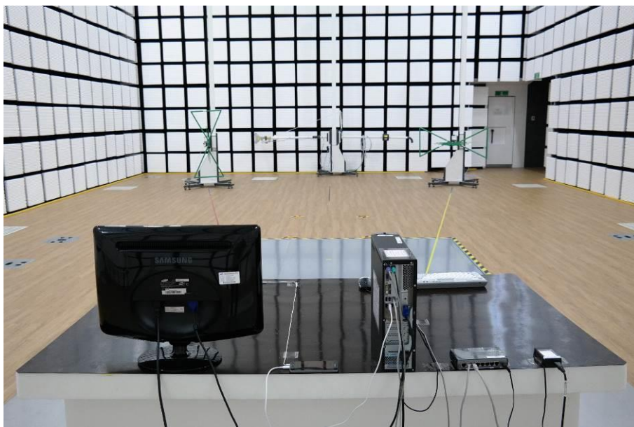
[ Radiated Disturbance for Below 1 GHz – Rear ]
