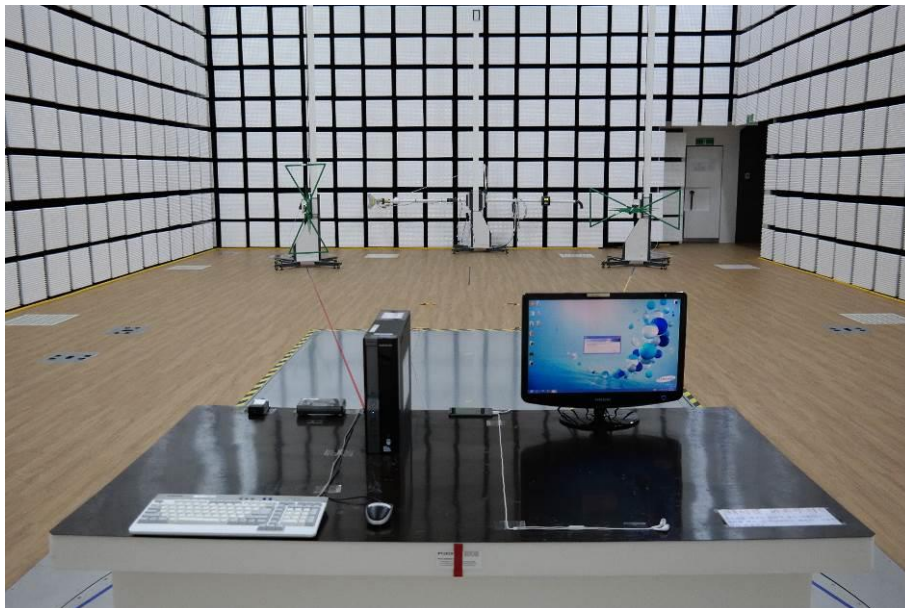
[ Radiated Disturbance for Below 1 GHz – Front ]
