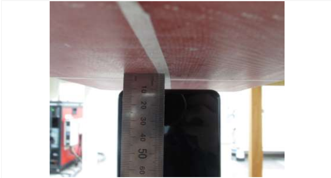
Distance of 10 mm from the EUT
