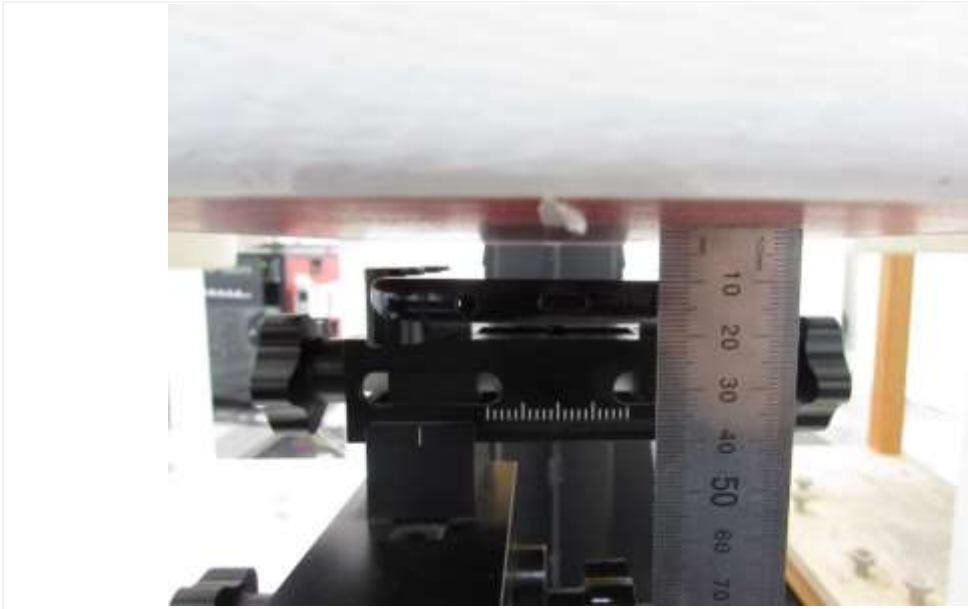
Distance of 10 mm from the EUT
