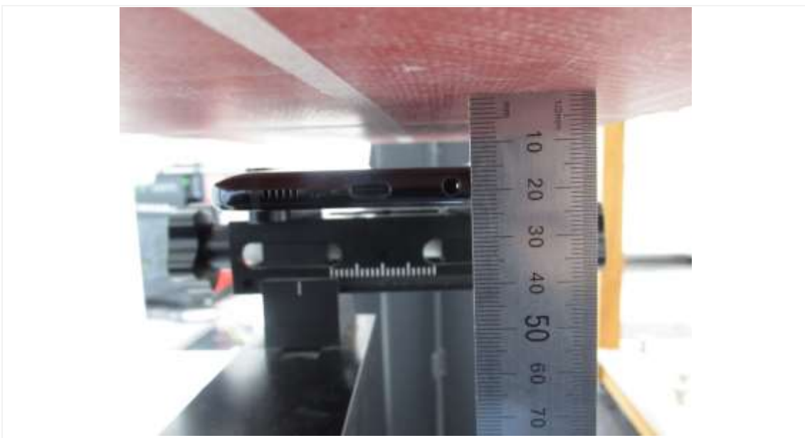
Distance of 15 mm from the EUT
