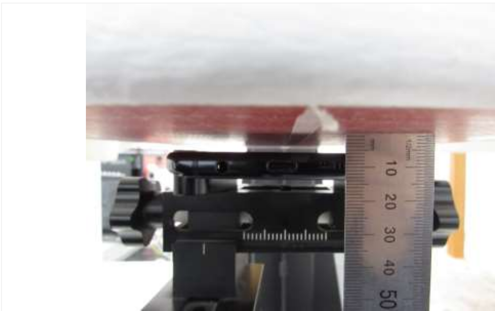
Distance of 6 mm from the EUT
