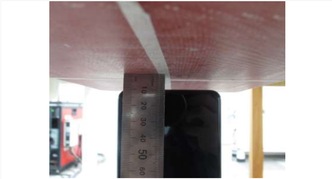
Distance of 10 mm from the EUT
