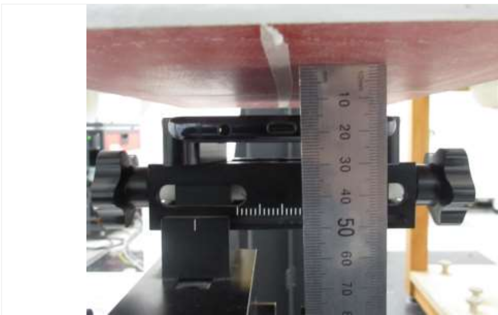
Distance of 15 mm from the EUT
