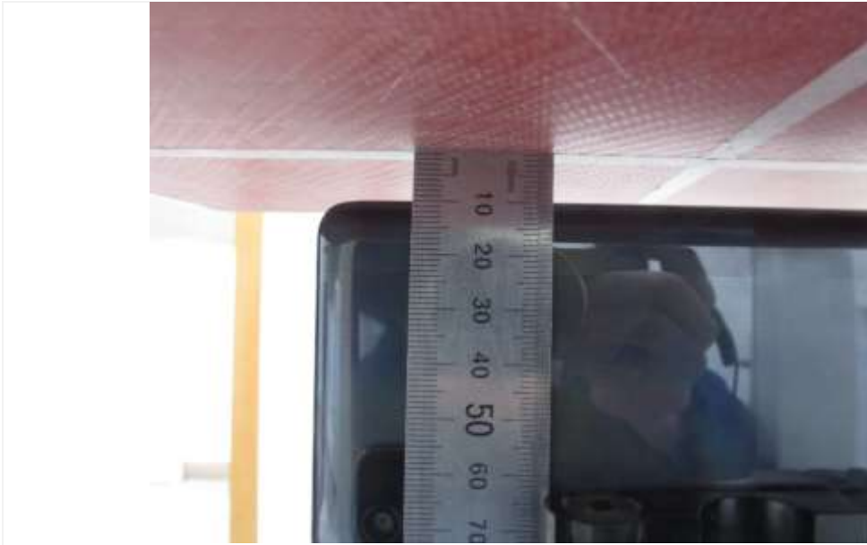
Distance of 10 mm from the EUT
