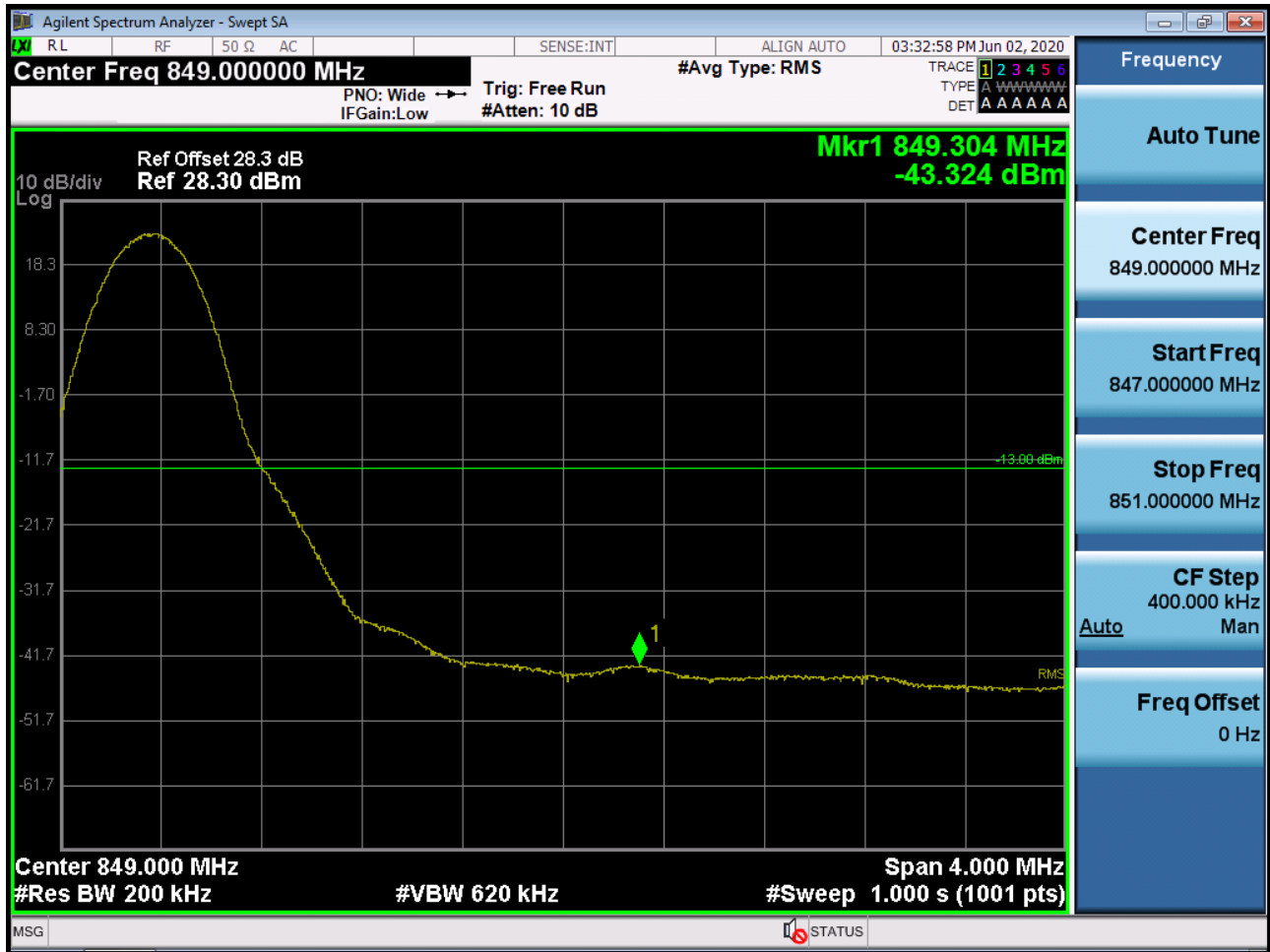
Sub6 n5. Upper Band Edge Plot (20M BW Ch.167800 BPSK_RB1_Offset 49)
