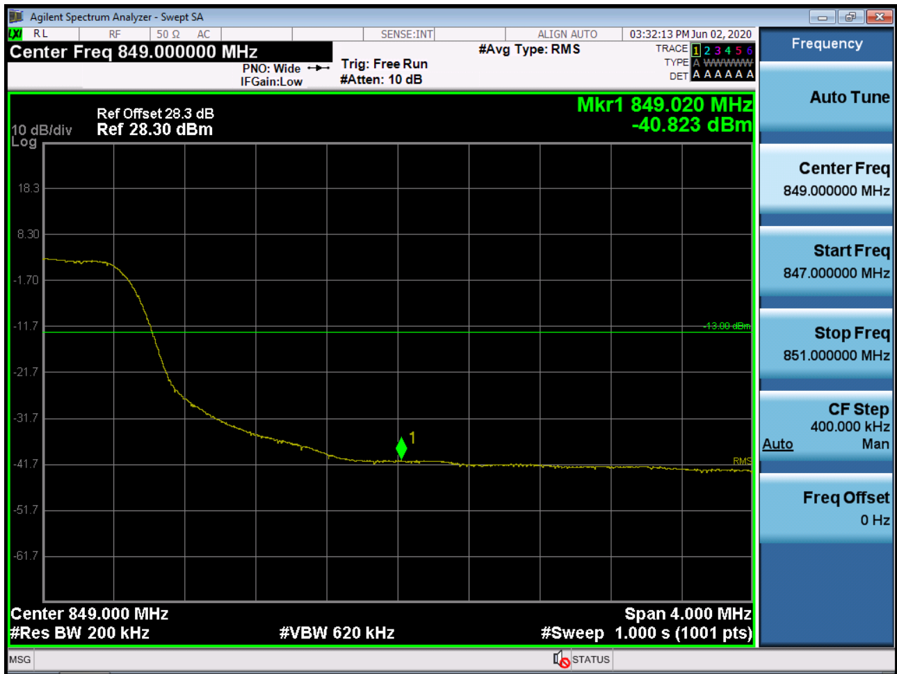
Sub6 n5. Upper Band Edge Plot (20M BW Ch.167800 BPSK_RB50_Offset 0)
