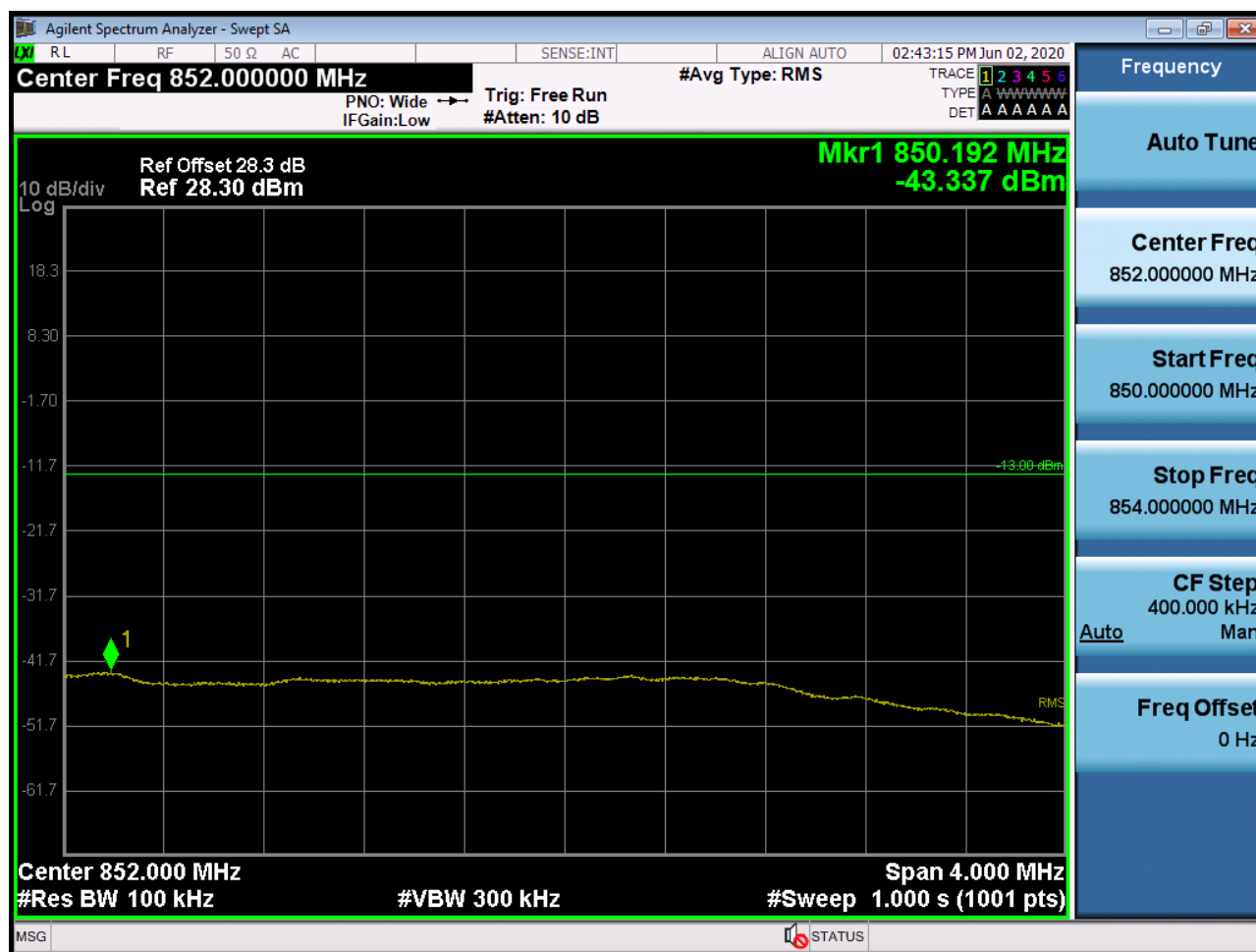
Sub6 n5. Upper Extended Band Edge Plot (10M BW Ch.168800 BPSK_RB15_0)
