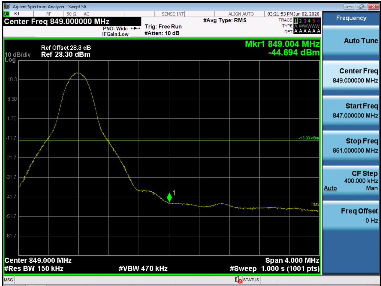
Sub6 n5. Upper Band Edge Plot (15M BW Ch.168300 BPSK_RB1_Offset 24)
