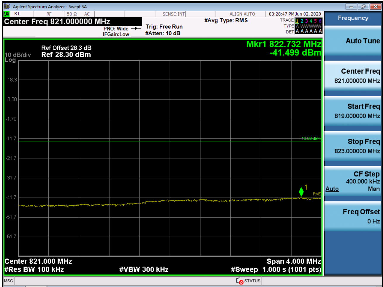
Sub6 n5. Lower Extended Band Edge Plot (20M BW Ch.166800 BPSK_RB50_0)
