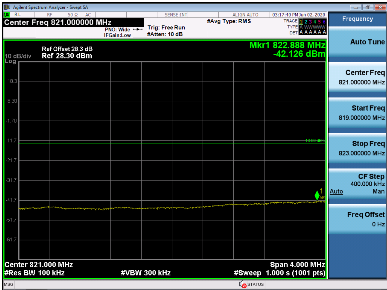
Sub6 n5. Lower Extended Band Edge Plot (15M BW Ch.166300 BPSK_RB25_0)
