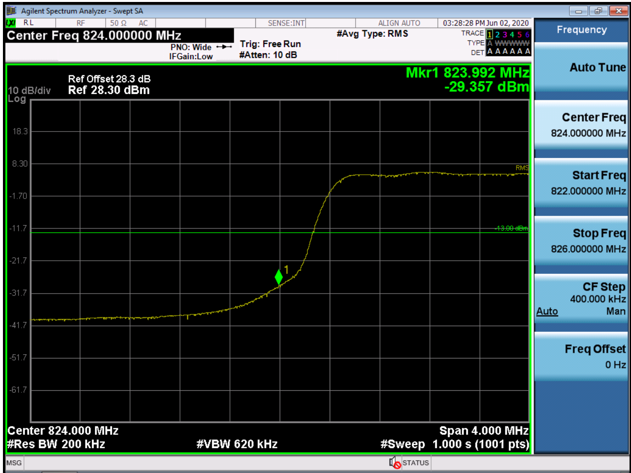
Sub6 n5. Lower Band Edge Plot (20M BW Ch.166800 BPSK_RB50_Offset 0)
