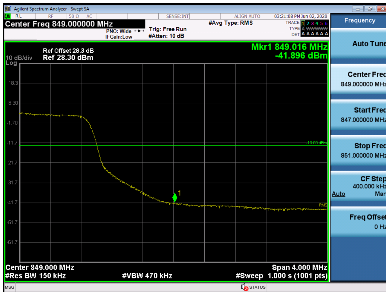
Sub6 n5. Upper Band Edge Plot (15M BW Ch.168300 BPSK_RB25_Offset 0)
