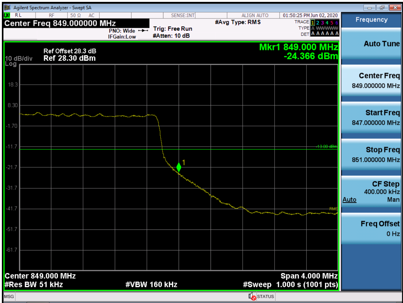
Sub6 n5. Upper Band Edge Plot (5M BW Ch.169300 BPSK_RB6_Offset 0)
