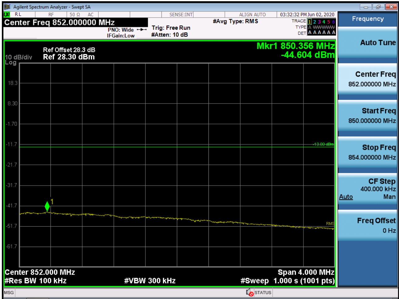
Sub6 n5. Upper Extended Band Edge Plot (20M BW Ch.167800 BPSK_RB50_0)
