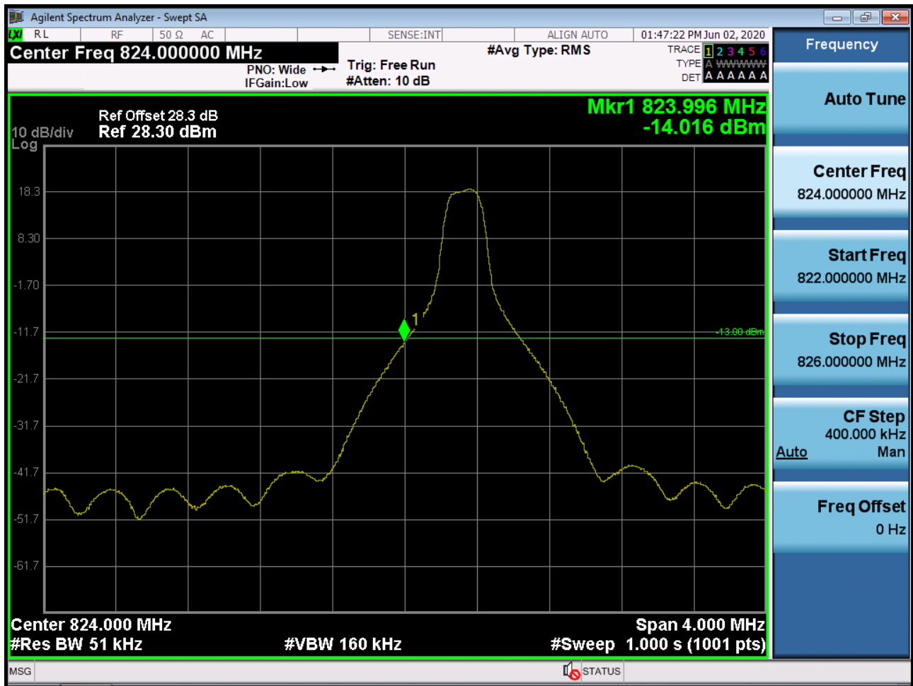
Sub6 n5. Lower Band Edge Plot (5M BW Ch.165300 BPSK_RB1_Offset 0)
