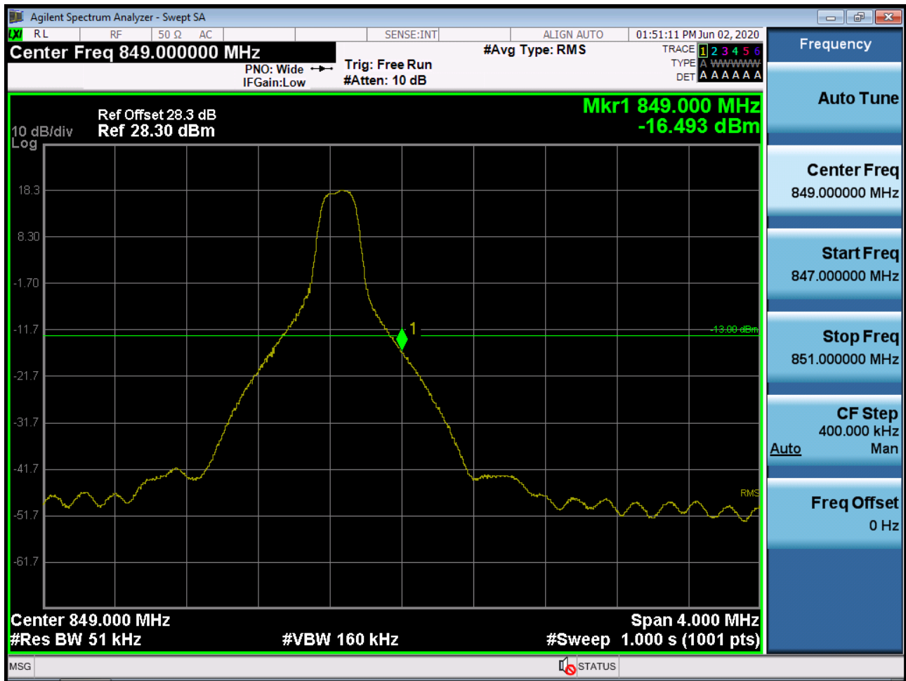
Sub6 n5. Upper Band Edge Plot (5M BW Ch.169300 BPSK_RB1_Offset 5)
