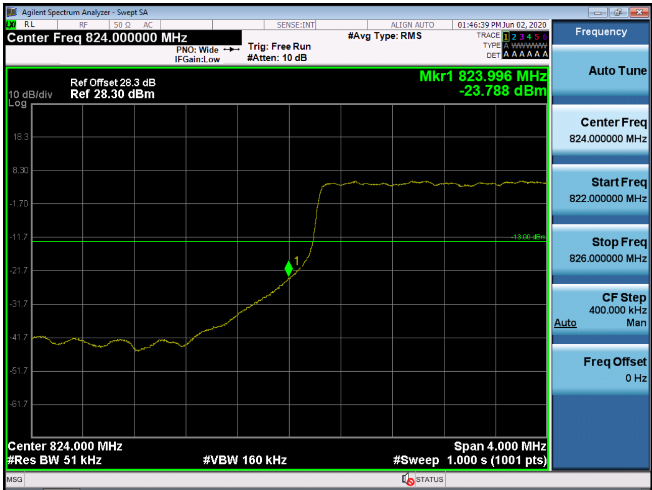
Sub6 n5. Lower Band Edge Plot (5M BW Ch.165300 BPSK_RB6_Offset 0)
