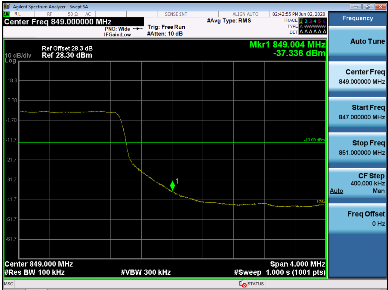
Sub6 n5. Upper Band Edge Plot (10M BW Ch.168800 BPSK_RB15_Offset 0)
