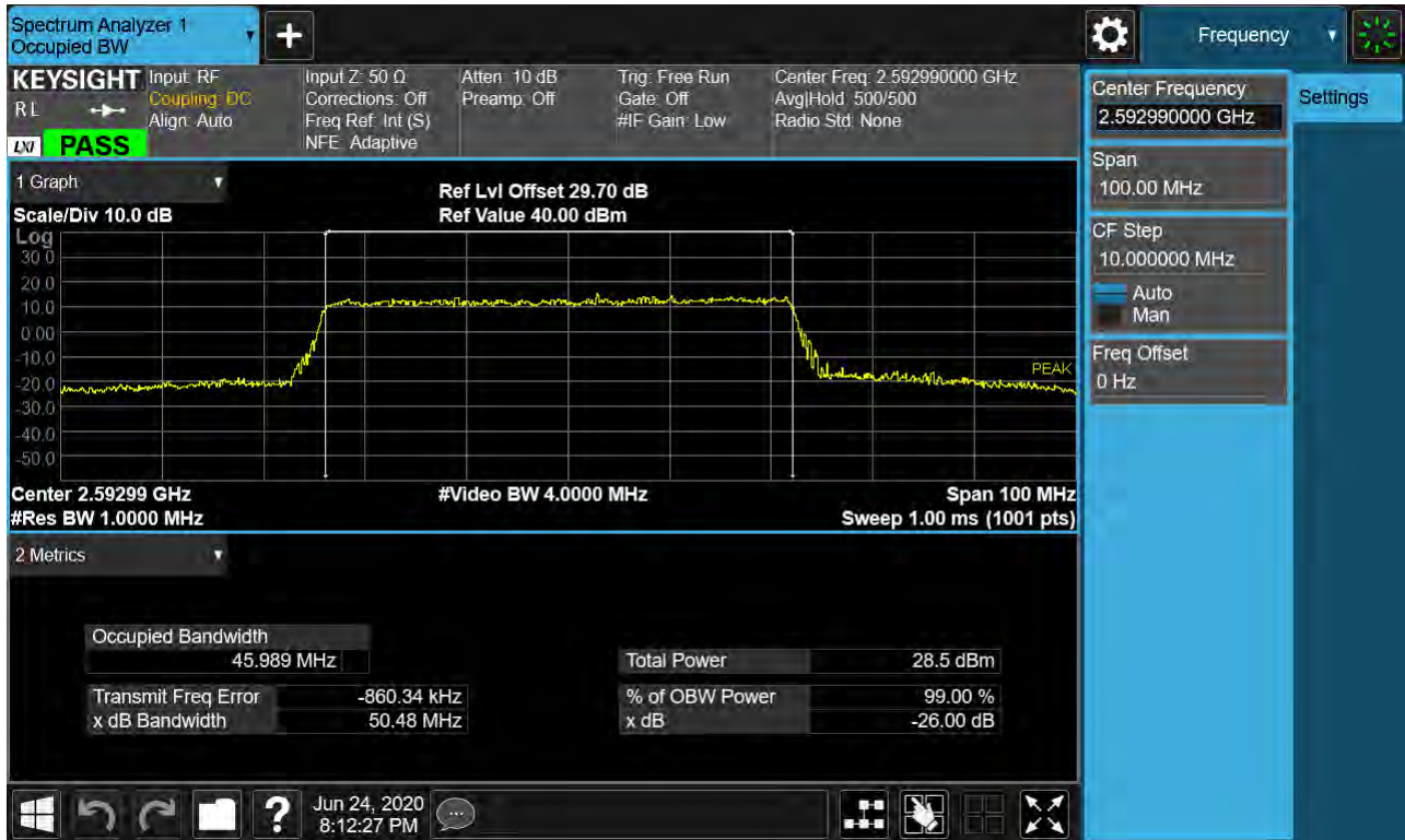
Sub6 n41. Occupied Bandwidth Plot (50 MHz Ch.518598 64-QAM RB 25)_SCS 30 kHz
