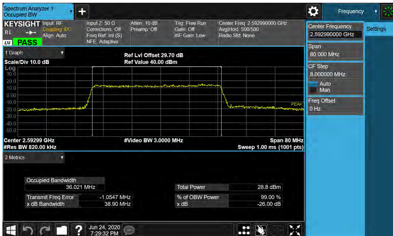
Sub6 n41. Occupied Bandwidth Plot (40 MHz Ch.518598 16-QAM RB 25)_SCS 30 kHz
