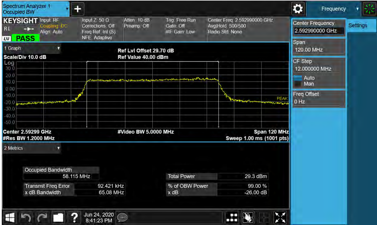
Sub6 n41. Occupied Bandwidth Plot (60 MHz Ch.518598 16-QAM RB 25)_SCS 30 kHz
