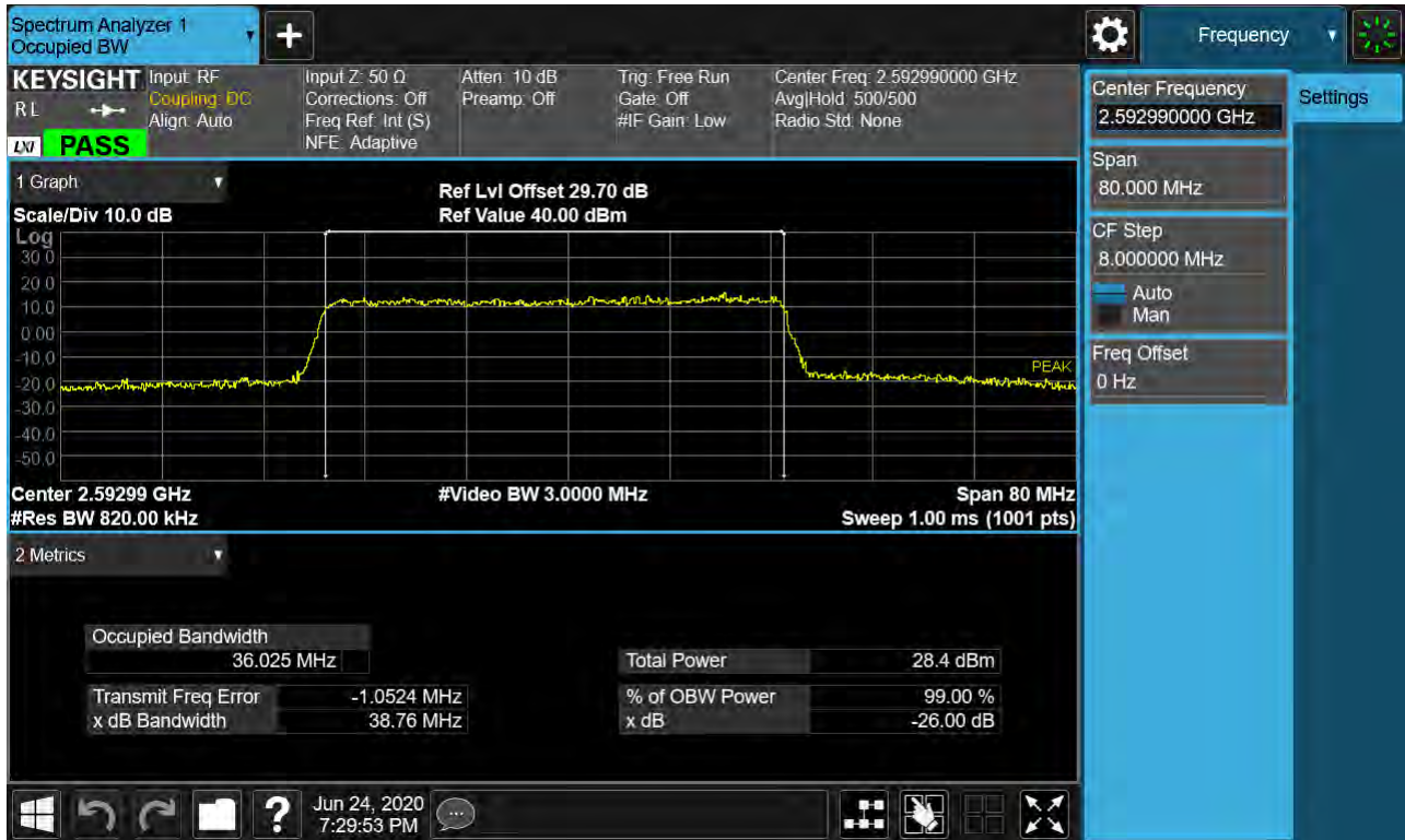
Sub6 n41. Occupied Bandwidth Plot (40 MHz Ch.518598 64-QAM RB 25)_SCS 30 kHz
