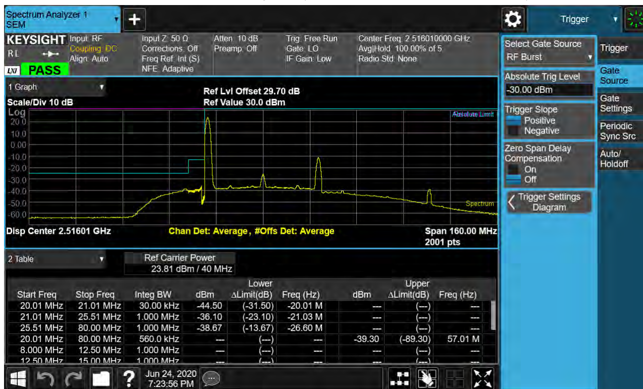
Sub6 n41. Low Channel Edge Plot (40 MHz Ch.503202 BPSK RB 1, Offset 0)-1
