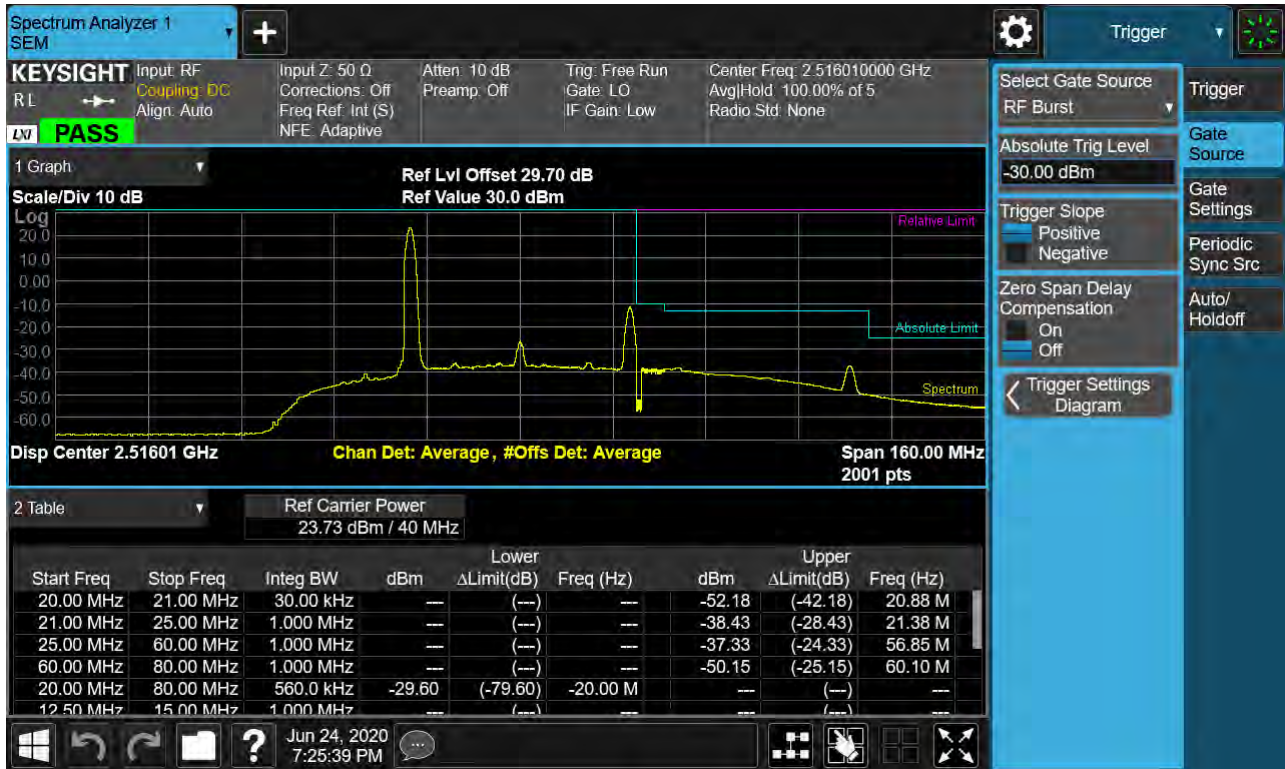
Sub6 n41. Low Channel Edge Plot (40 MHz Ch.503202 BPSK_RB1_Offset 0)-2
