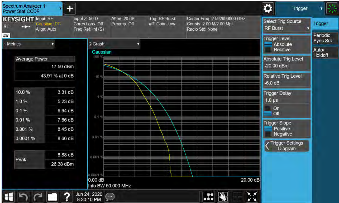
Sub6 n41. PAR Plot (50M BW_Ch.518598_256QAM_RB25_0)
