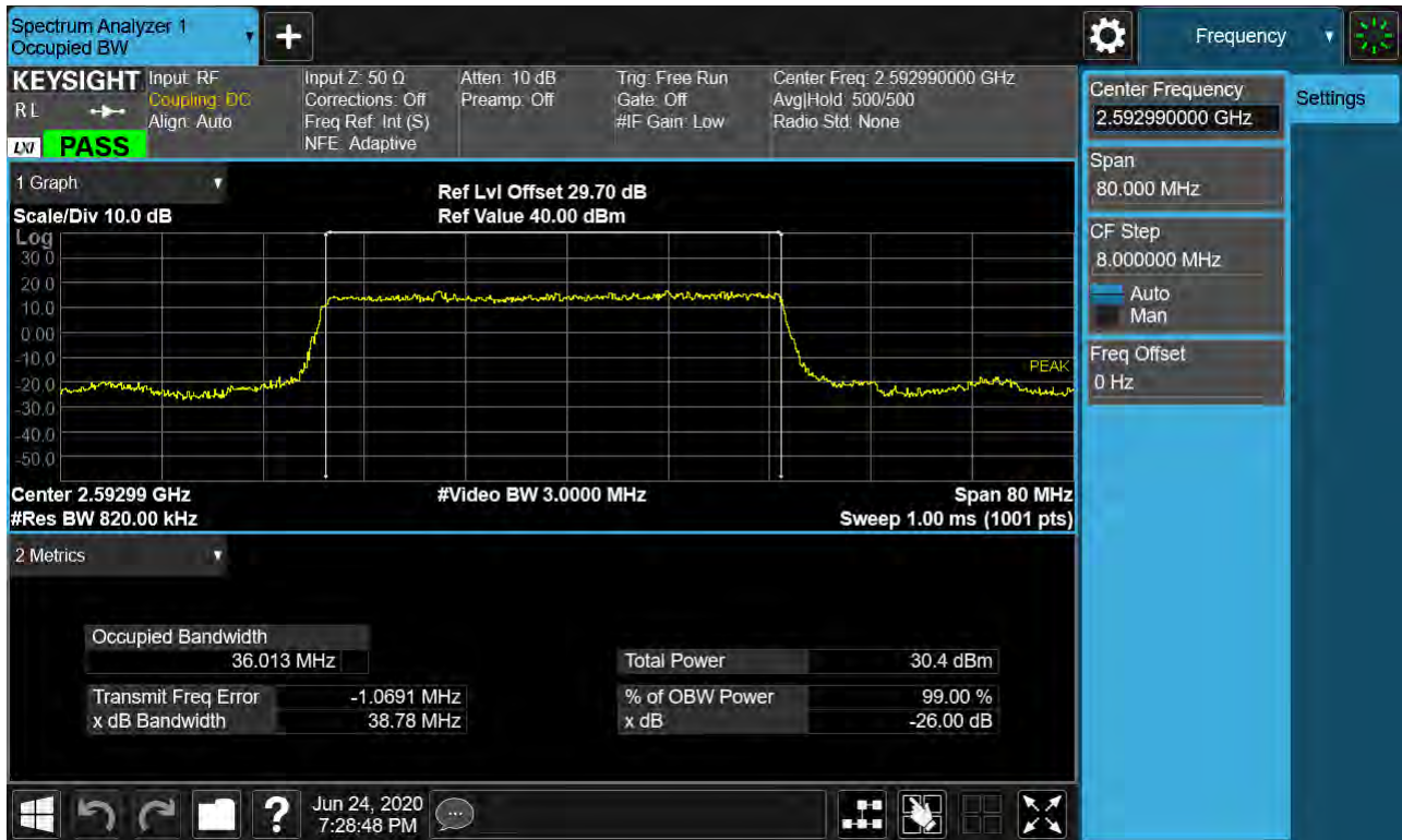
Sub6 n41. Occupied Bandwidth Plot (40 MHz Ch.518598 BPSK RB 25) _SCS 30 kHz
