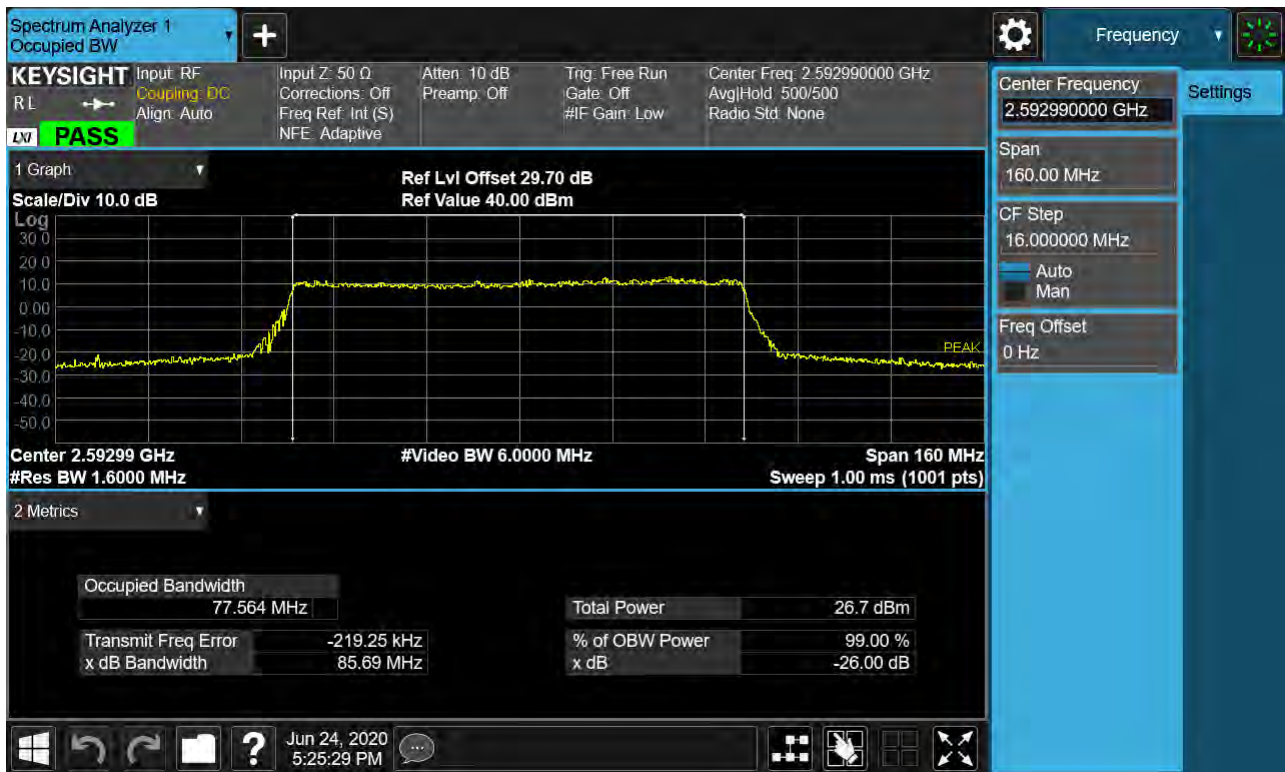
Sub6 n41. Occupied Bandwidth Plot (80 MHz Ch.518598 256-QAM RB 25) _SCS 30 kHz
