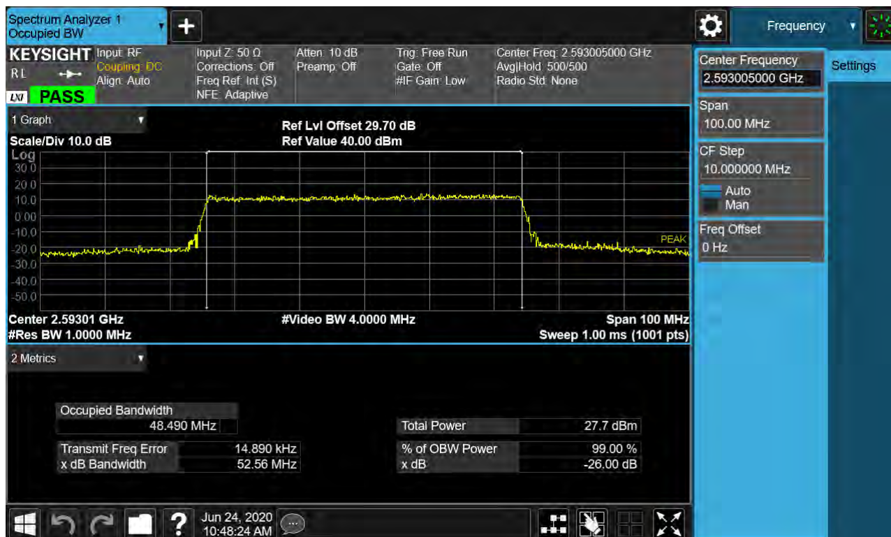
Sub6 n41. Occupied Bandwidth Plot (50 MHz Ch.518601 64-QAM RB 25)_SCS 15 kHz
