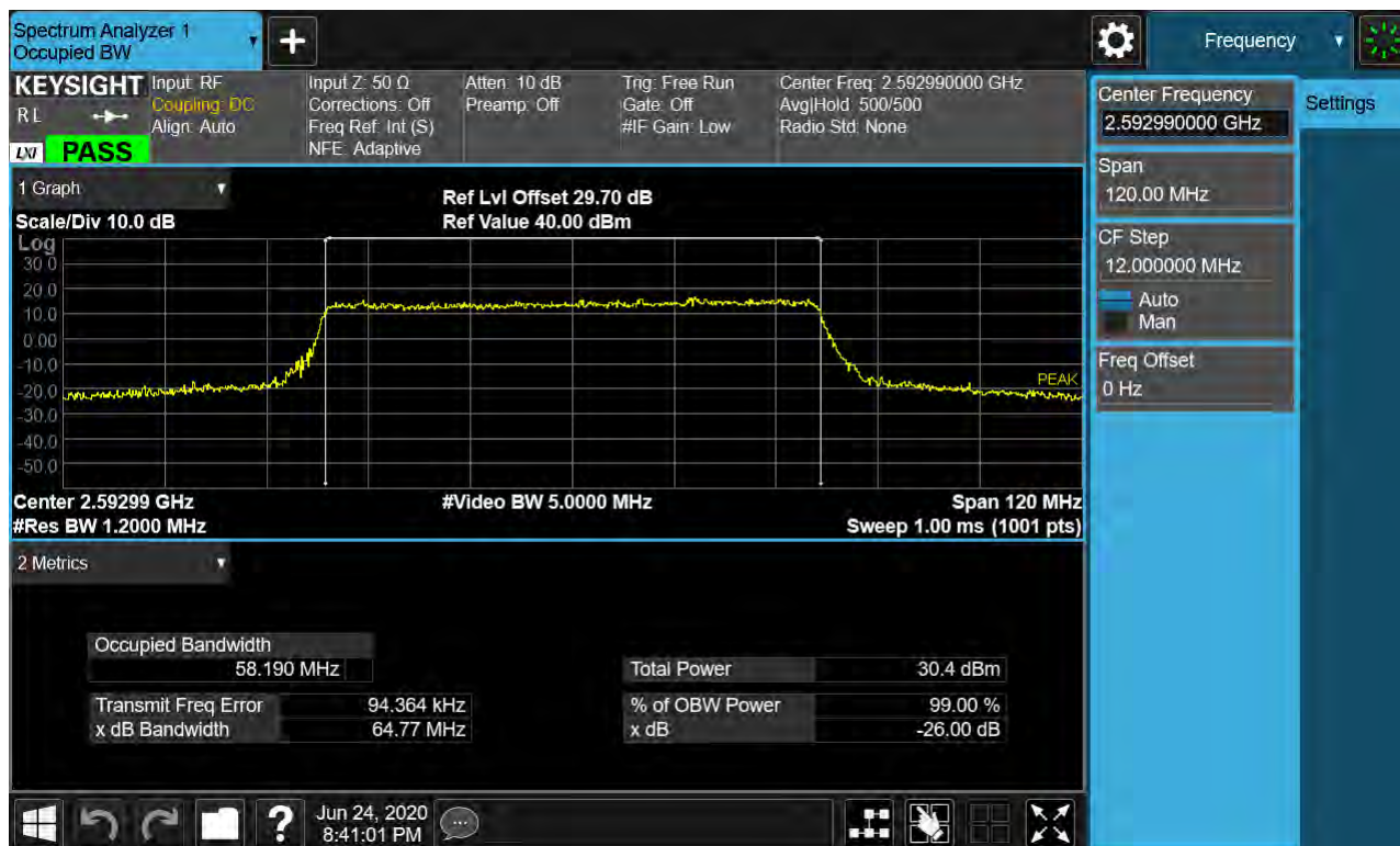
Sub6 n41. Occupied Bandwidth Plot (60 MHz Ch.518598 QPSK RB 25) _SCS 30 kHz
