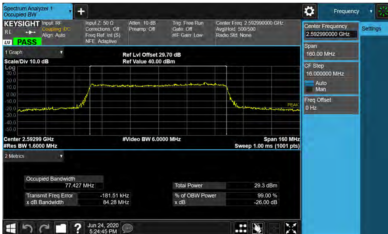
Sub6 n41. Occupied Bandwidth Plot (80 MHz Ch.518598 16-QAM RB 25)_SCS 30 kHz
