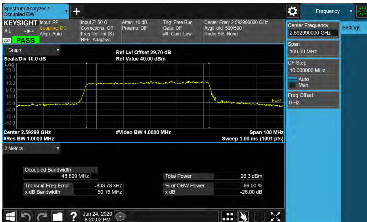
Sub6 n41. Occupied Bandwidth Plot (50 MHz Ch.518598 256-QAM RB 25) _SCS 30 kHz
