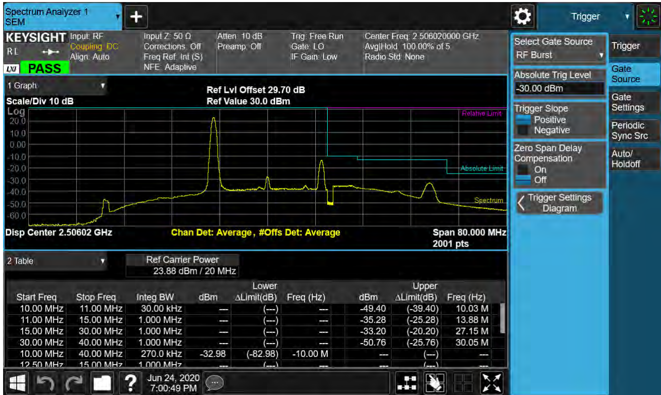
Sub6 n41. Low Channel Edge Plot (20 MHz Ch.501204 BPSK_RB1_Offset 0)-2
