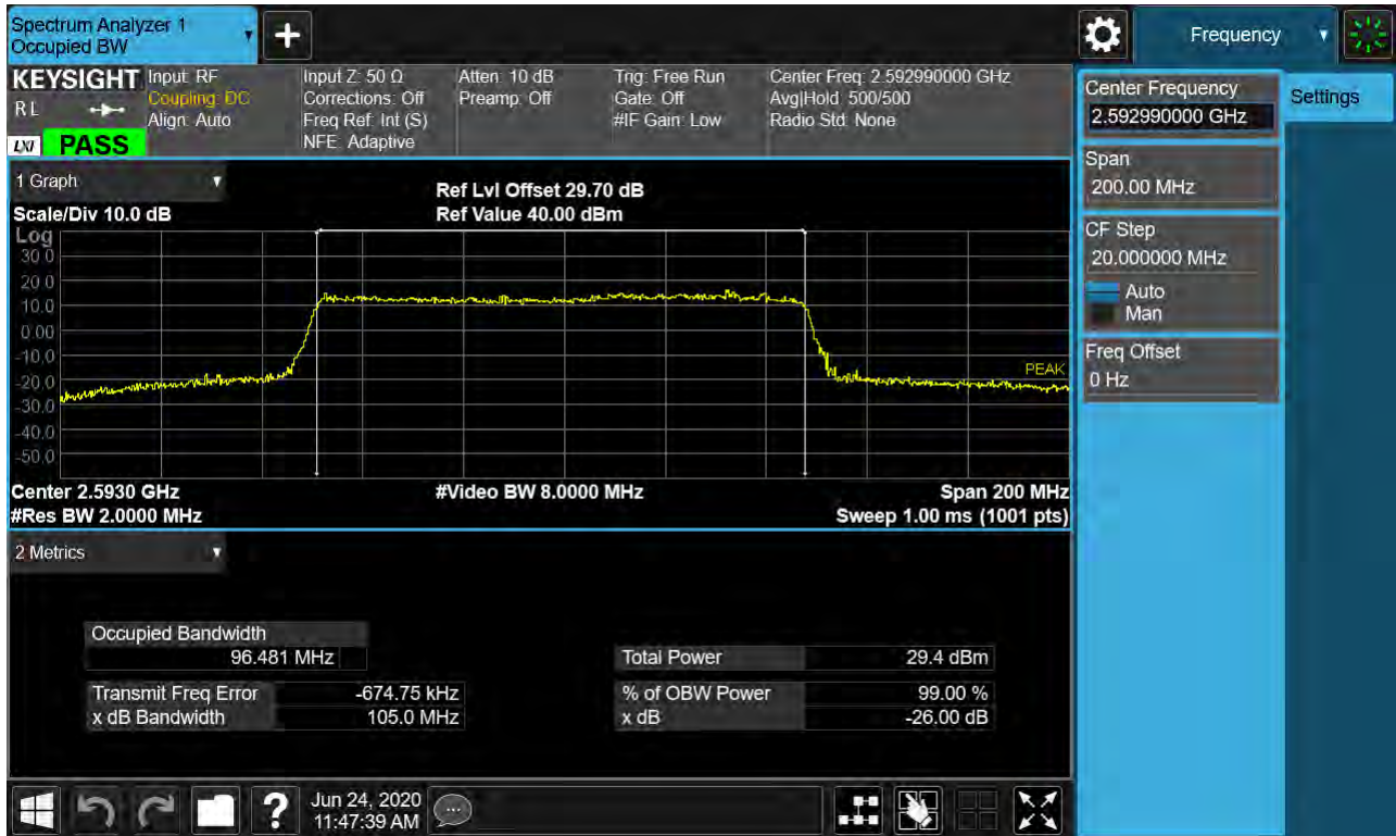
Sub6 n41. Occupied Bandwidth Plot (100 MHz Ch.518598 16-QAM RB 25) _SCS 30 kHz
