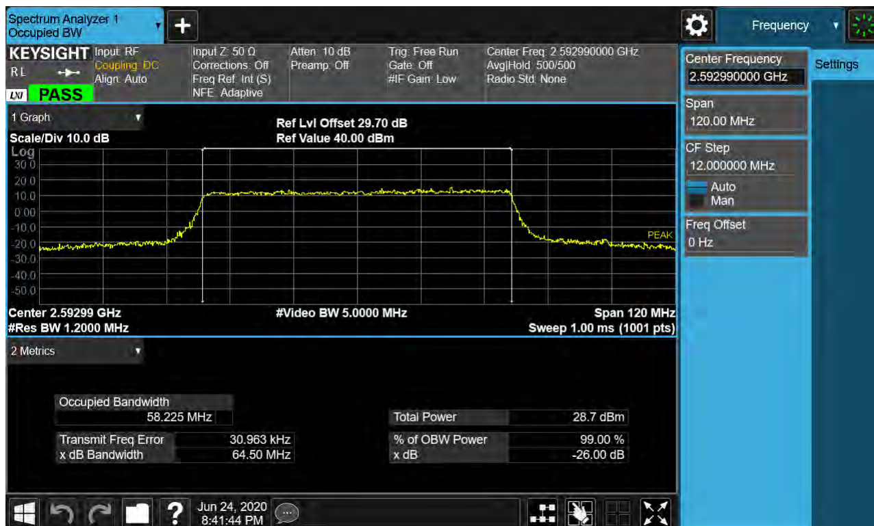
Sub6 n41. Occupied Bandwidth Plot (60 MHz Ch.518598 64-QAM RB 25)_SCS 30 kHz
