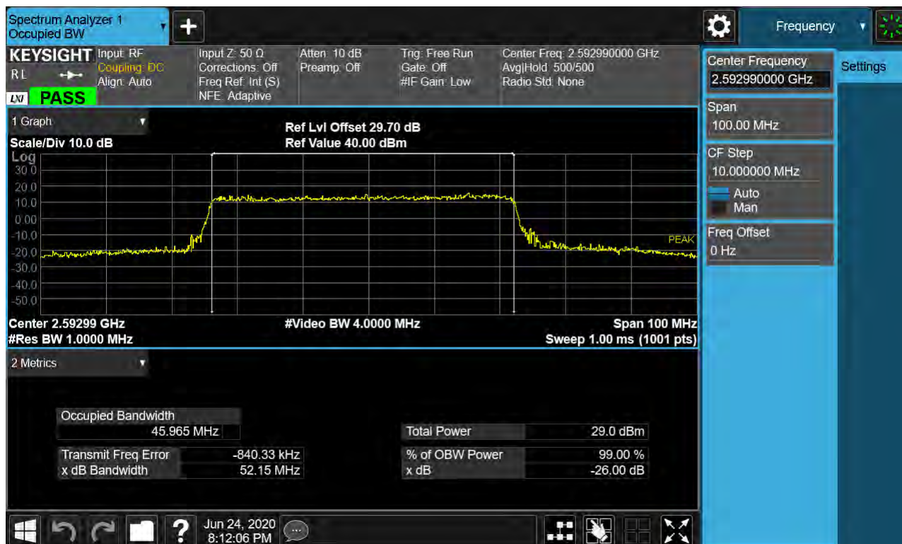
Sub6 n41. Occupied Bandwidth Plot (50 MHz Ch.518598 16-QAM RB 25)_SCS 30 kHz
