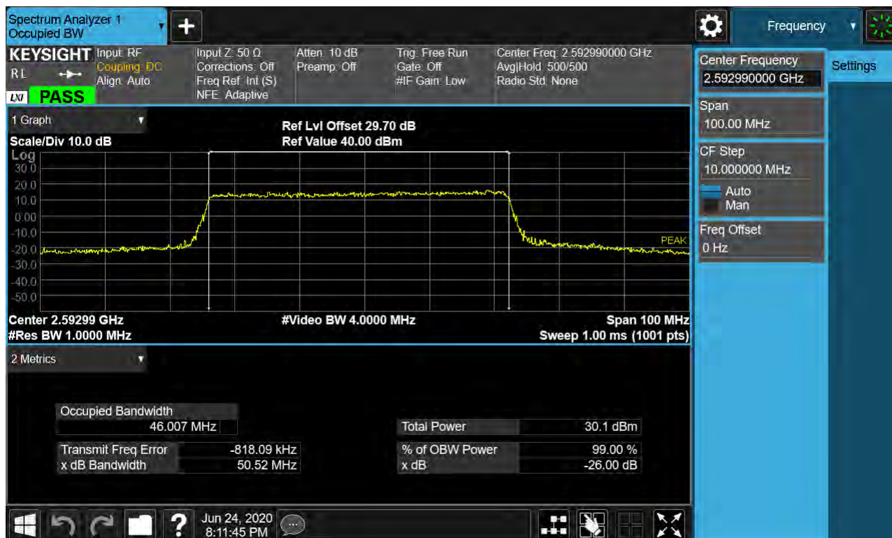
Sub6 n41. Occupied Bandwidth Plot (50 MHz Ch.518598 QPSK RB 25) _SCS 30 kHz
