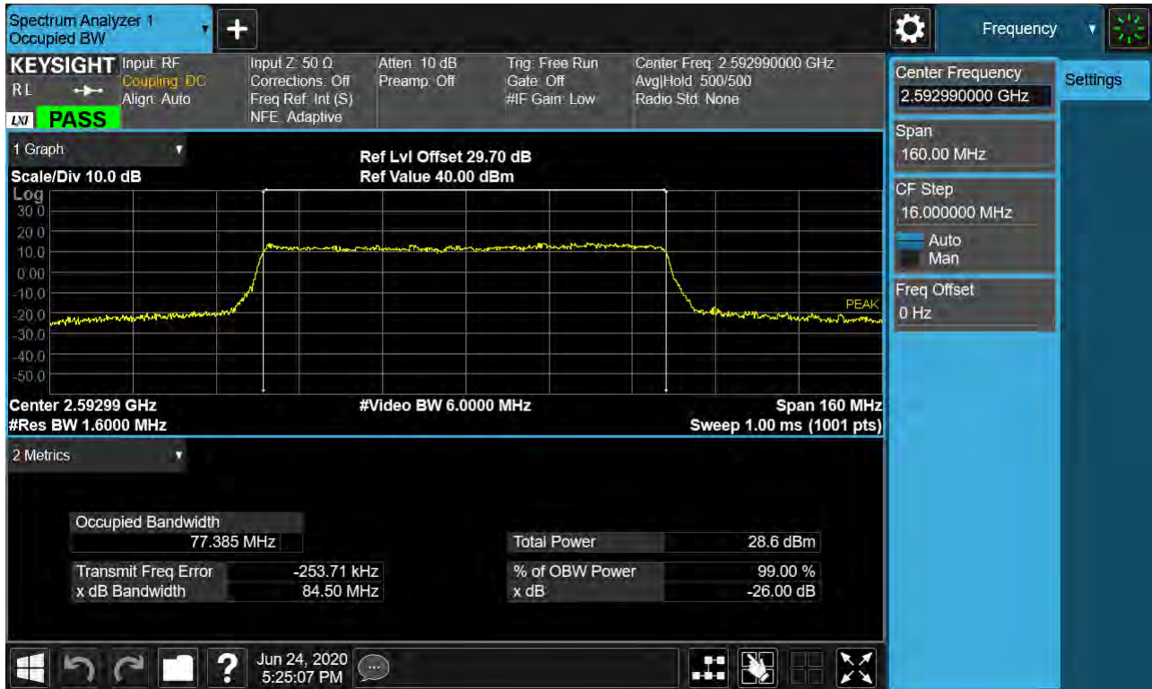
Sub6 n41. Occupied Bandwidth Plot (80 MHz Ch.518598 64-QAM RB 25)_SCS 30 kHz
