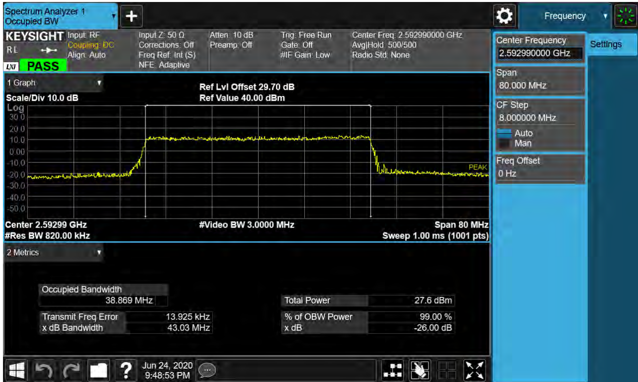
Sub6 n41. Occupied Bandwidth Plot (40 MHz Ch.518601 64-QAM RB 25)_SCS 15 kHz
