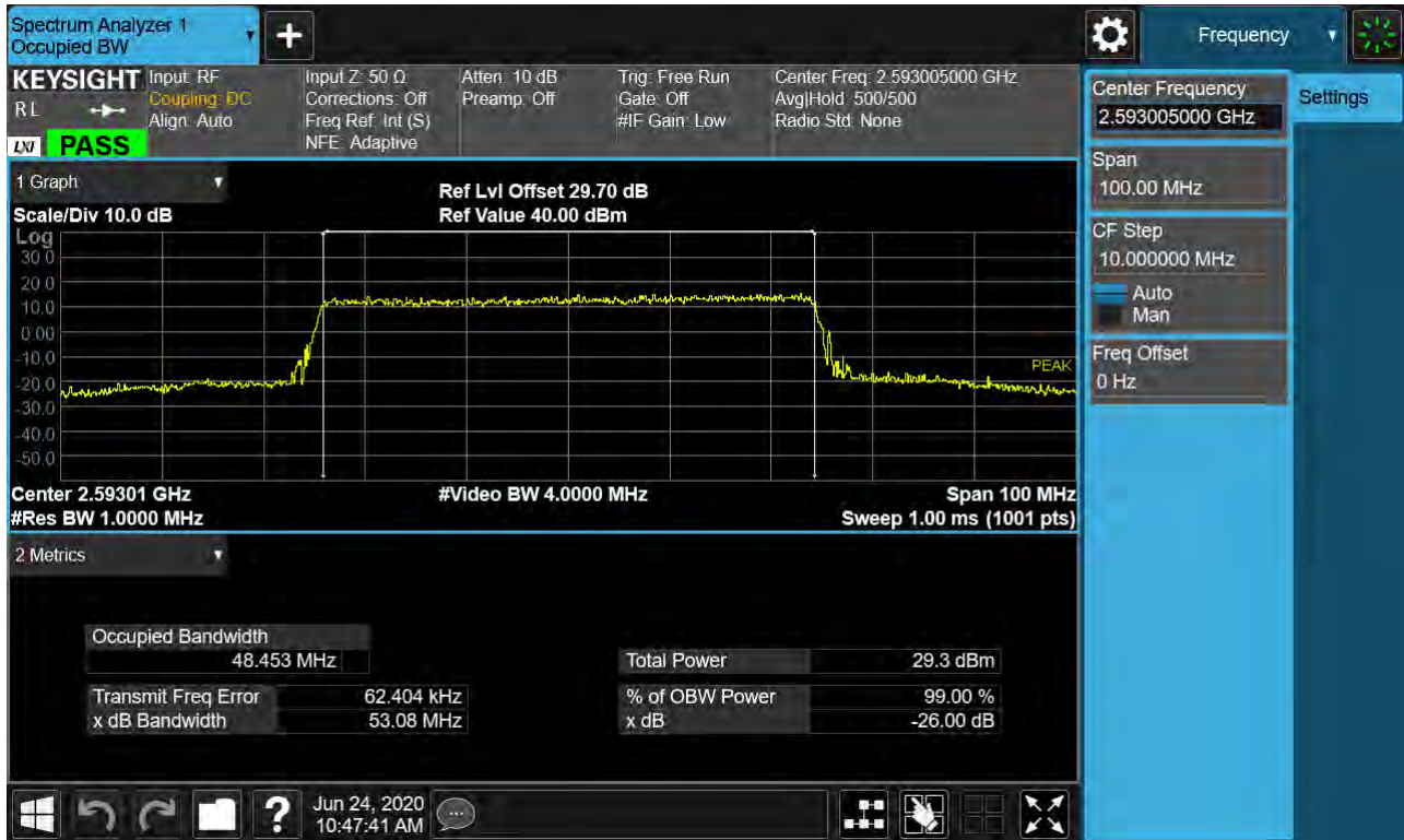
Sub6 n41. Occupied Bandwidth Plot (50 MHz Ch.518601 QPSK RB 25) _SCS 15 kHz
