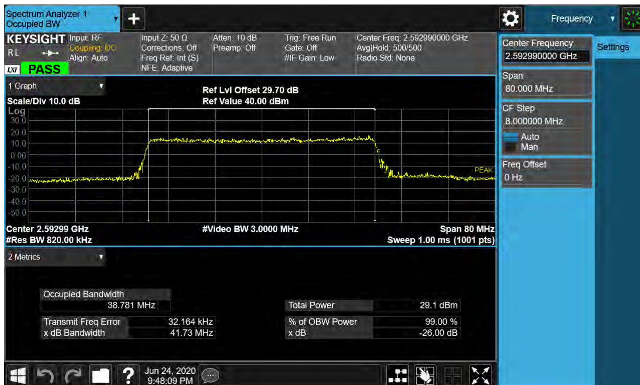
Sub6 n41. Occupied Bandwidth Plot (40 MHz Ch.518601 QPSK RB 25) _SCS 15 kHz
