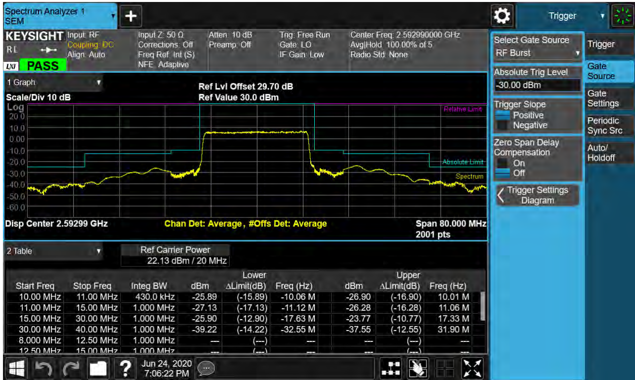
Sub6 n41. Mid Channel Edge Plot (20 MHz Ch.518598 BPSK RB 25)
