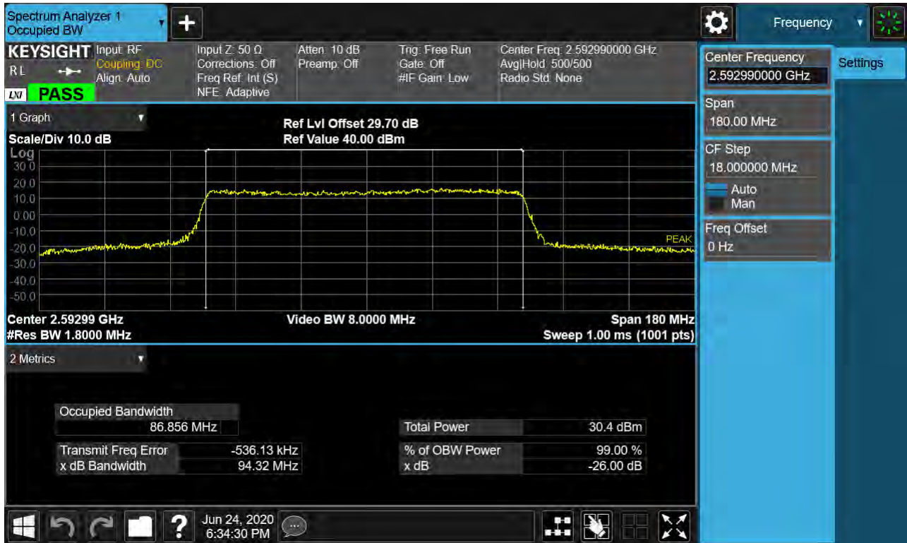
Sub6 n41. Occupied Bandwidth Plot (90 MHz Ch.518598 QPSK RB 25) _SCS 30 kHz
