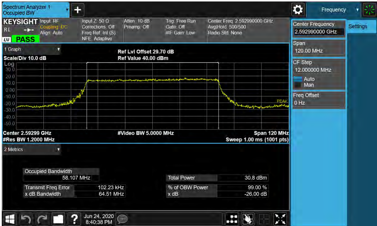
Sub6 n41. Occupied Bandwidth Plot (60 MHz Ch.518598 BPSK RB 25) _SCS 30 kHz
