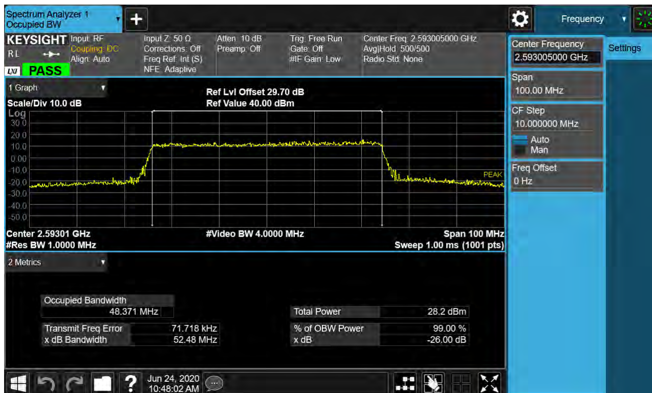
Sub6 n41. Occupied Bandwidth Plot (50 MHz Ch.518601 16-QAM RB 25)_SCS 15 kHz
