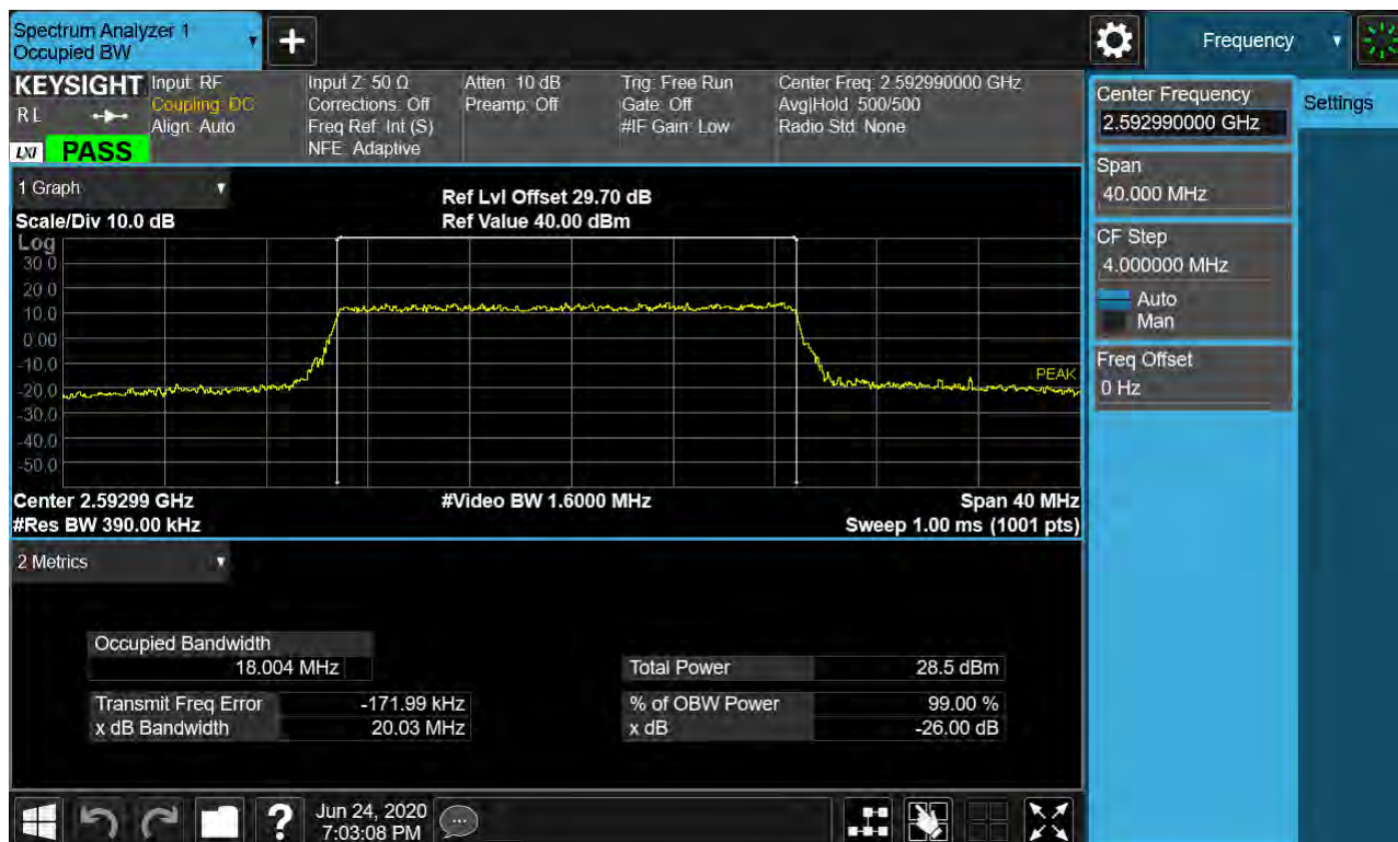
Sub6 n41. Occupied Bandwidth Plot (20 MHz Ch.518598 16-QAM RB 25)_SCS 30 kHz
