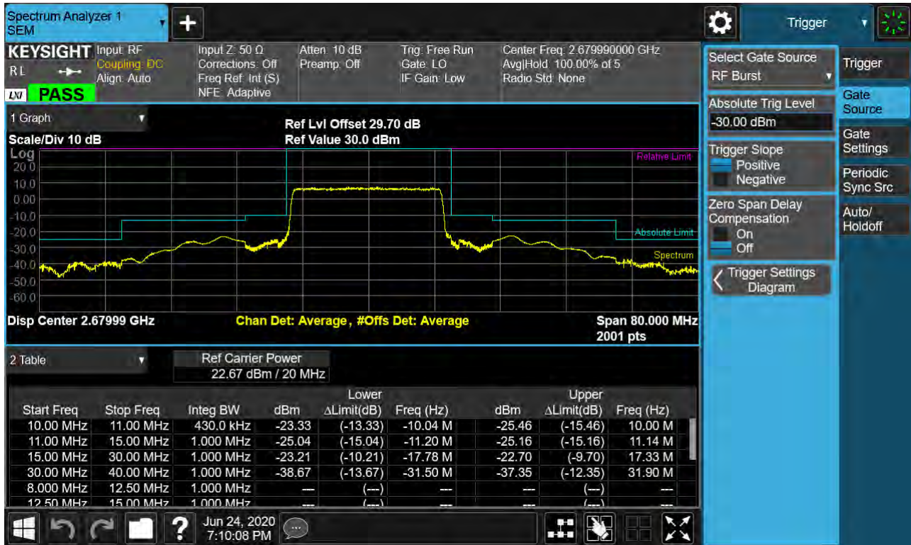
Sub6 n41. High Channel Edge Plot (20 MHz Ch.535998 BPSK_RB25_Offset 0)
