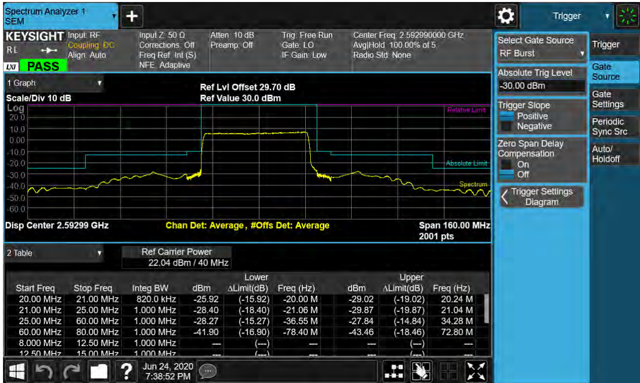
Sub6 n41. Mid Channel Edge Plot (40 MHz Ch.518598 BPSK RB 25)
