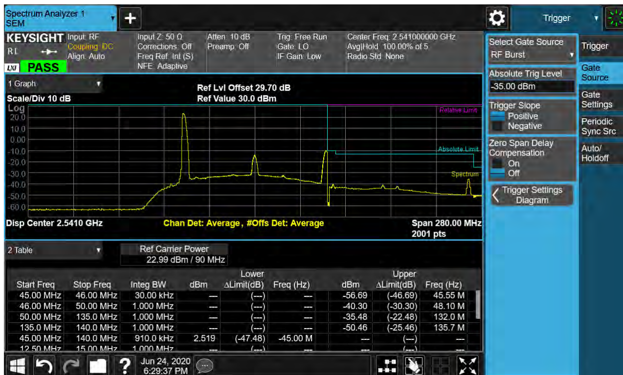
Sub6 n41. Low Channel Edge Plot (90 MHz Ch.508200 BPSK_RB1_Offset 0)-2
