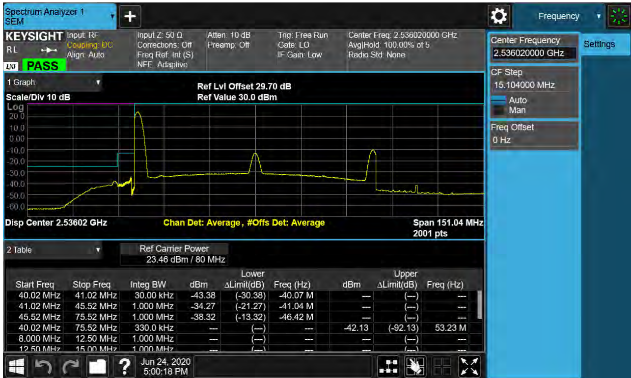
Sub6 n41. Low Channel Edge Plot (80 MHz Ch.507204 BPSK RB 1, Offset 0)-1
