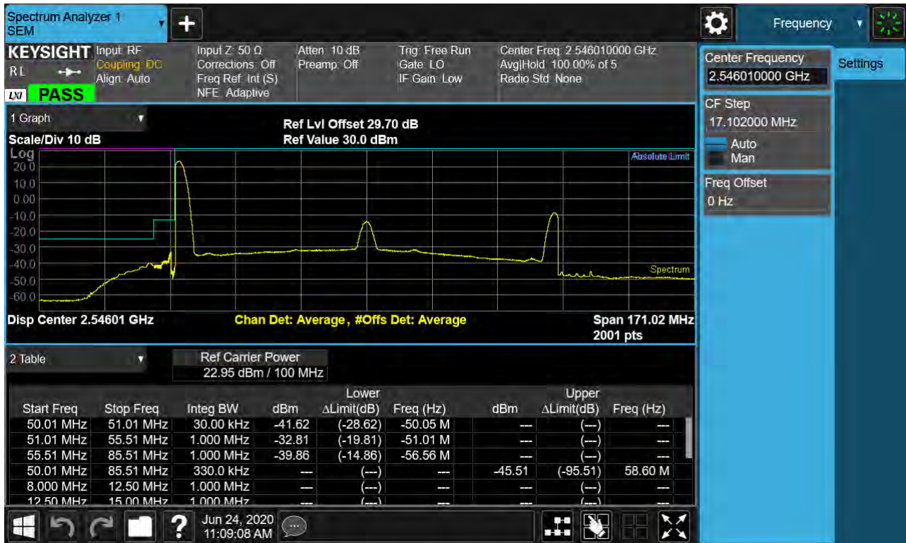
Sub6 n41. Low Channel Edge Plot (100 MHz Ch.509202 BPSK RB 1, Offset 0)-1
