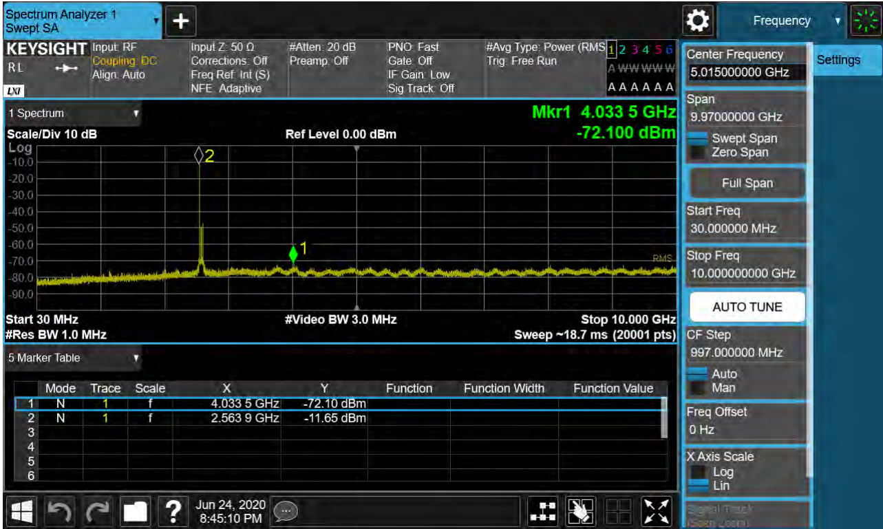
Sub6 n41. Conducted Spurious Plot 1 (60 MHz Ch.518598 BPSK RB 1, Offset 0)
