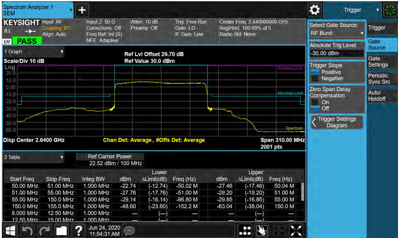
Sub6 n41. High Channel Edge Plot (100 MHz Ch.528000 BPSK_RB25_Offset 0)
