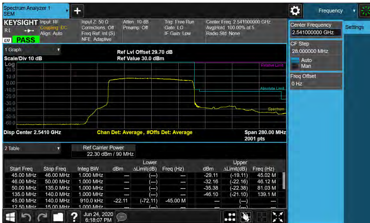
Sub6 n41. Low Channel Edge Plot (90 MHz Ch.508200 BPSK_RB25_Offset 0)-2
