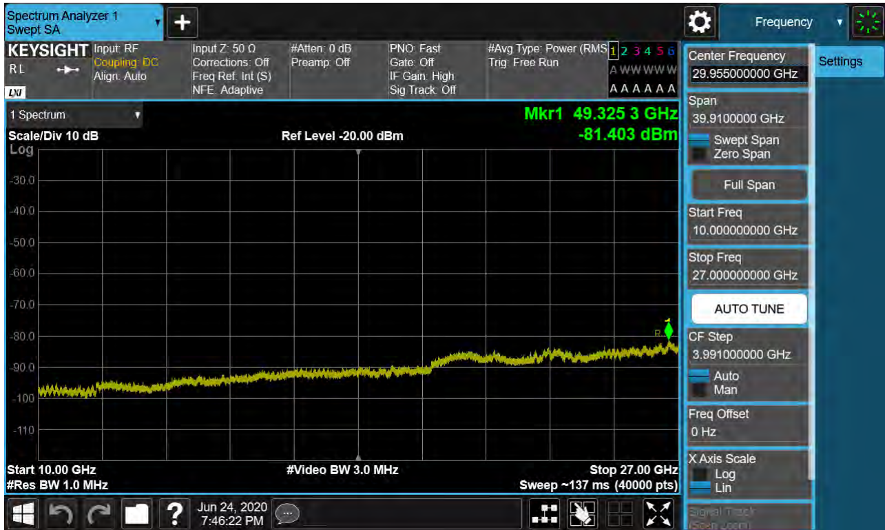
Sub6 n41. Conducted Spurious Plot 2 (40 MHz Ch.534000 BPSK RB 1, Offset 0)
