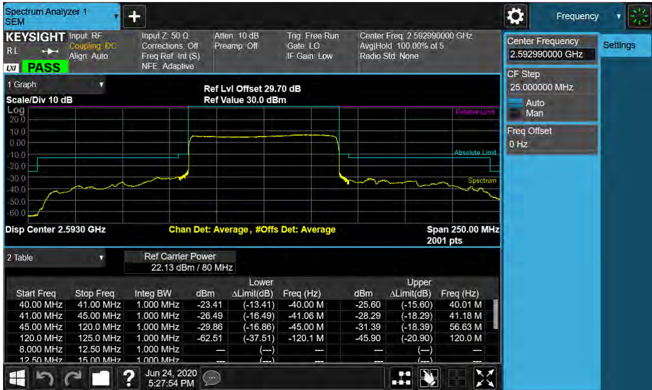
Sub6 n41. Mid Channel Edge Plot (80 MHz Ch.518598 BPSK RB 25)
