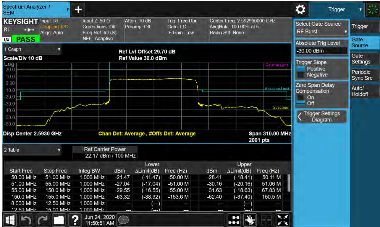
Sub6 n41. Mid Channel Edge Plot (100 MHz Ch.518598 BPSK RB 25)
