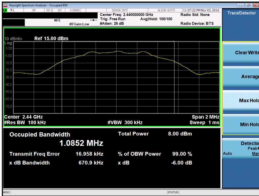
Plot 7-2. 6dB Bandwidth Plot (Bluetooth (LE) – Ch. 19)
