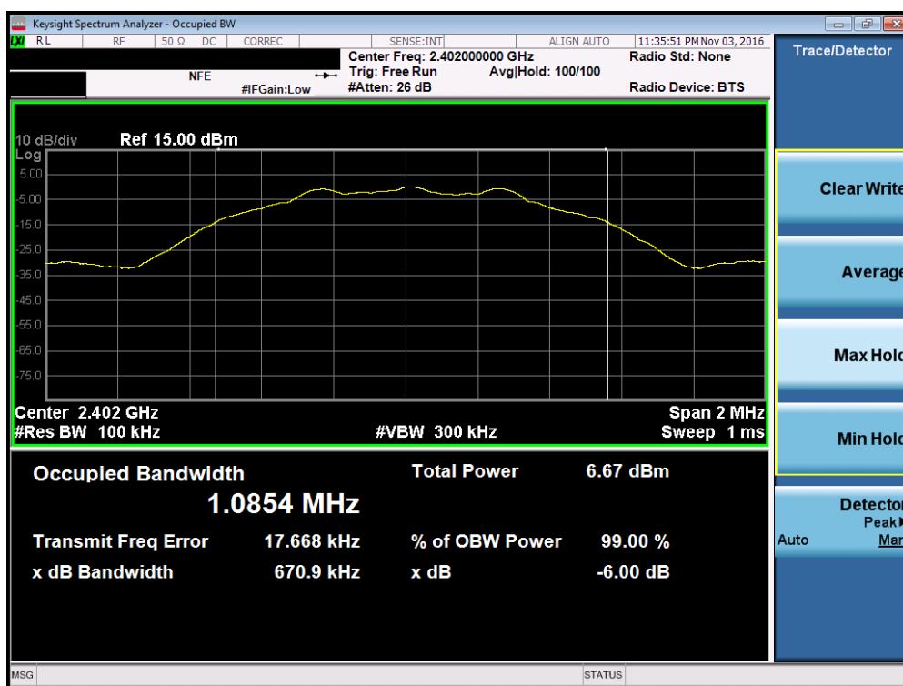
Plot 7-1. 6dB Bandwidth Plot (Bluetooth (LE) – Ch. 0)
