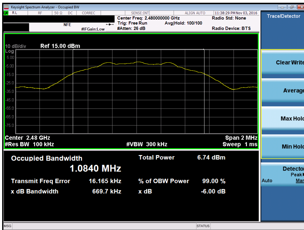
Plot 7-3. 6dB Bandwidth Plot (Bluetooth (LE) – Ch. 39)
