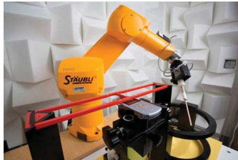
Figure 4-3 SPEAG Robotic System
