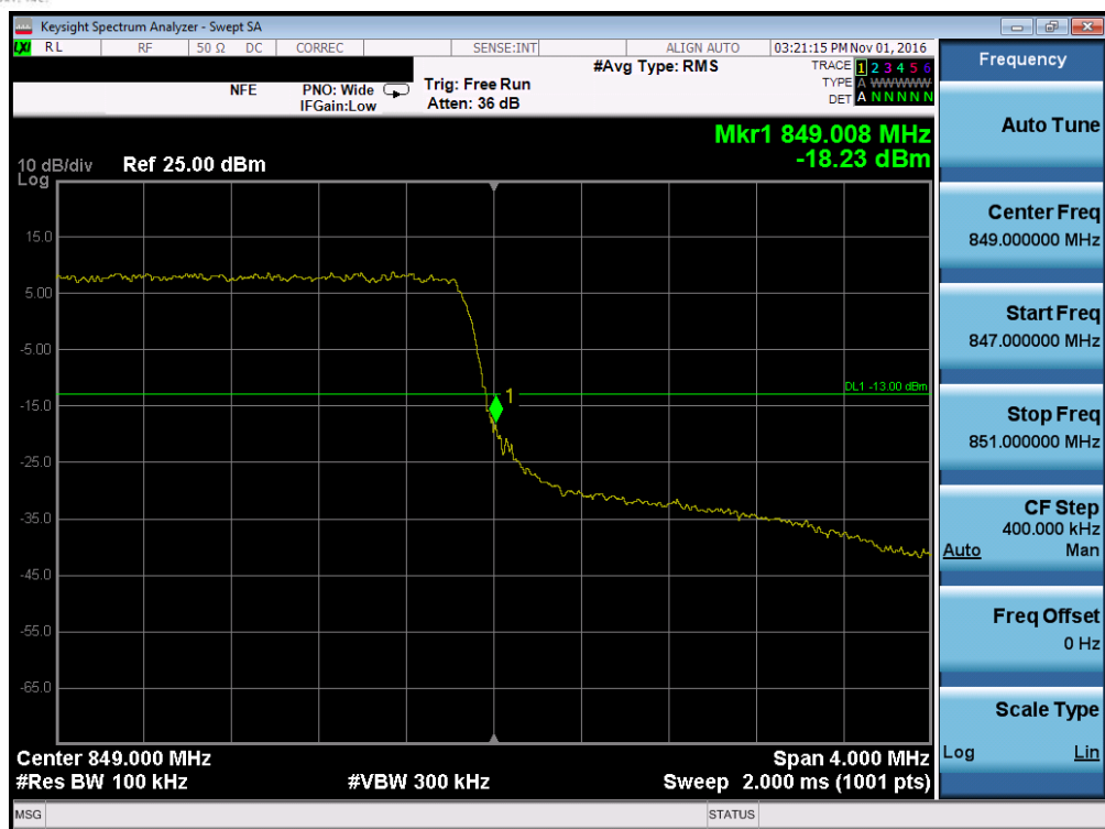
Plot 7-99. Upper Band Edge Plot (Band 5 – 3.0MHz QPSK – RB Size 15)
