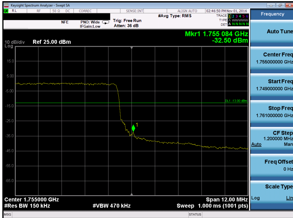
Plot 7-122. Upper Band Edge Plot (Band 4 – 15.0MHz QPSK – RB Size 75)
