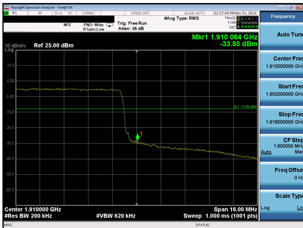
Plot 7-150. Upper Band Edge Plot (Band 2 – 20.0MHz QPSK – RB Size 100)
