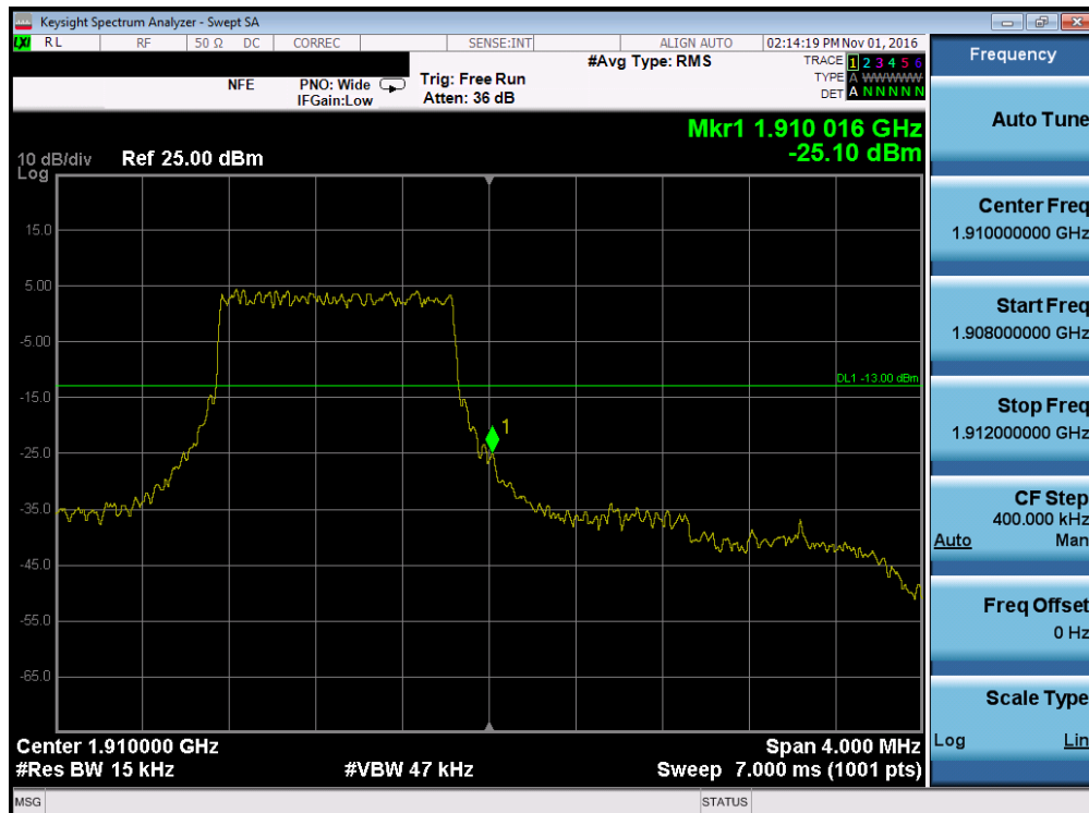
Plot 7-130. Upper Band Edge Plot (Band 2 – 1.4MHz QPSK – RB Size 6)
