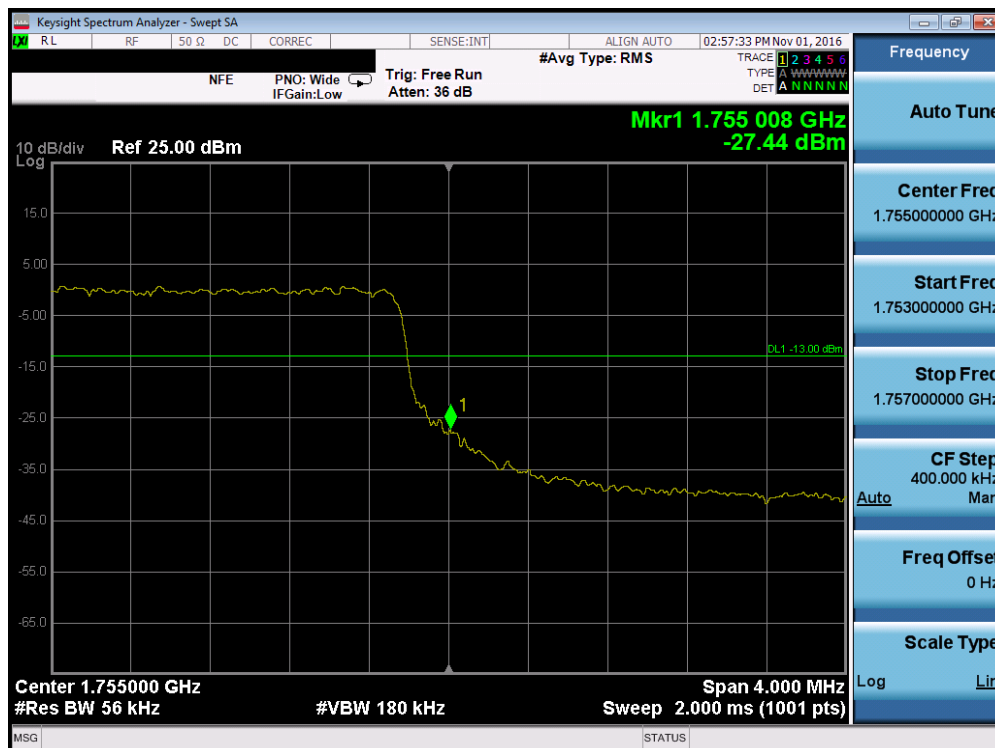
Plot 7-114. Upper Band Edge Plot (Band 4 – 5.0MHz QPSK – RB Size 25)
