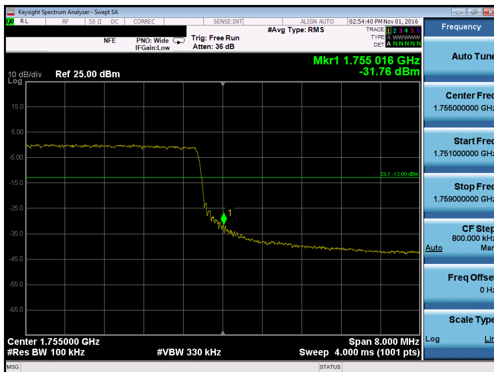
Plot 7-118. Upper Band Edge Plot (Band 4 – 10.0MHz QPSK – RB Size 50)
