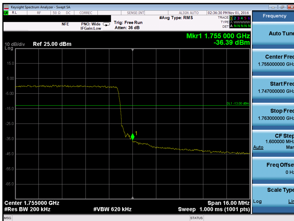
Plot 7-126. Upper Band Edge Plot (Band 4 – 20.0MHz QPSK – RB Size 100)
