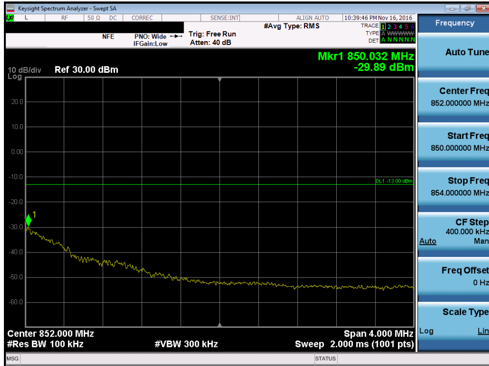
Plot 7-97. Upper Extended Band Edge Plot (Band 5 – 1.4MHz QPSK – RB Size 6)
