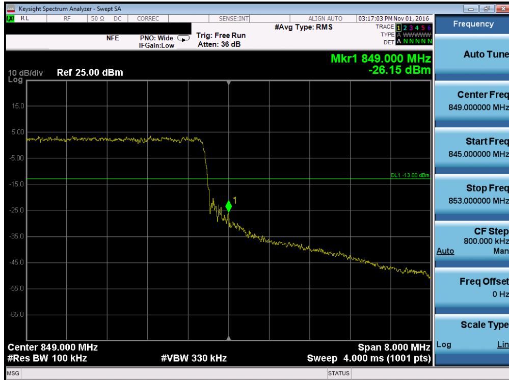
Plot 7-103. Upper Band Edge Plot (Band 5 - 10.0MHz QPSK - RB Size 50)
