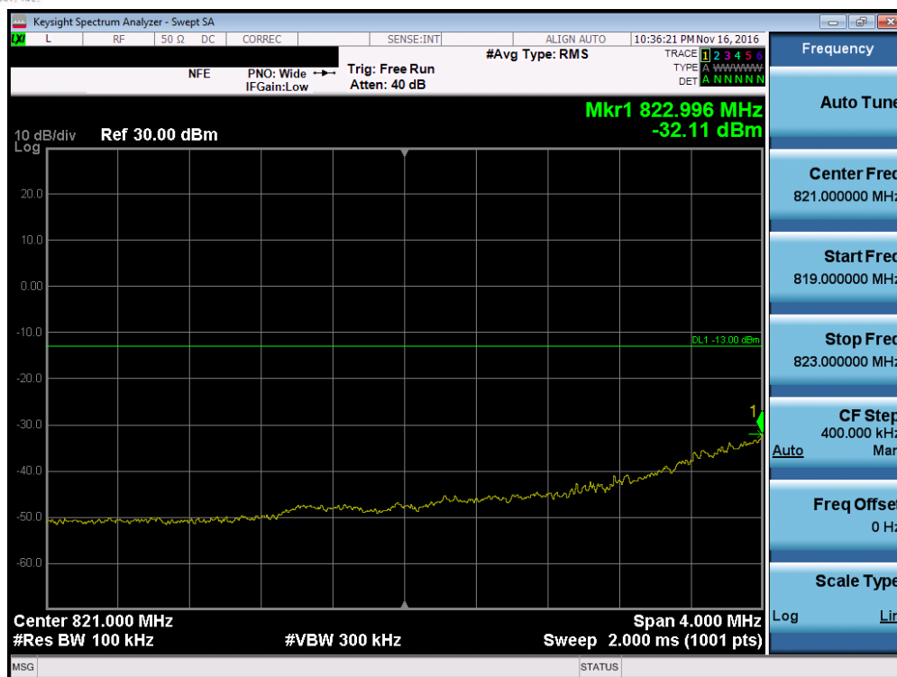
Plot 7-95. Lower Extended Band Edge Plot (Band 5 - 1.4MHz QPSK - RB Size 6)
