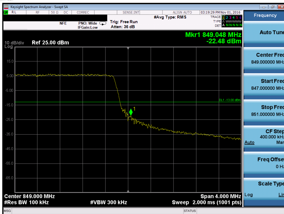
Plot 7-101. Upper Band Edge Plot (Band 5 - 5.0MHz QPSK - RB Size 25)
