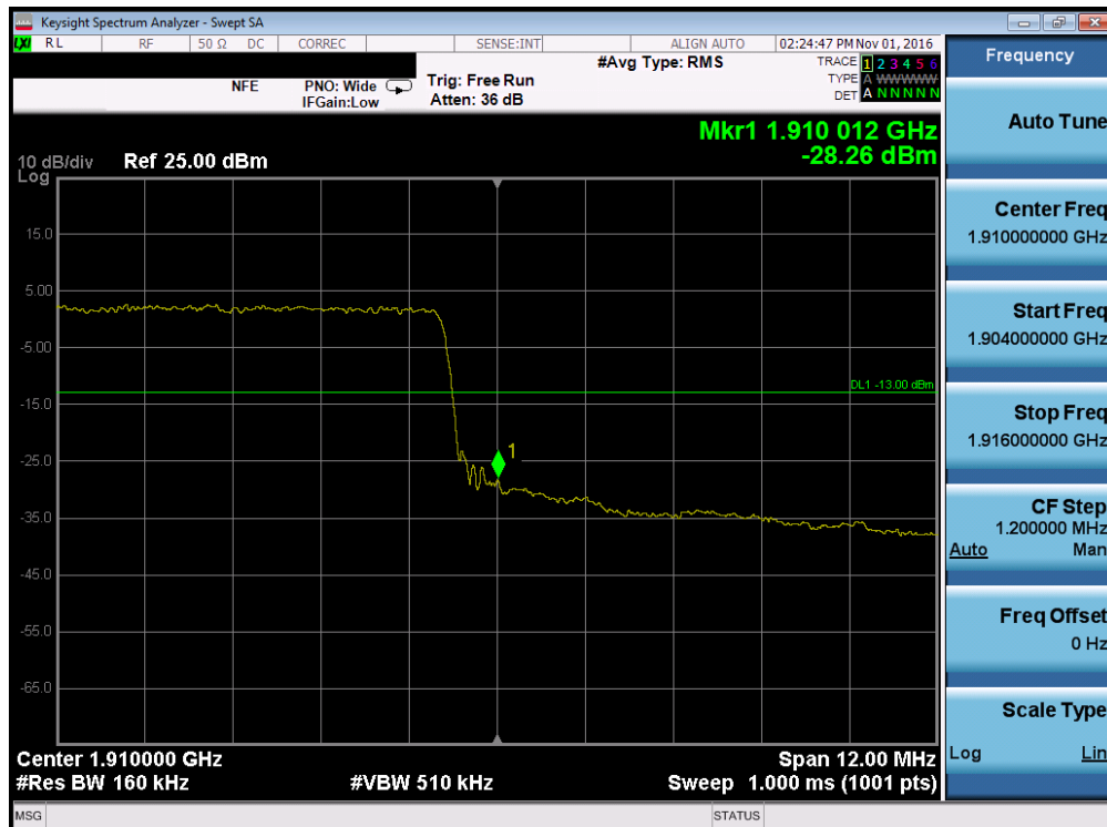
Plot 7-146. Upper Band Edge Plot (Band 2 – 15.0MHz QPSK – RB Size 75)
