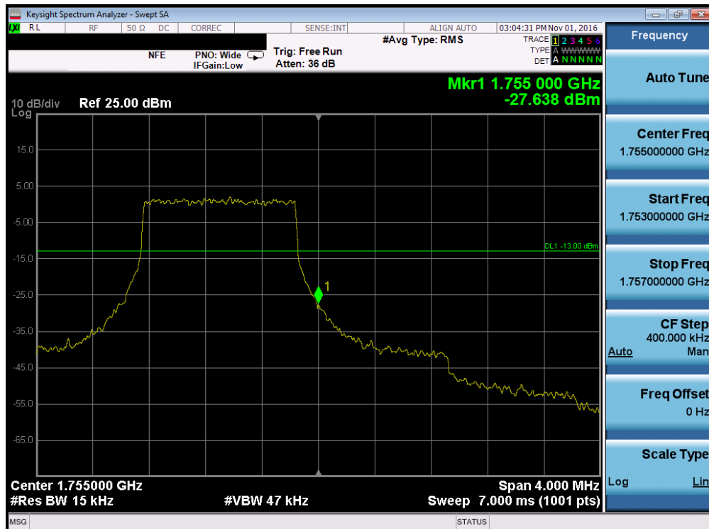
Plot 7-106. Upper Band Edge Plot (Band 4 – 1.4MHz QPSK – RB Size 6)
