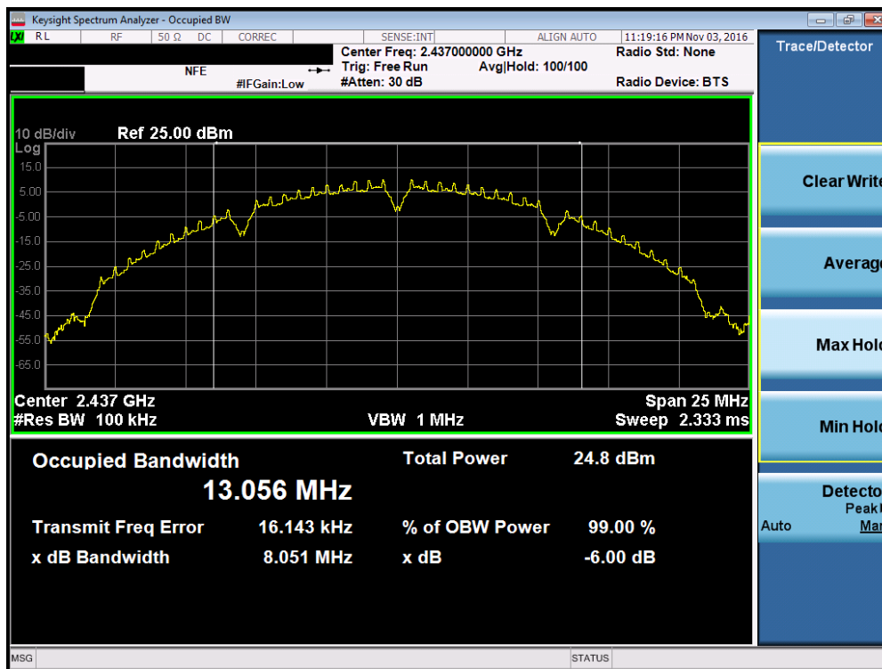
Plot 7-2. 6dB Bandwidth Plot (802.11b – Ch. 6)
