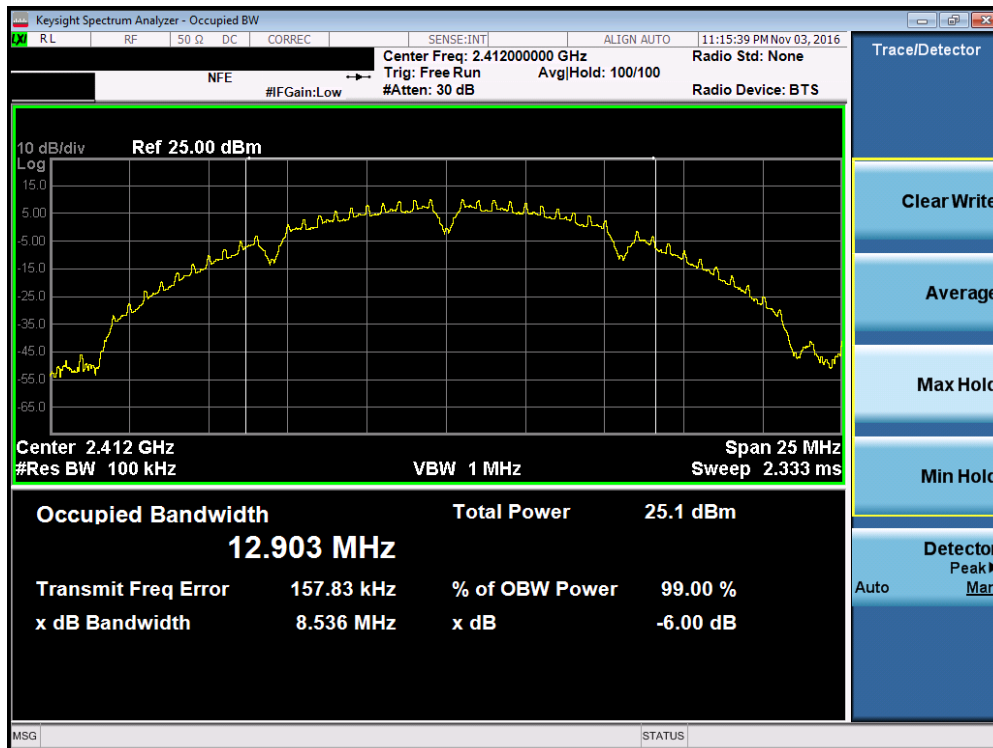
Plot 7-1. 6dB Bandwidth Plot (802.11b – Ch. 1)
