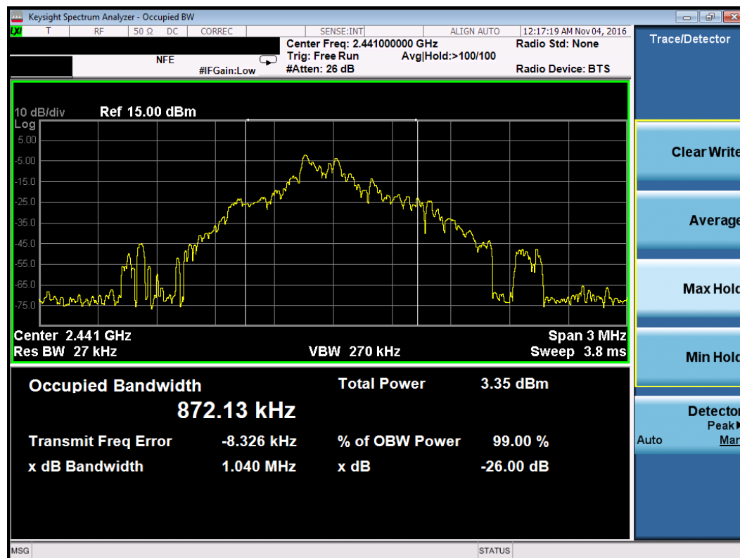
Plot 7-1. Occupied Bandwidth Plot (ANT+ – Ch. 39)
