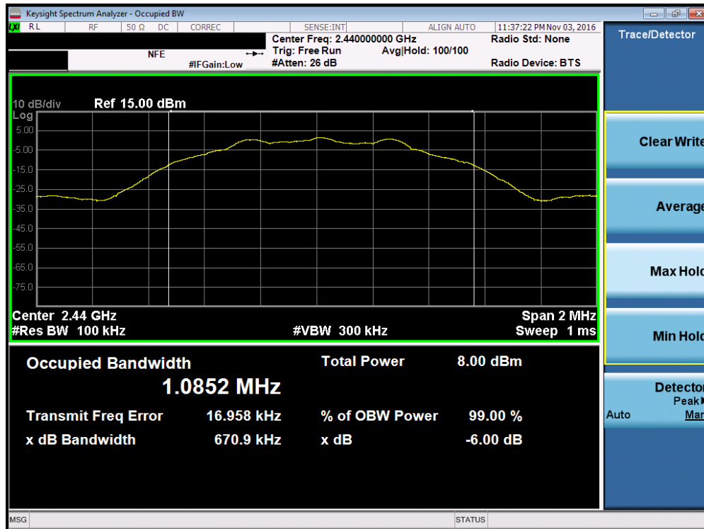
Plot 7-2. 6dB Bandwidth Plot (Bluetooth (LE) – Ch. 19)
