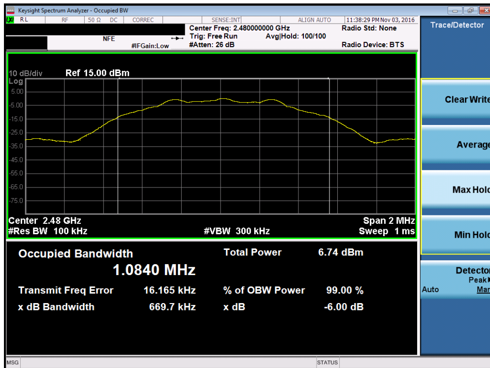
Plot 7-3. 6dB Bandwidth Plot (Bluetooth (LE) – Ch. 39)
