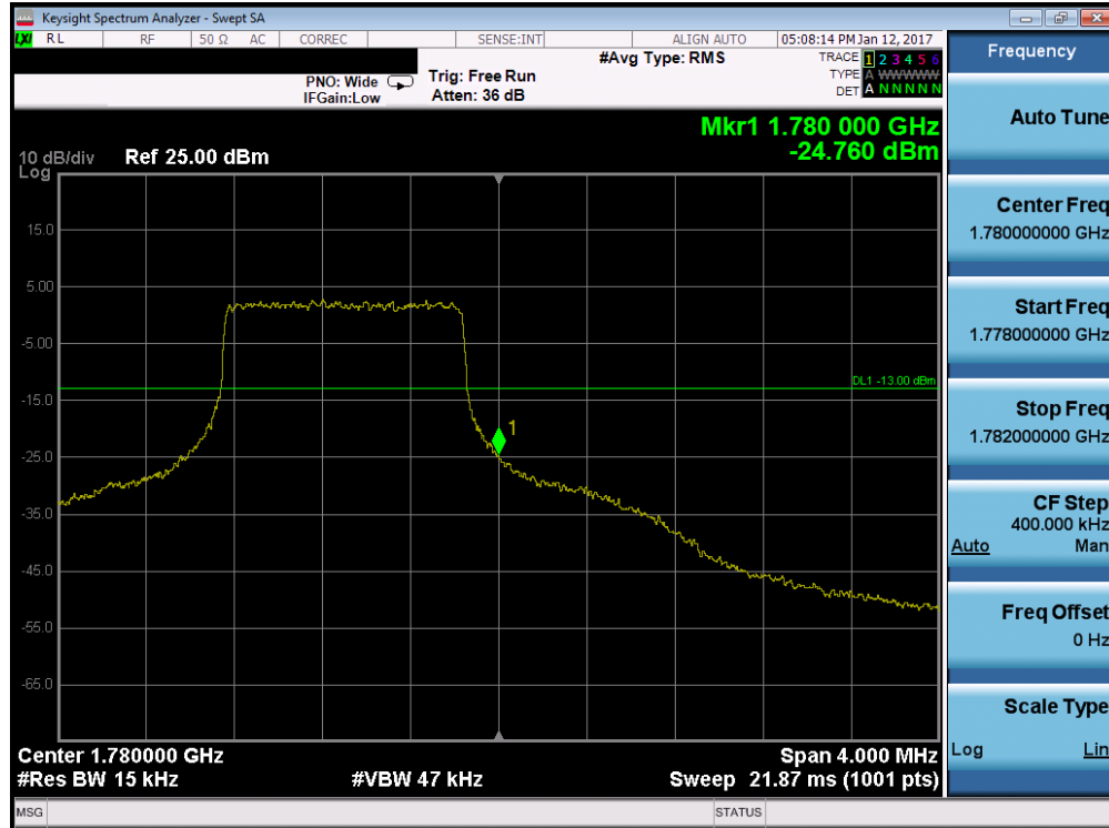
Plot 7-124. Upper Band Edge Plot (Band 66/4 – 1.4MHz QPSK – RB Size 6)
