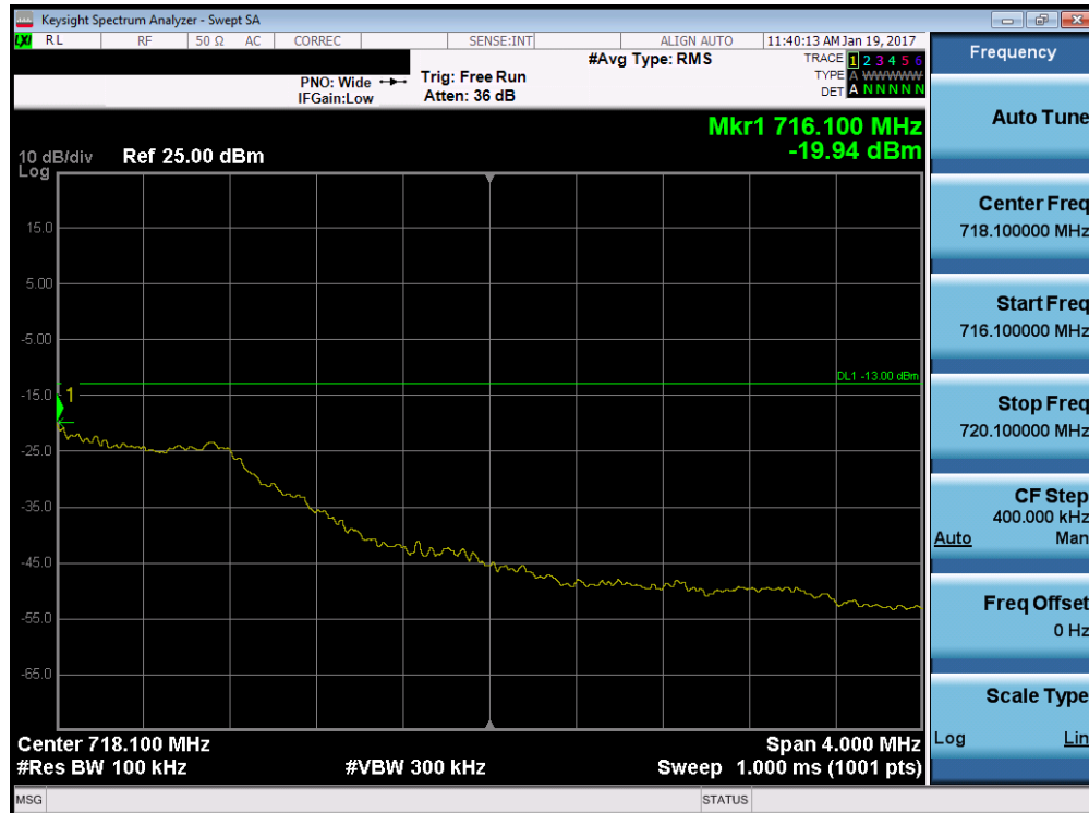
Plot 7-87. Upper Extended Band Edge Plot (Band 12 – 1.4MHz QPSK – RB Size 6)
