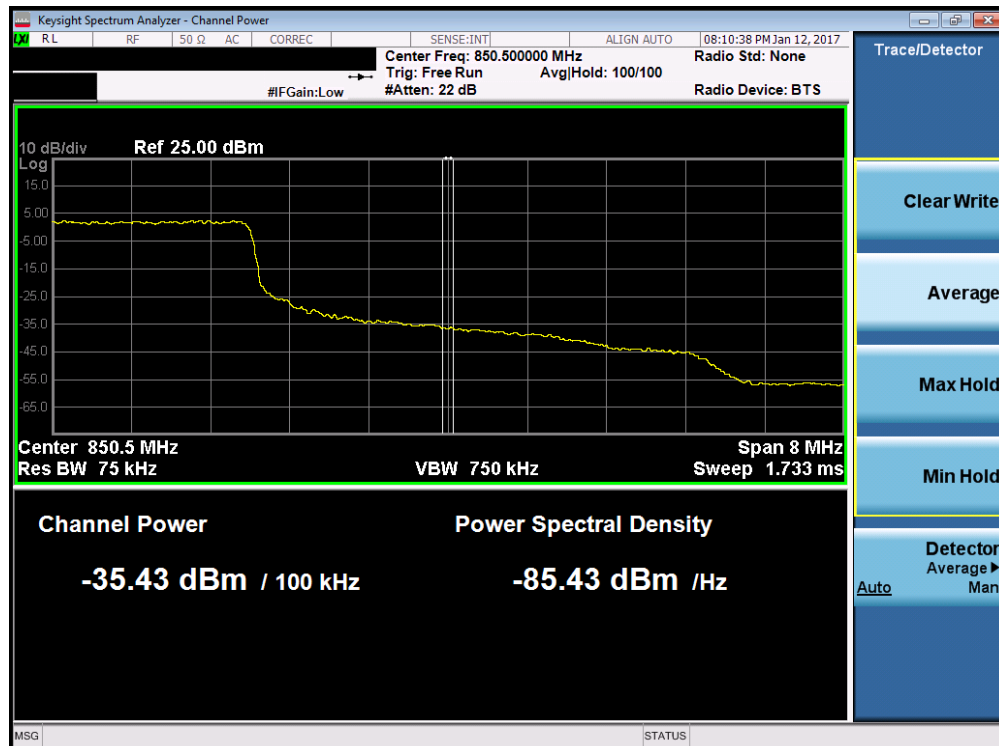
Plot 7-121. Upper Extended Band Edge Plot (Band 5 – 10.0MHz QPSK – RB Size 50)
