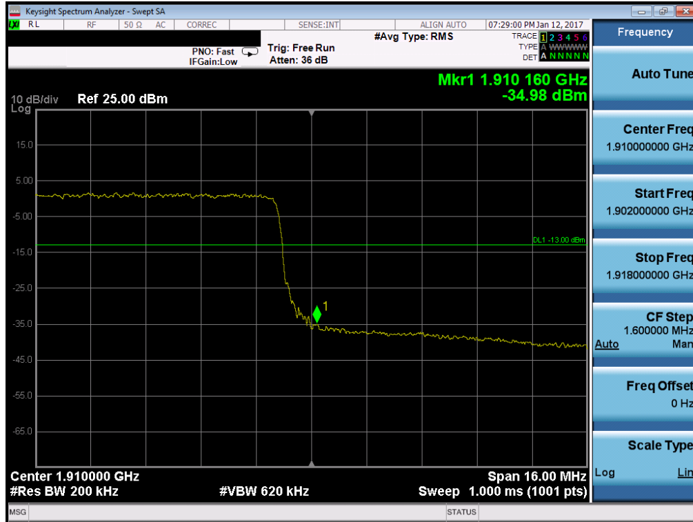
Plot 7-168. Upper Band Edge Plot (Band 2 – 20MHz QPSK – RB Size 100)
