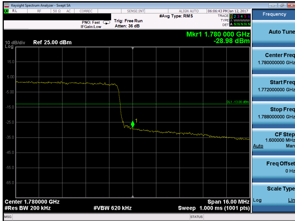
Plot 7-144. Upper Band Edge Plot (Band 66/4 – 20.0MHz QPSK – RB Size 100)
