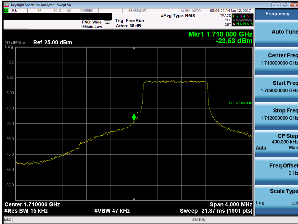
Plot 7-122. Lower Band Edge Plot (Band 66/4 – 1.4MHz QPSK – RB Size 6)
