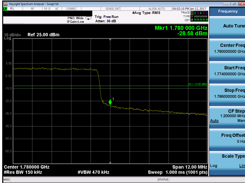
Plot 7-140. Upper Band Edge Plot (Band 66/4 – 15.0MHz QPSK – RB Size 75)
