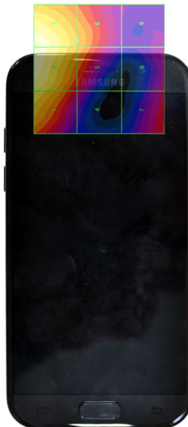
Figure 17-4 E-Field WD Scan overlay
