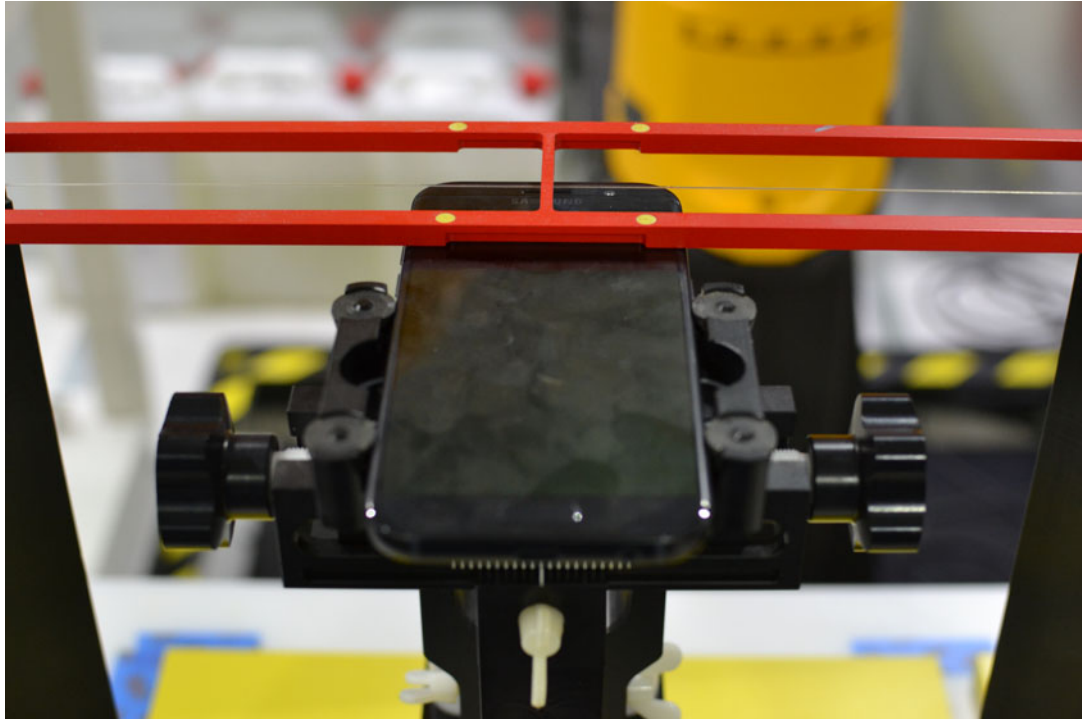
Figure 17-1 Ear Reference Point HAC Phantom Alignment
