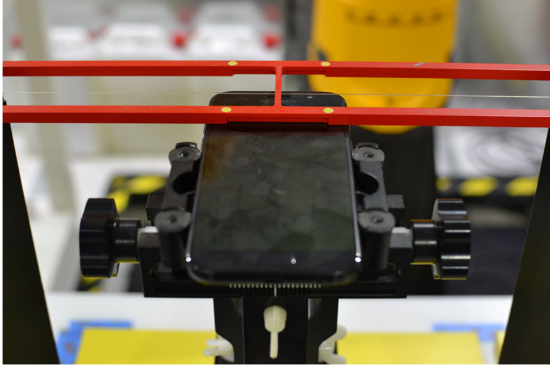
Figure 17-1 Ear Reference Point HAC Phantom Alignment
