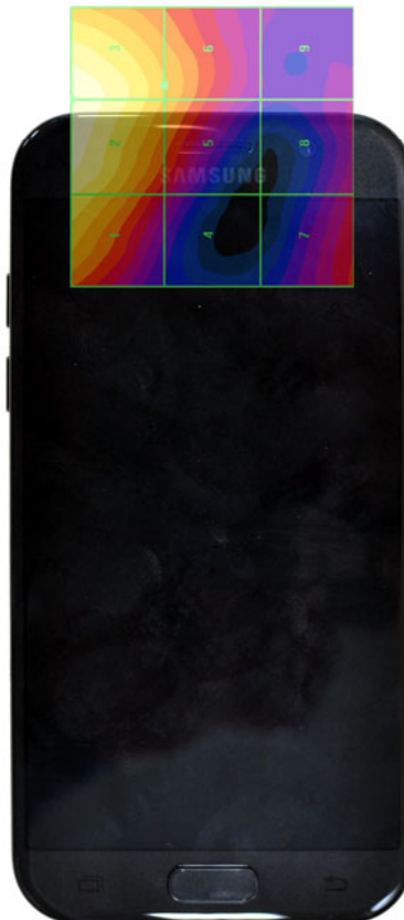
Figure 17-4 E-Field WD Scan overlay
