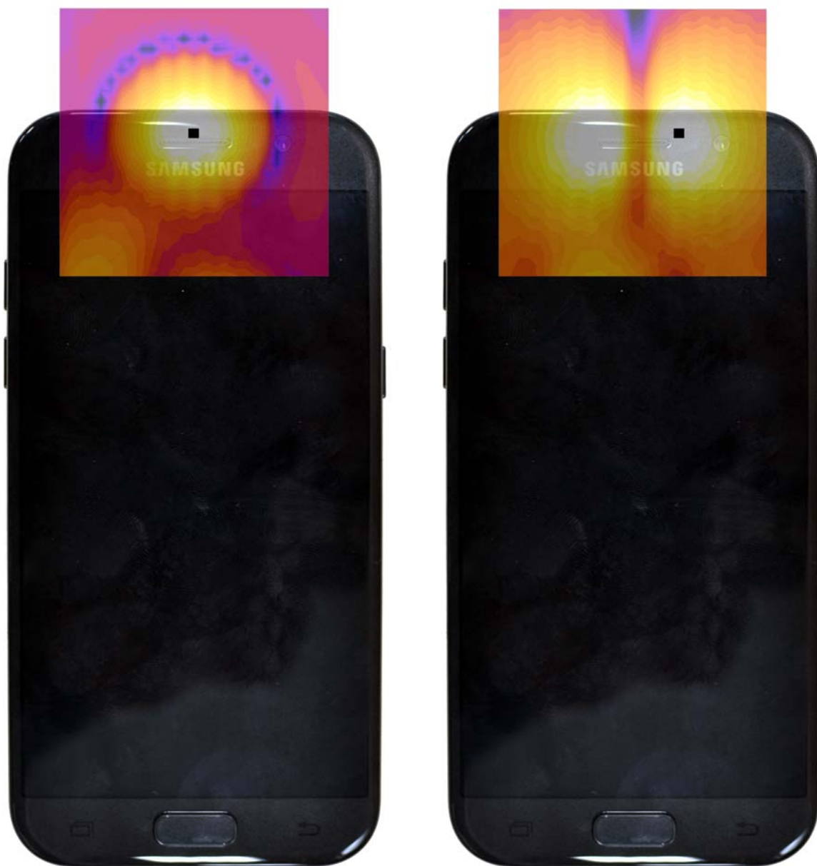
Figure 14-3 T-Coil Scan Overlay Magnetic Field Distributions
