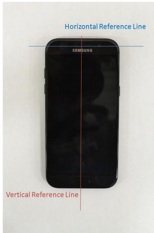
SAR Test Setup Photo 6 Vertical and Horizontal Reference
