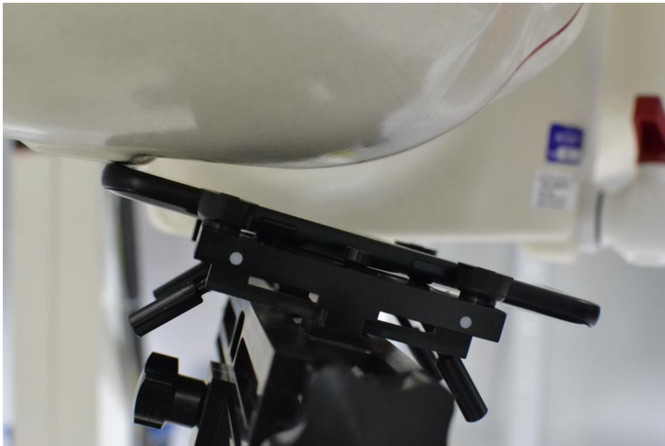
SAR Test Setup Photo 2 Right Tilt
