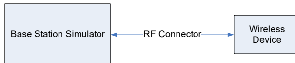
Figure 9-1 Power Measurement Setup
