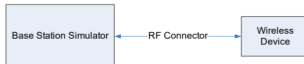
Figure 9-2 Power Measurement Setup
