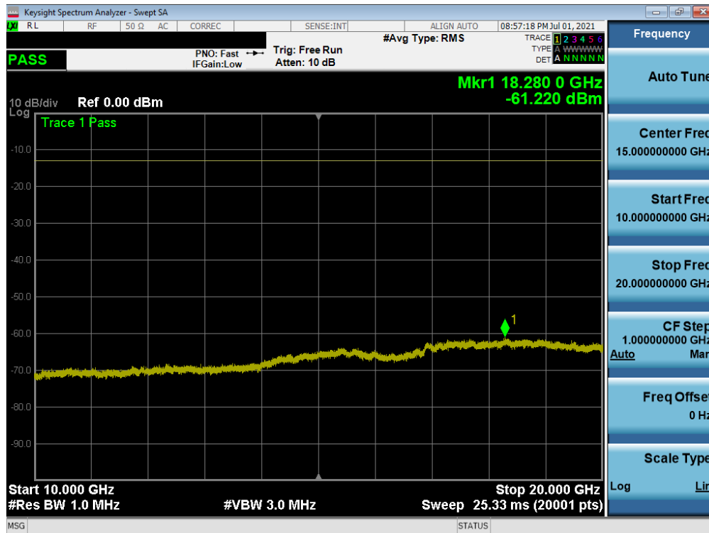
Plot 7-21. Conducted Spurious Plot (LTE Band 2 - 20MHz QPSK - 1RB - Mid Channel)
