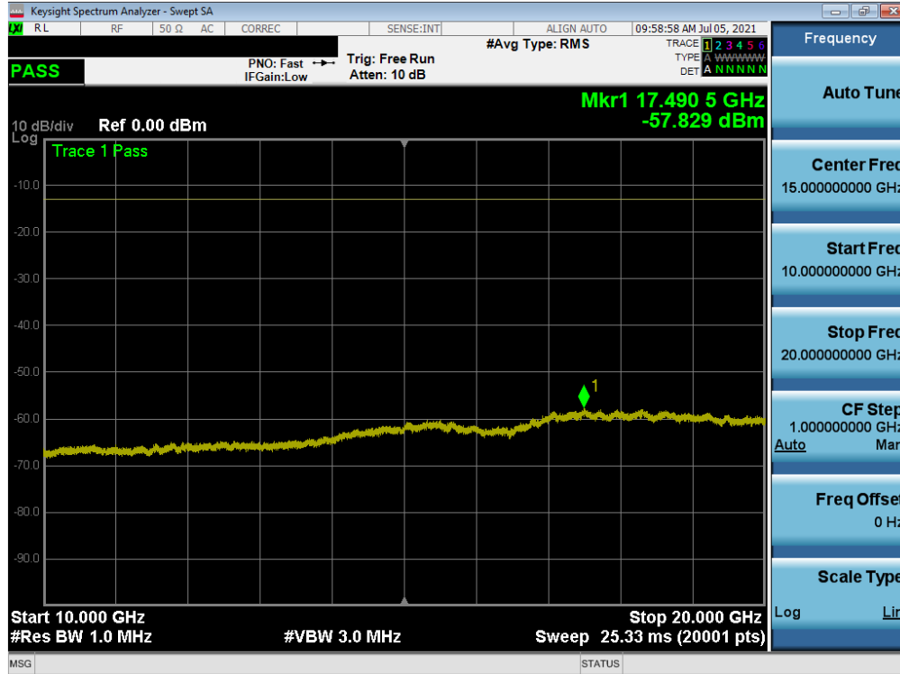
Plot 7-36. Conducted Spurious Plot (WCDMA Ch. 9262)
