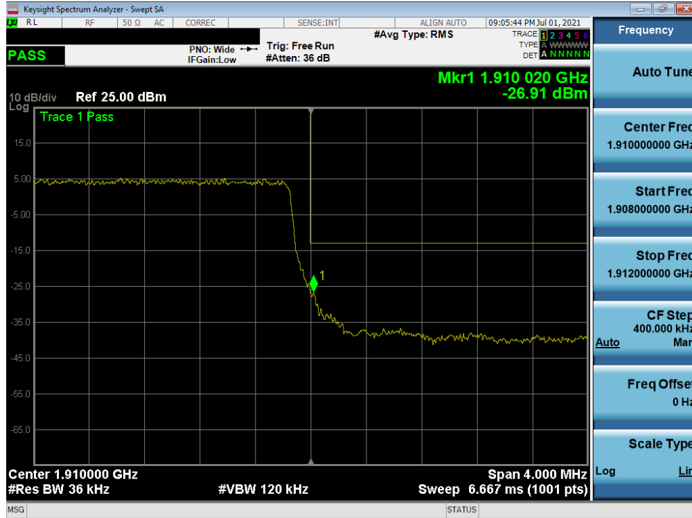
Plot 7-61. Upper Band Edge Plot (LTE Band 2 - 3MHz QPSK – Full RB)
