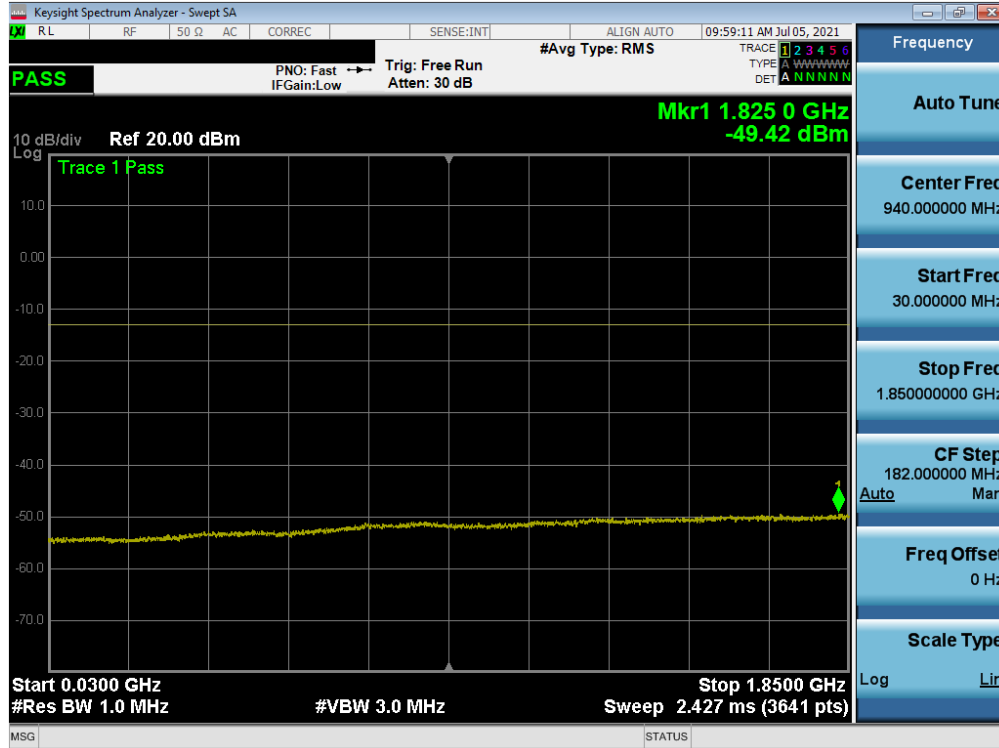
Plot 7-40. Conducted Spurious Plot (WCDMA Ch. 9538)
