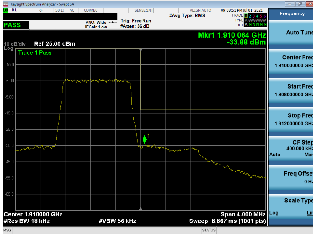
Plot 7-65. Upper Band Edge Plot (LTE Band 2 – 1.4MHz QPSK – Full RB)
