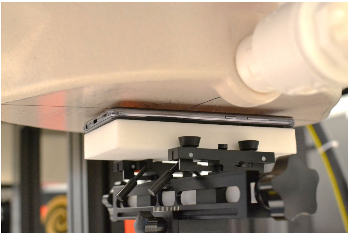
SAR Test Setup Photo 10 – Phablet, Front Side at 5mm
