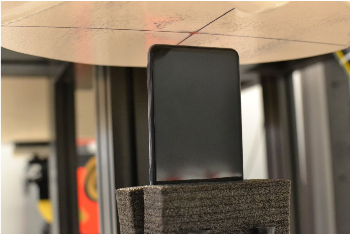
SAR Test Setup Photo 12 – Hotspot, Bottom Edge at 10mm
