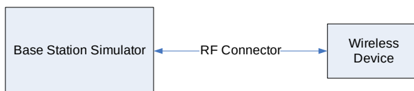
Figure 9-1 Power Measurement Setup
