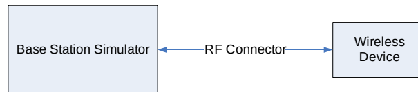
Figure 9-2 Power Measurement Setup
