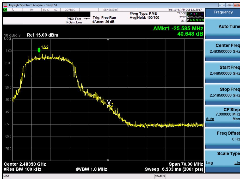
Plot 7-24. Band Edge Plot (802.11n (2.4GHz) – Ch. 11)
