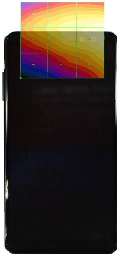
Figure 18-4 E-Field WD Scan overlay
