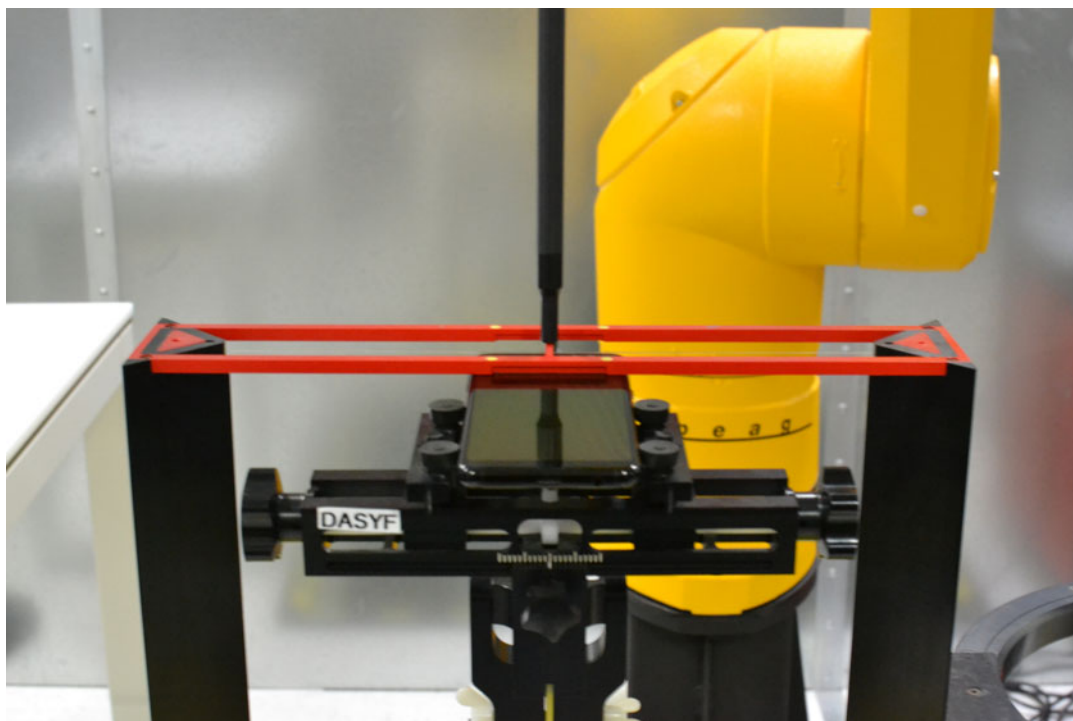
Figure 18-1 Ear Reference Point HAC Phantom Alignment
