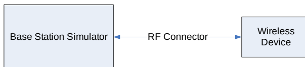
Figure 9-2 Power Measurement Setup
