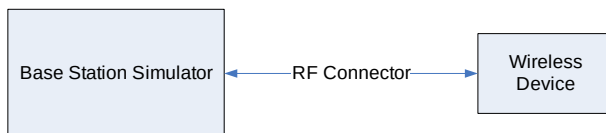
Figure 9-2 Power Measurement Setup
