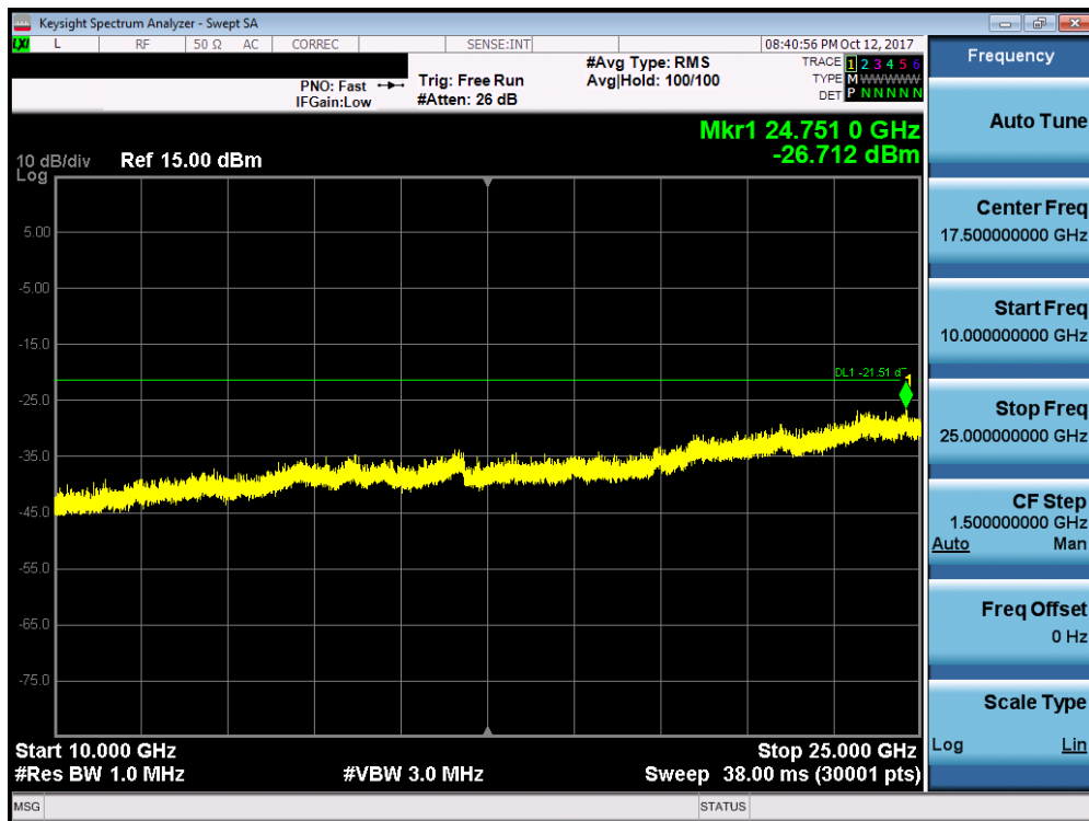
Plot 7-28. Conducted Spurious Plot (802.11b – Ch. 6)
