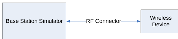
Figure 9-2 Power Measurement Setup
