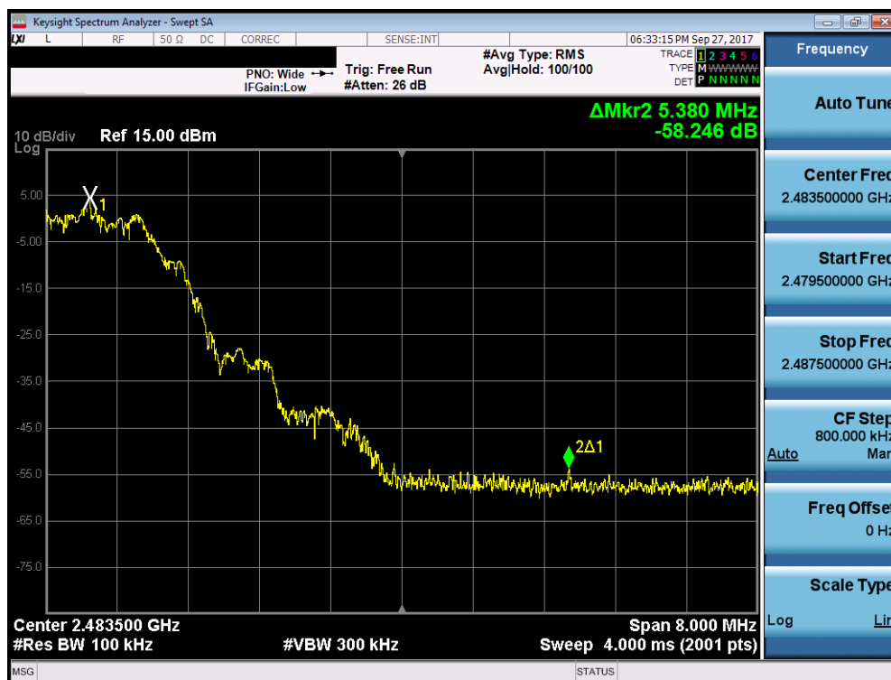
Plot 7-22. Band Edge Plot (Bluetooth (LE), 2Mbps - Ch. 39)
