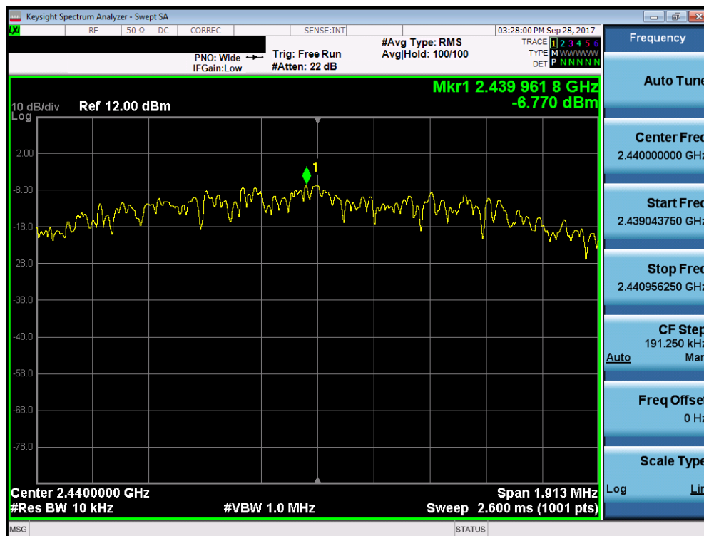
Plot 7-17. Power Spectral Density Plot (Bluetooth (LE), 2Mbps – Ch. 19)
