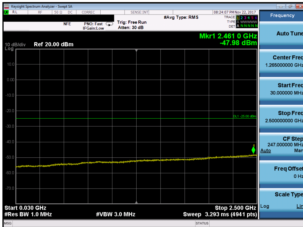
Plot 7-124. Conducted Spurious Plot (Band 7 - 10.0MHz QPSK - RB Size 1, RB Offset 0 - Mid Channel)
