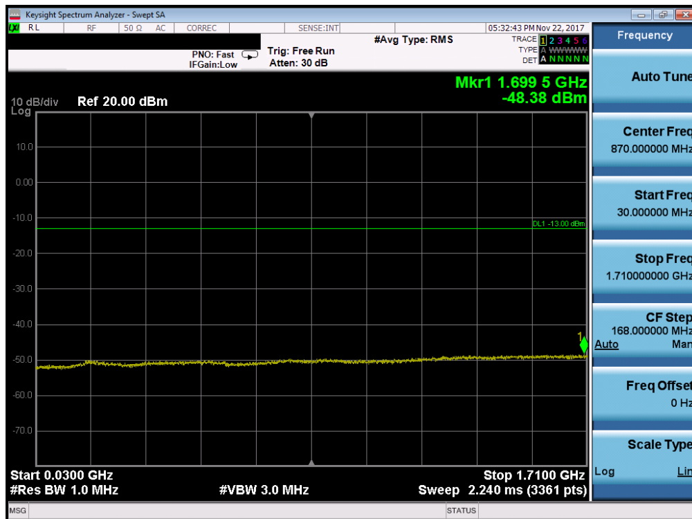
Plot 7-106. Conducted Spurious Plot (Band 66/4 - 15.0MHz QPSK - RB Size 1, RB Offset 0 - Mid Channel)
