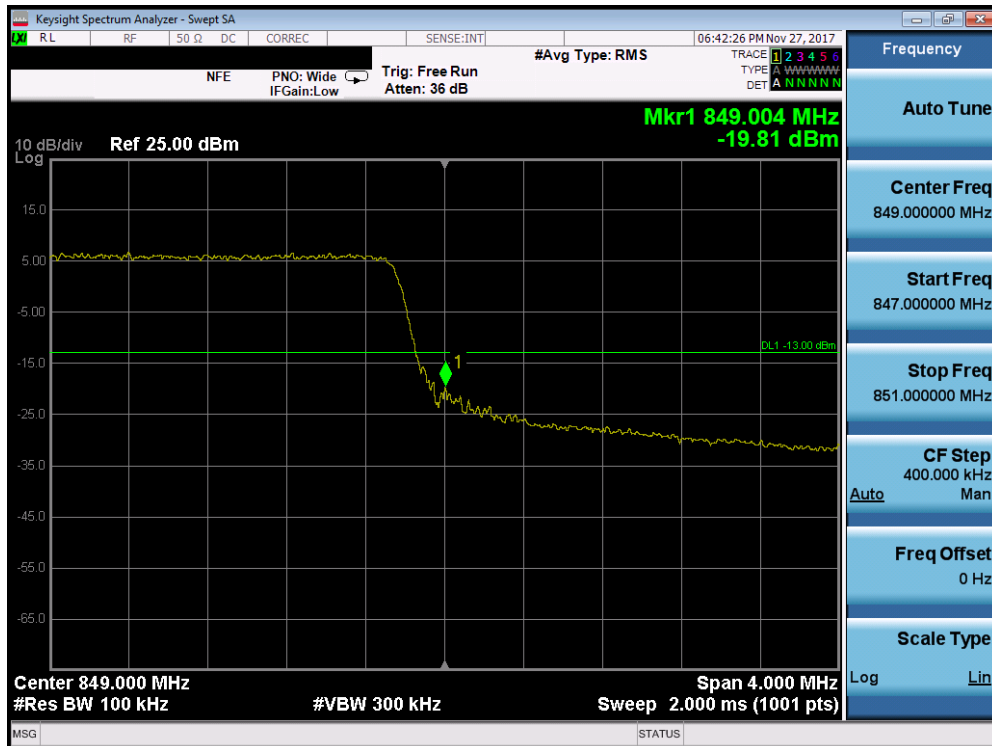
Plot 7-153. Upper Band Edge Plot (Band 26/5 - 5.0MHz QPSK - Full RB Configuration)
