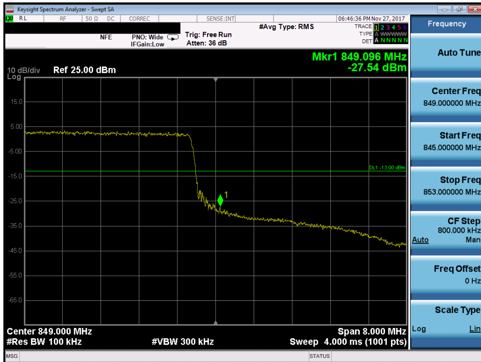
Plot 7-155. Upper Band Edge Plot (Band 26/5 - 10.0MHz QPSK - Full RB Configuration)
