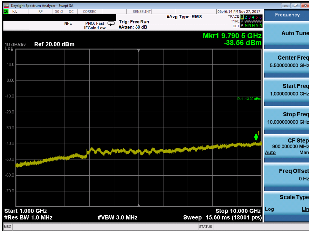
Plot 7-102. Conducted Spurious Plot (Band 26/5 - 10.0MHz QPSK - RB Size 1, RB Offset 0 - High Channel)
