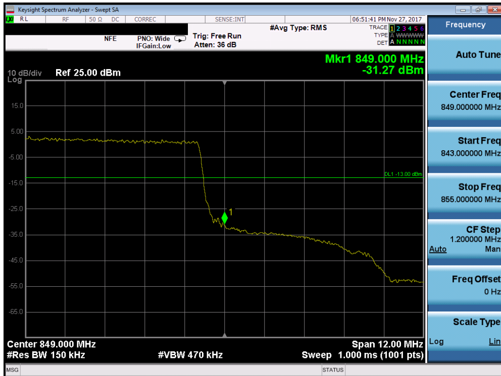
Plot 7-157. Upper Band Edge Plot (Band 26 - 15.0MHz QPSK - Full RB Configuration)
