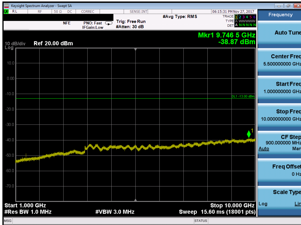
Plot 7-84. Conducted Spurious Plot (Band 12/17 - 5.0MHz QPSK - RB Size 1, RB Offset 0 - Low Channel)
