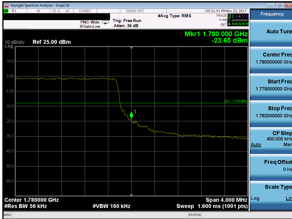
Plot 7-174. Upper Band Edge Plot (Band 66 - 5.0MHz QPSK - Full RB Configuration)
