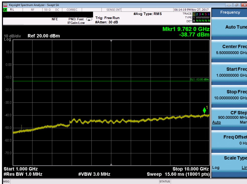
Plot 7-87. Conducted Spurious Plot (Band 12/17 - 5.0MHz QPSK - RB Size 1, RB Offset 0 - Mid Channel)
