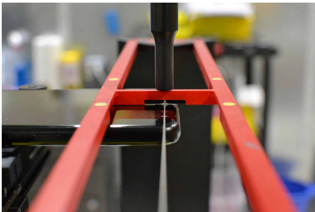
Figure 17-2 HAC Phantom Plane Alignment
