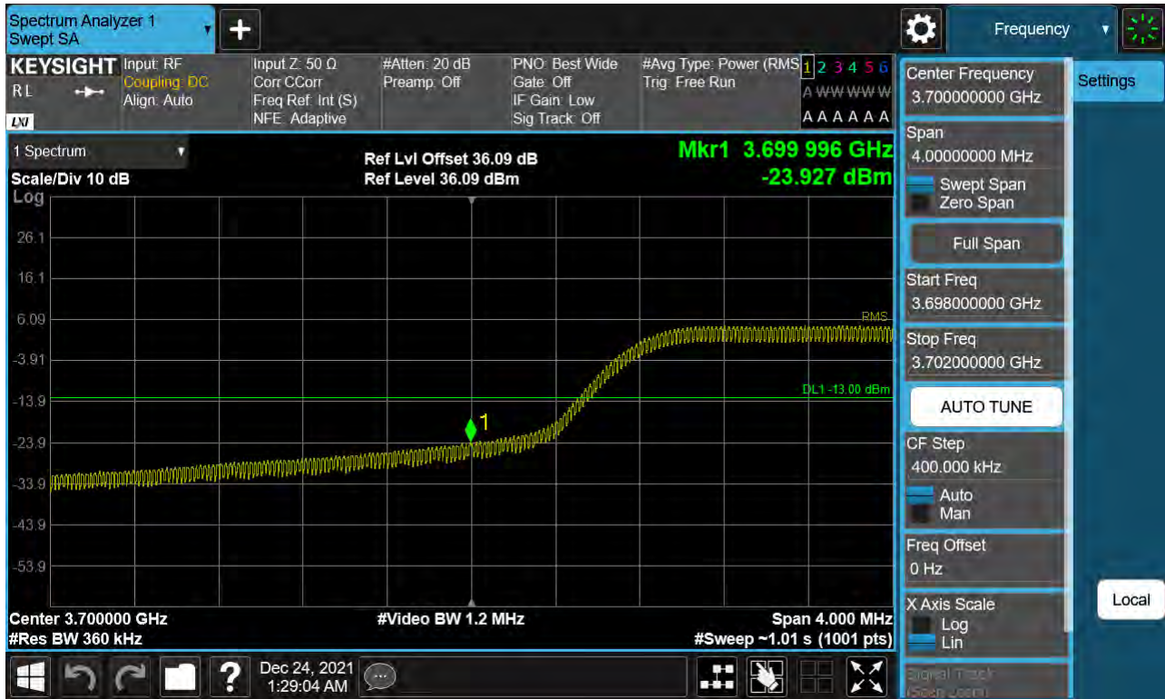
Sub6 n77. Low Band Edge Plot (60 M BW Ch.648668 BPSK FullIRB)(1)
