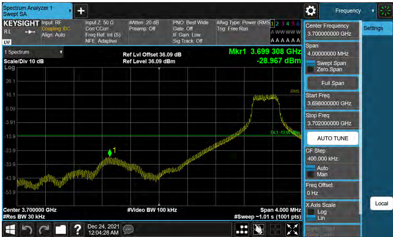
Sub6 n77. Low Band Edge Plot (70 M BW Ch.649000 BPSK 1RB)(1)
