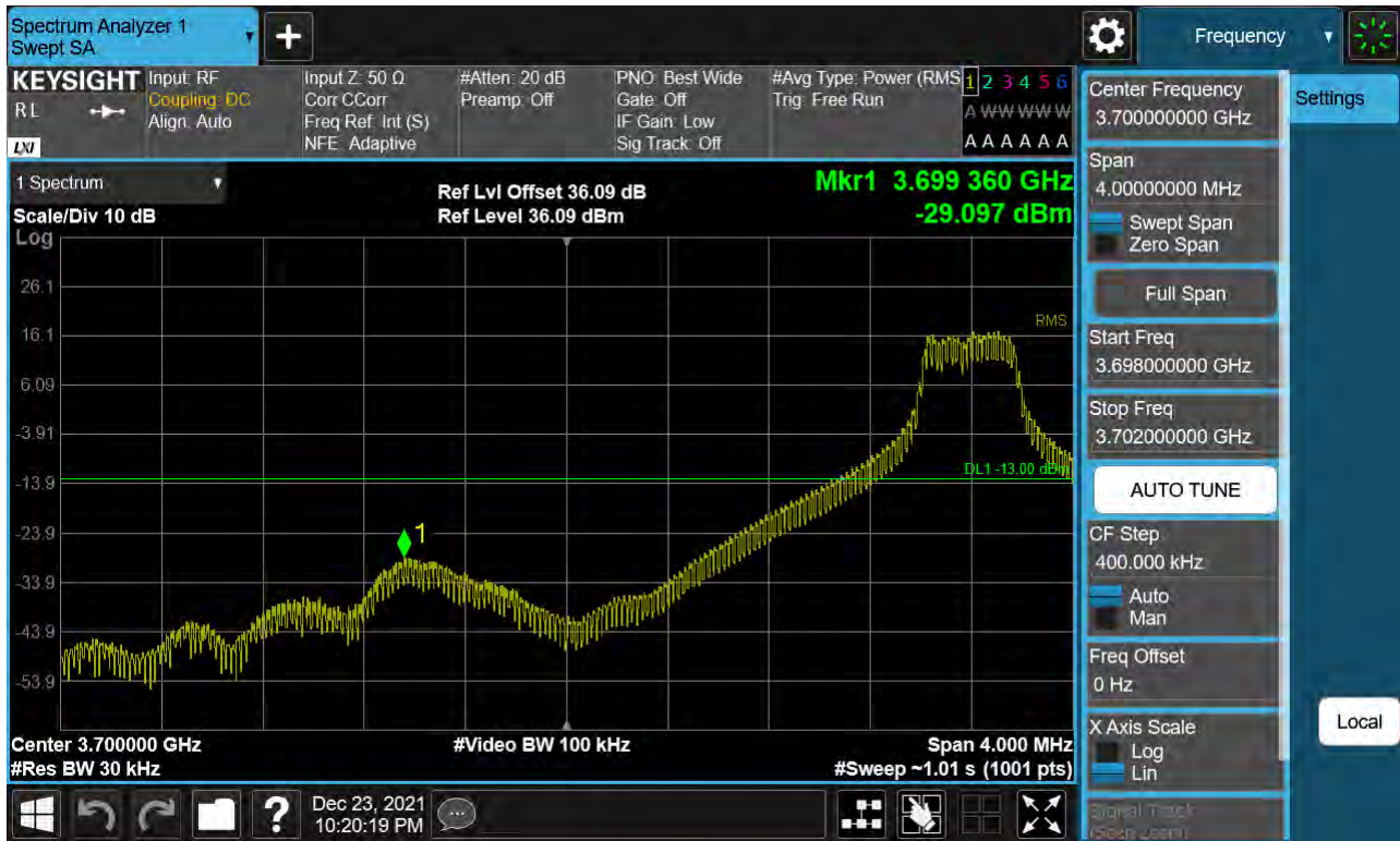
Sub6 n77. Low Band Edge Plot (50 M BW Ch.648334 BPSK 1RB)(1)
