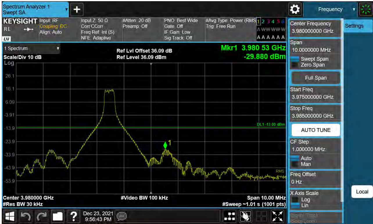
Sub6 n77. High Band Edge Plot (30 M BW Ch.664332 BPSK 1RB)(1)
