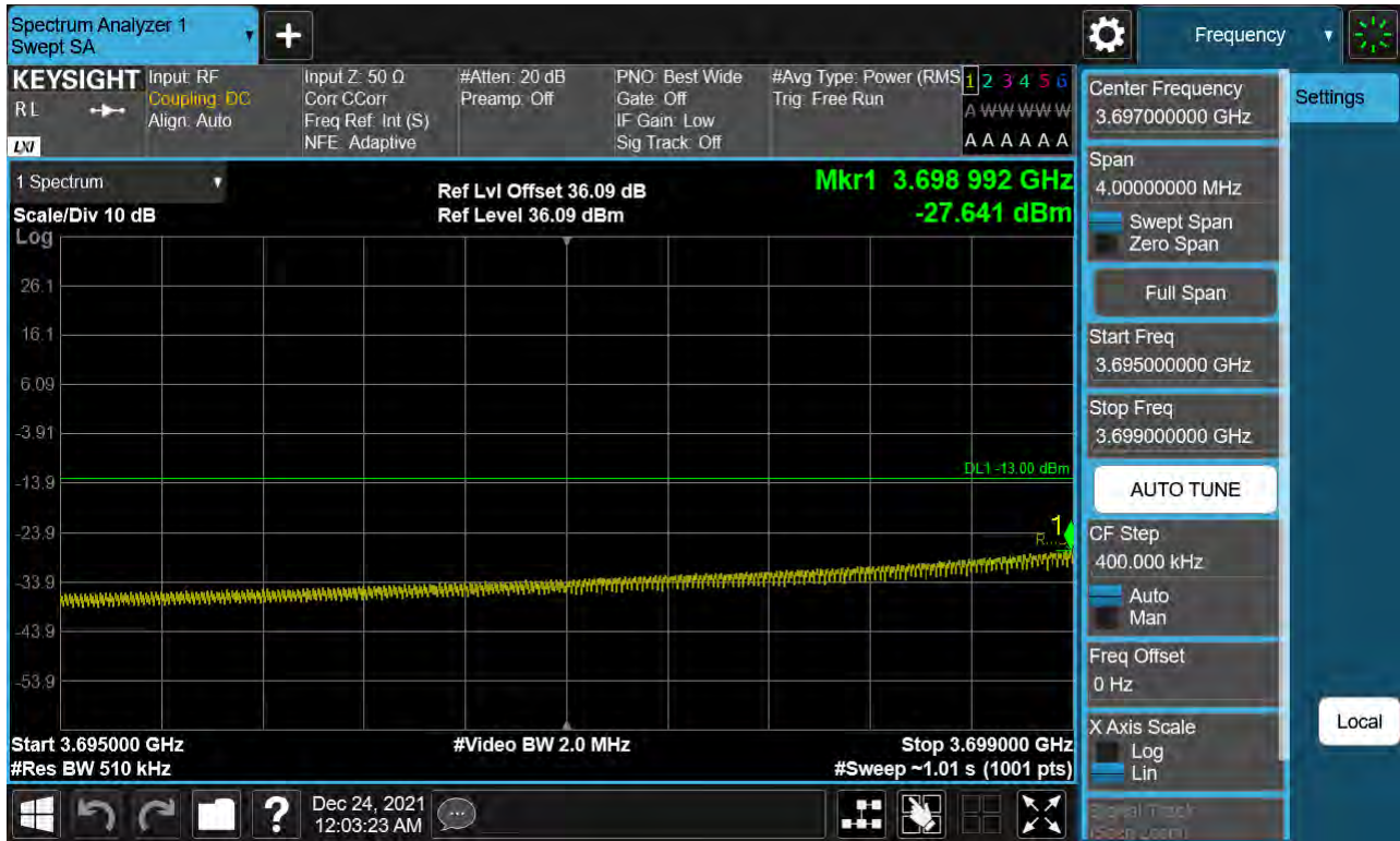
Sub6 n77. Low Band Edge Plot (70 M BW Ch.649000 BPSK FullRB)(2)
