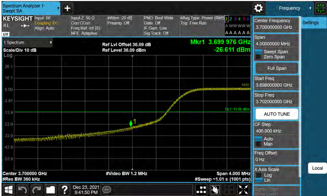
Sub6 n77. Low Band Edge Plot (30 M BW Ch.647668 BPSK FullIRB)(1)
