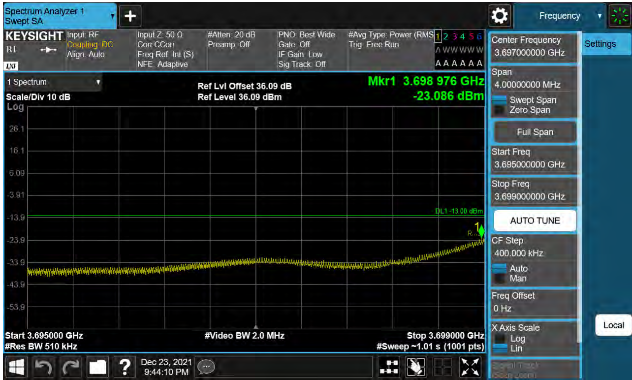
Sub6 n77. Low Band Edge Plot (30 M BW Ch.647668 BPSK 1RB)(2)
