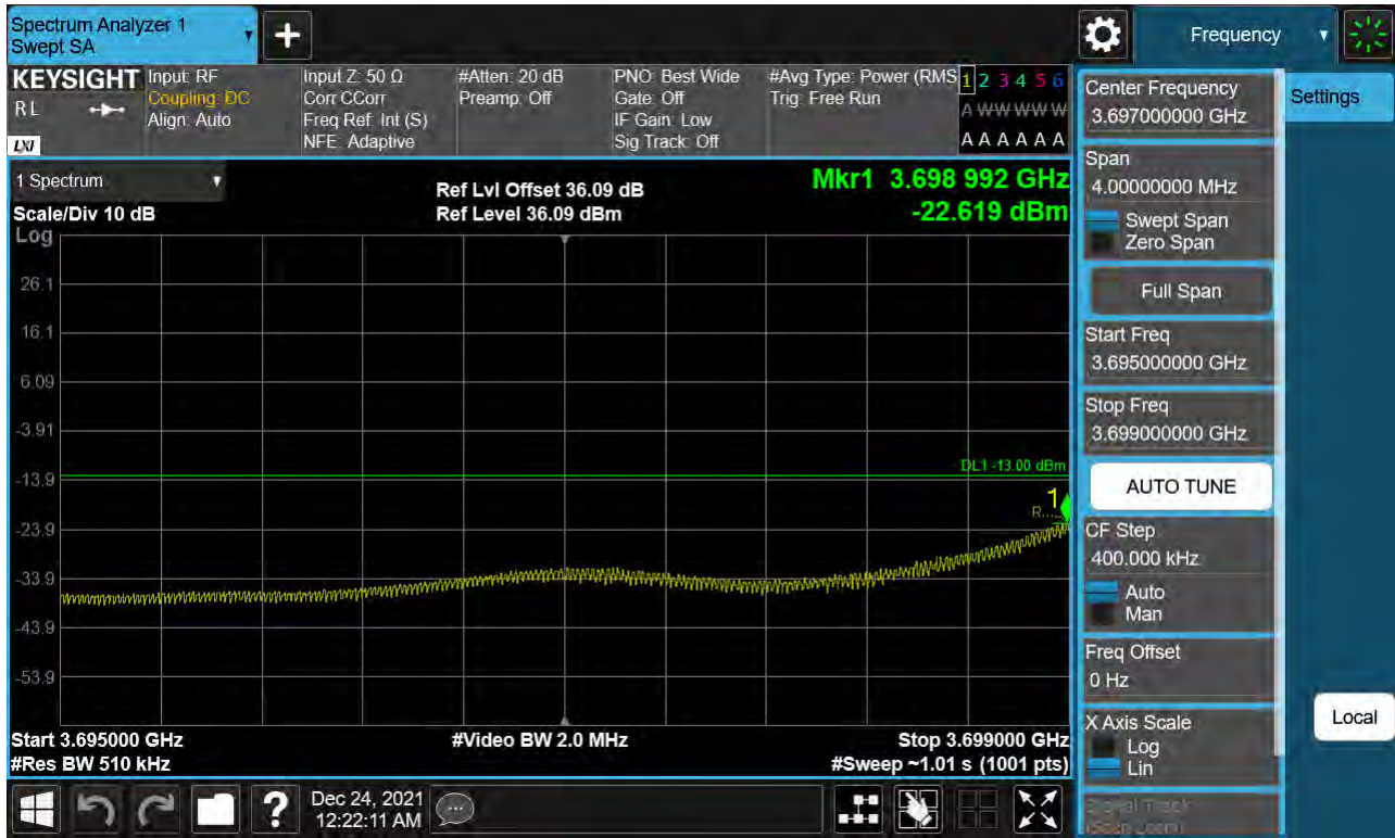
Sub6 n77. Low Band Edge Plot (80 M BW Ch.649334 BPSK 1RB)(2)
