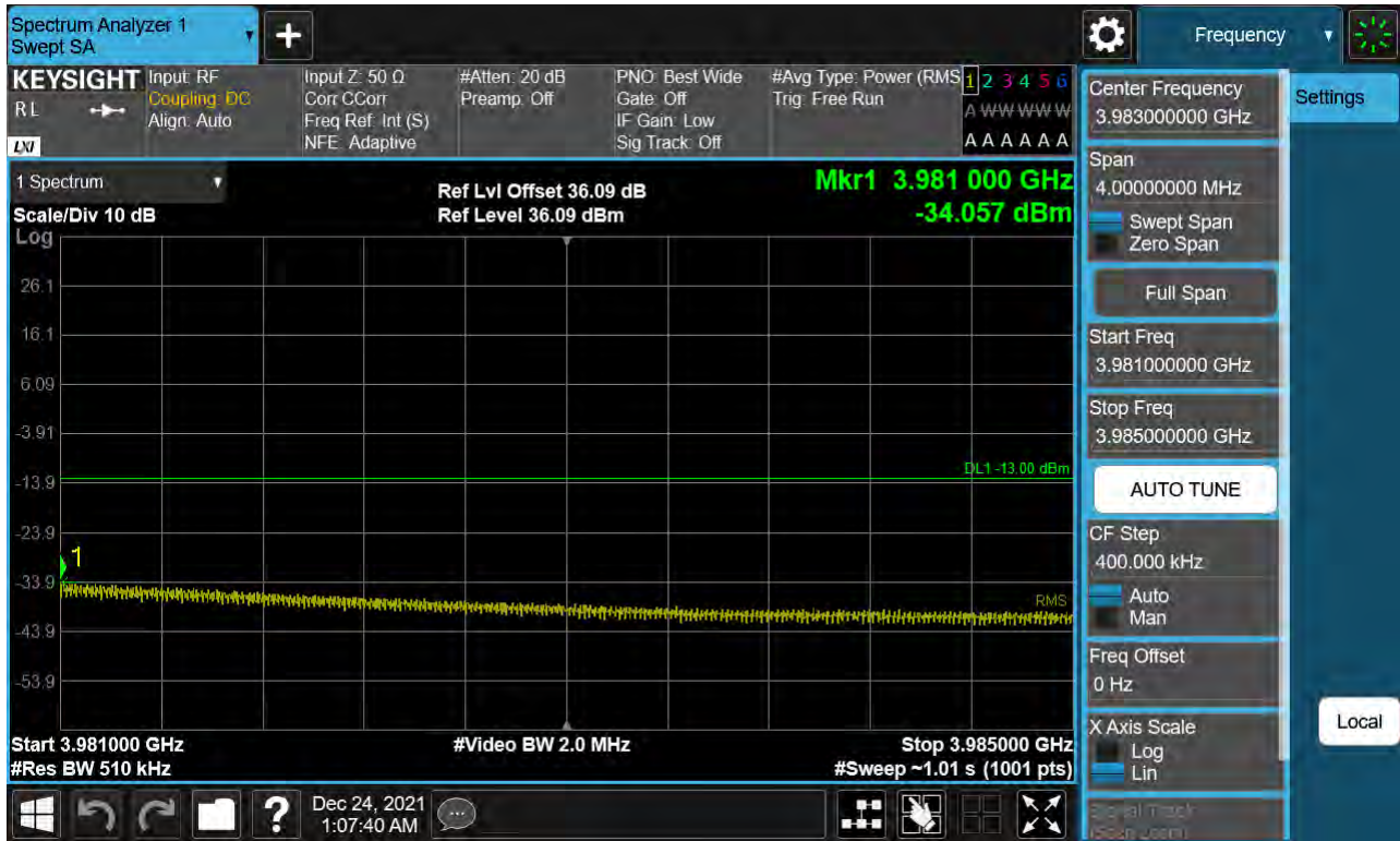
Sub6 n77. High Band Edge Plot (100 M BW Ch.662000 BPSK FullRB)(2)
