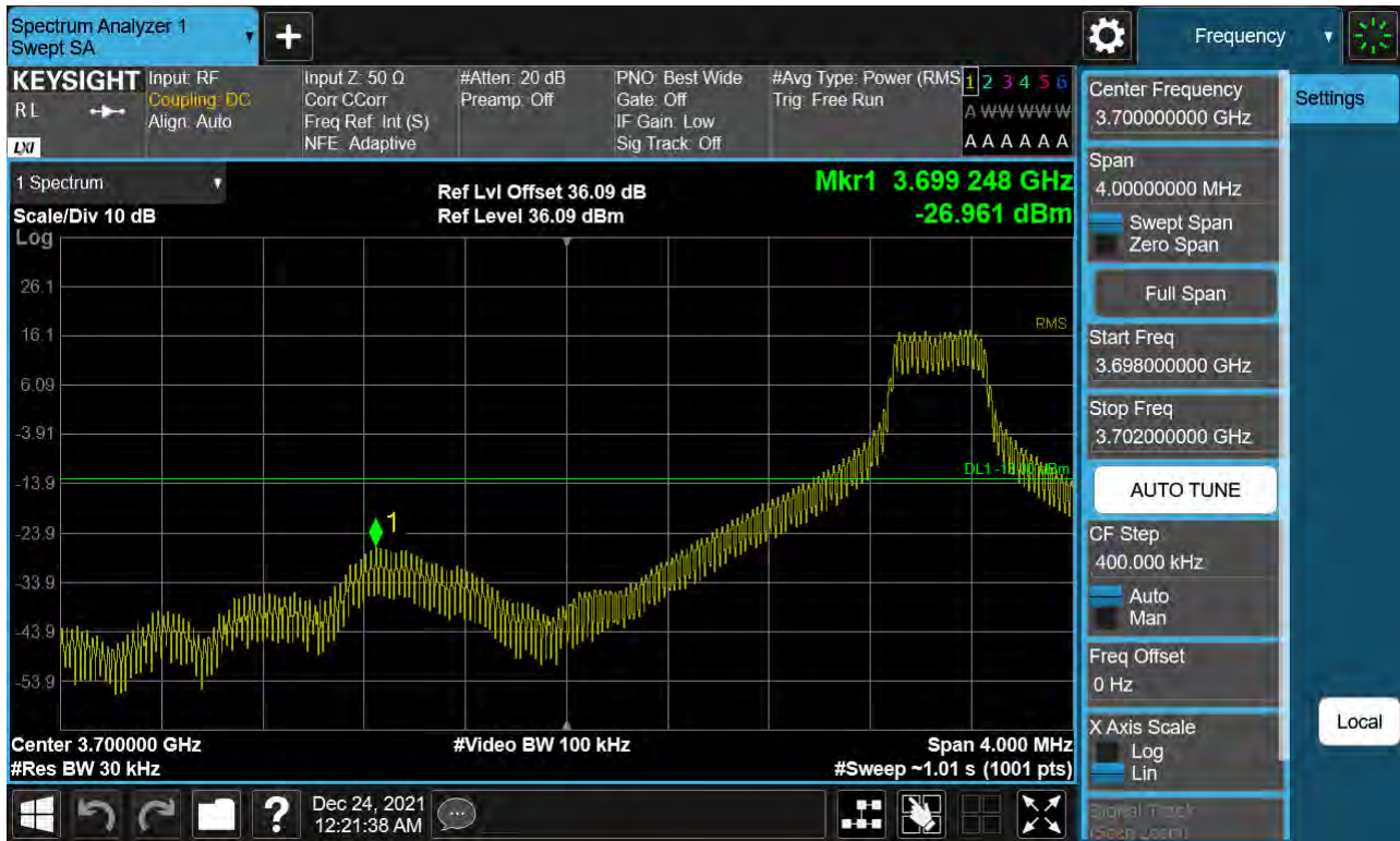
Sub6 n77. Low Band Edge Plot (80 M BW Ch.649334 BPSK 1RB)(1)
