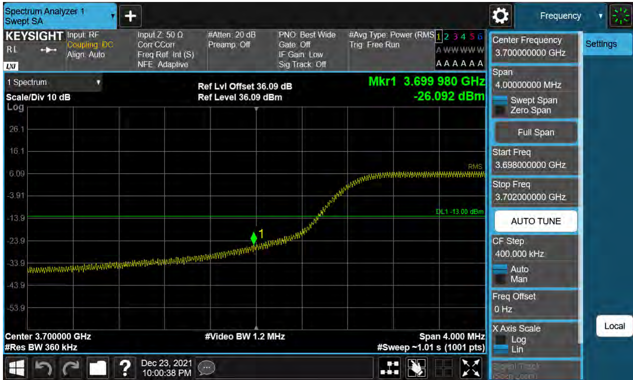
Sub6 n77. Low Band Edge Plot (40 M BW Ch.648000 BPSK FullIRB)(1)
