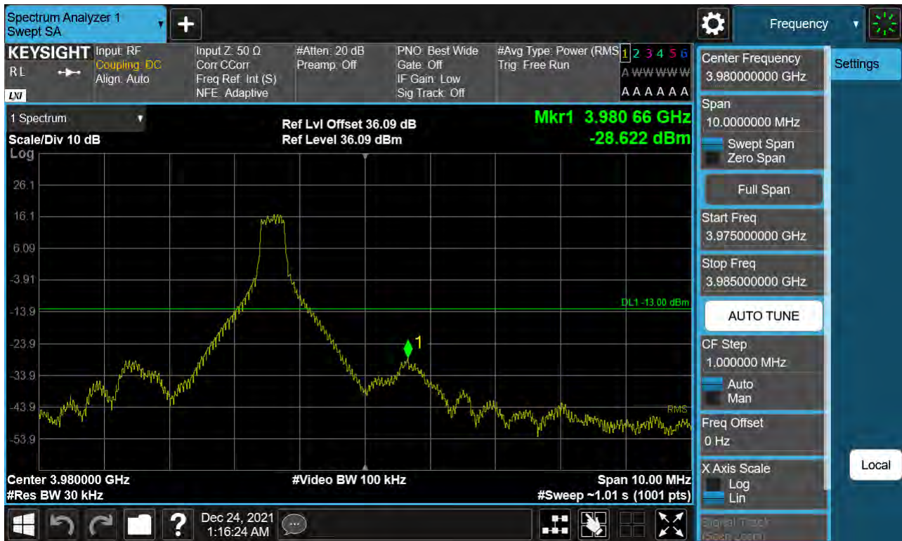
Sub6 n77. High Band Edge Plot (100 M BW Ch.662000 BPSK 1RB)(1)
