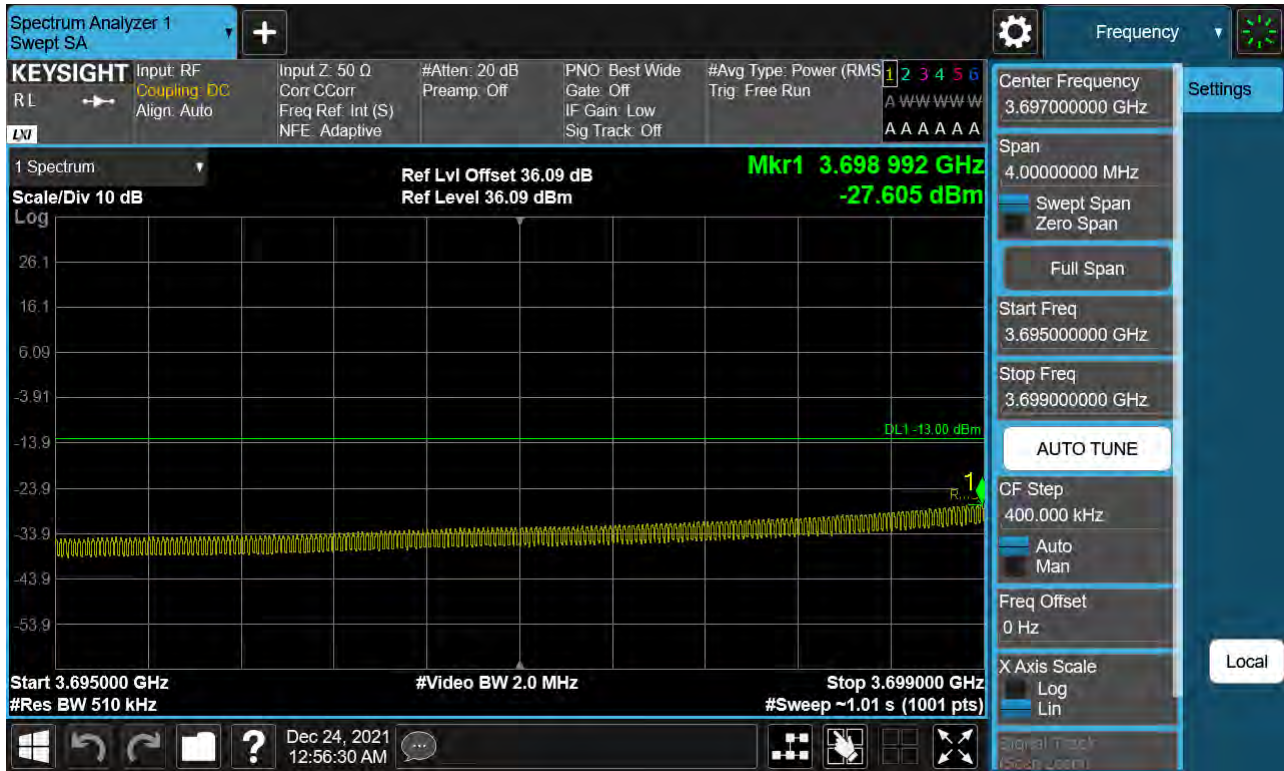
Sub6 n77. Low Band Edge Plot (100 M BW Ch.650000 BPSK FullRB)(2)
