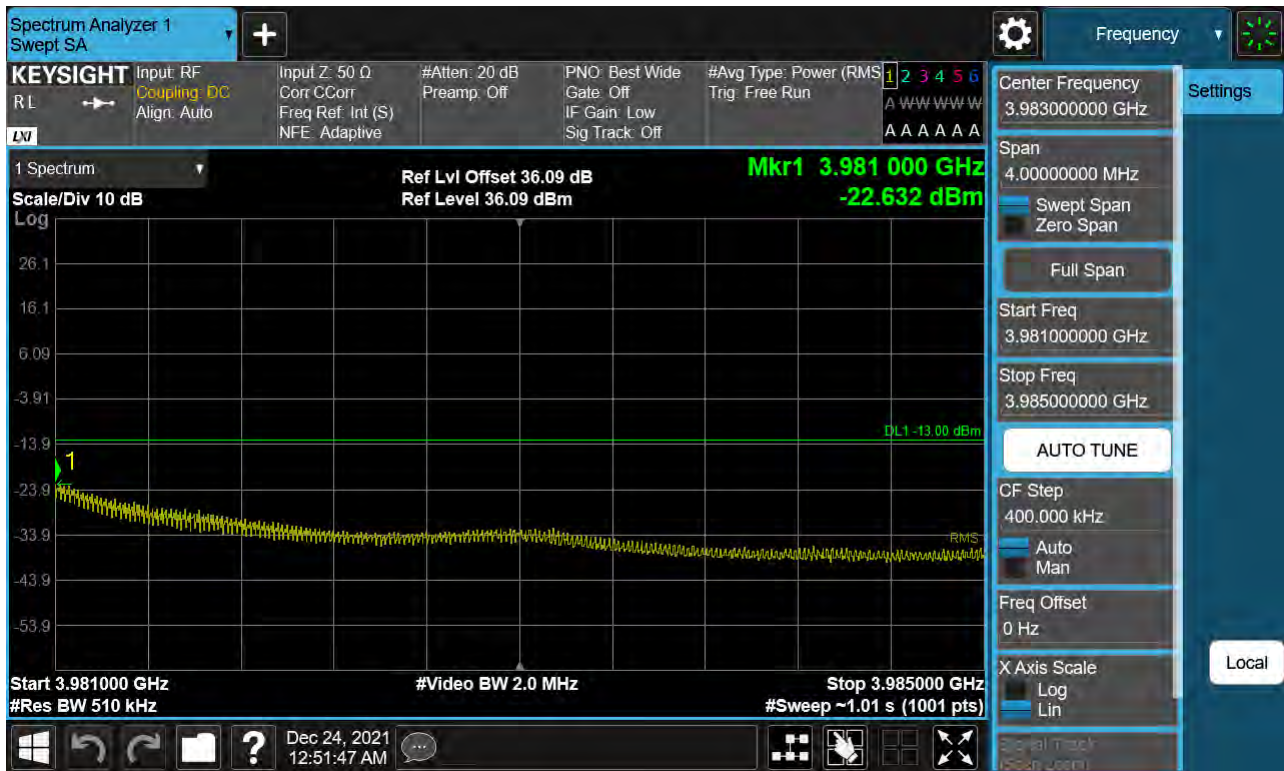
Sub6 n77. High Band Edge Plot (90 M BW Ch.662332 BPSK 1RB)(2)
