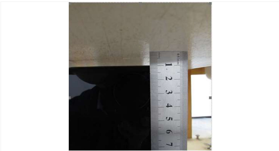
Distance of 10 mm from the EUT
