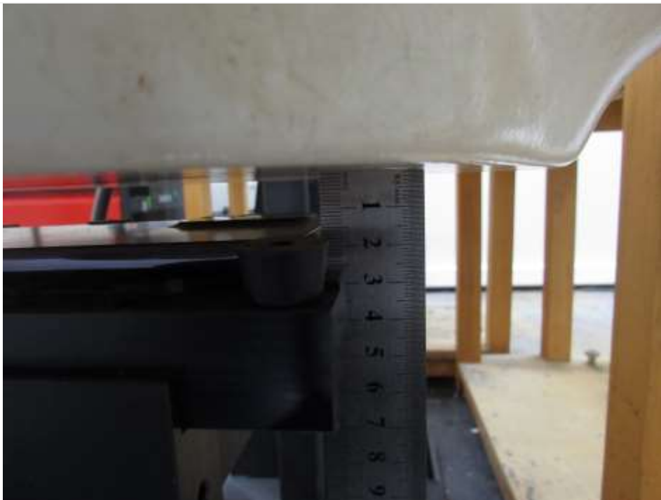
Distance of 15 mm from the EUT
