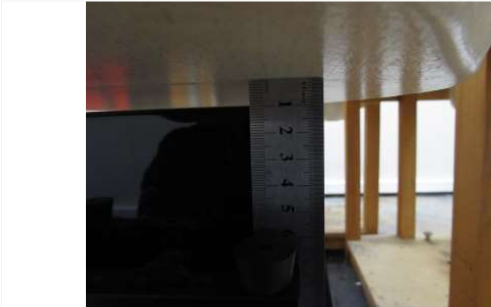
Distance of 10 mm from the EUT
