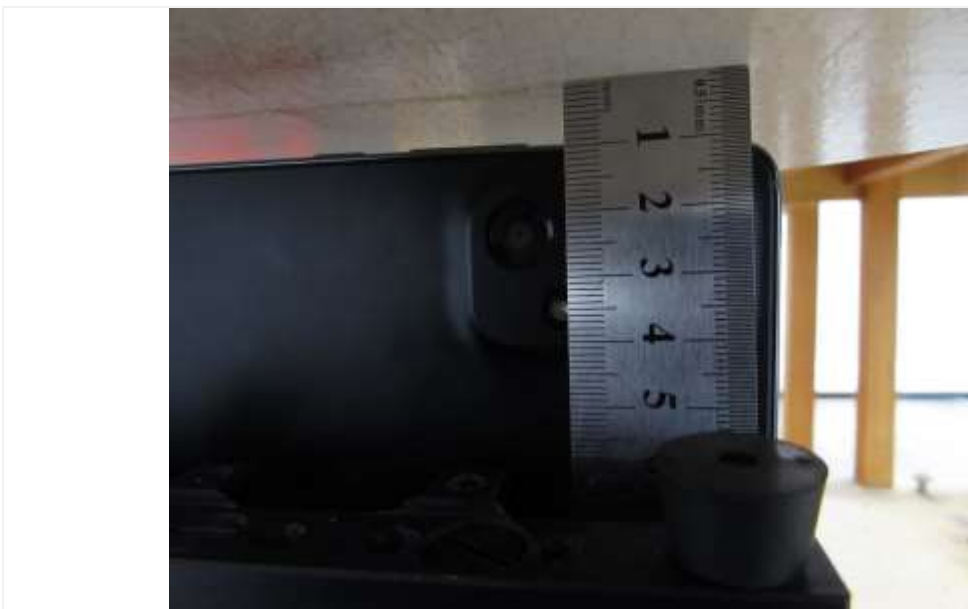
Distance of 10 mm from the EUT
