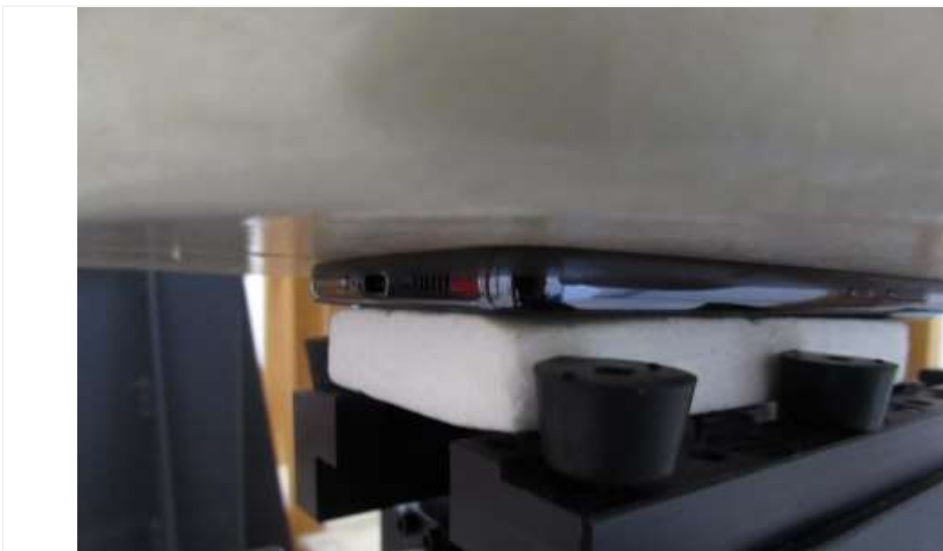
Distance of 0 mm from the EUT
