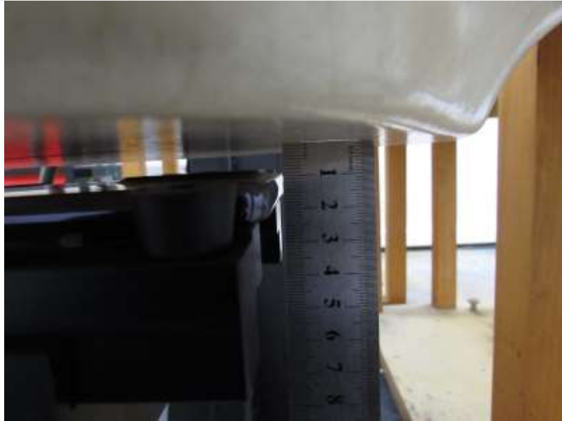
Distance of 10 mm from the EUT
