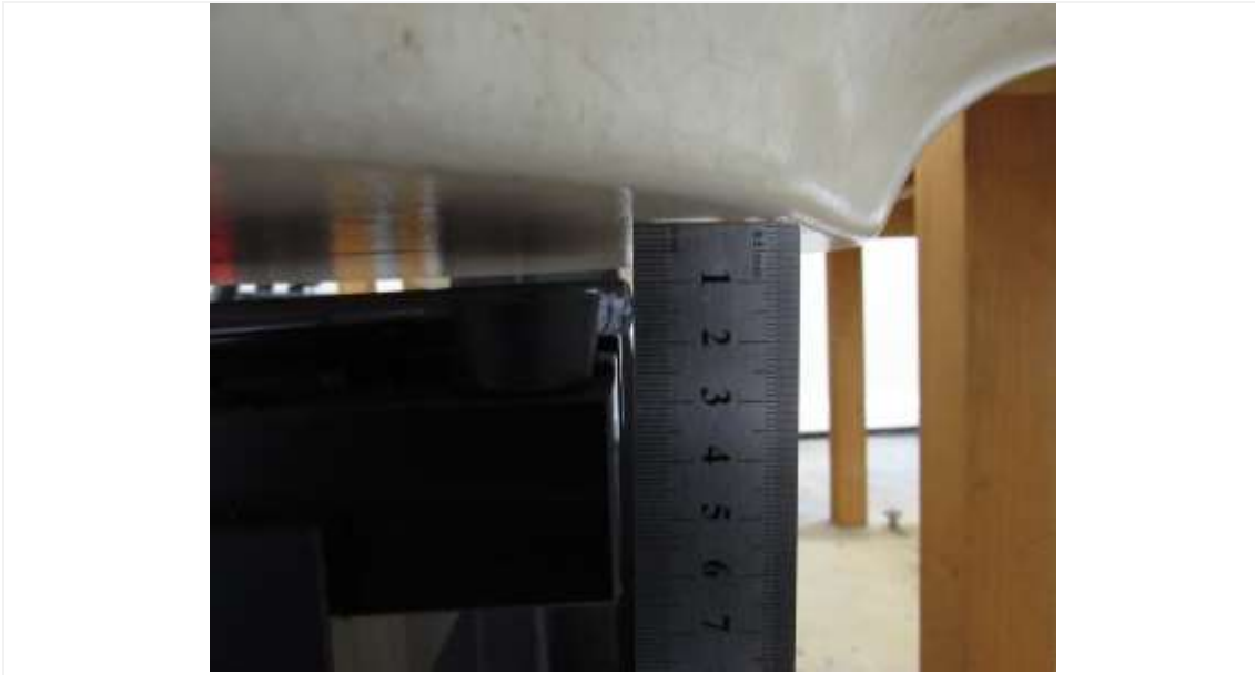
Distance of 10 mm from the EUT
