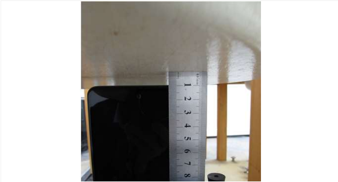
Distance of 10 mm from the EUT
