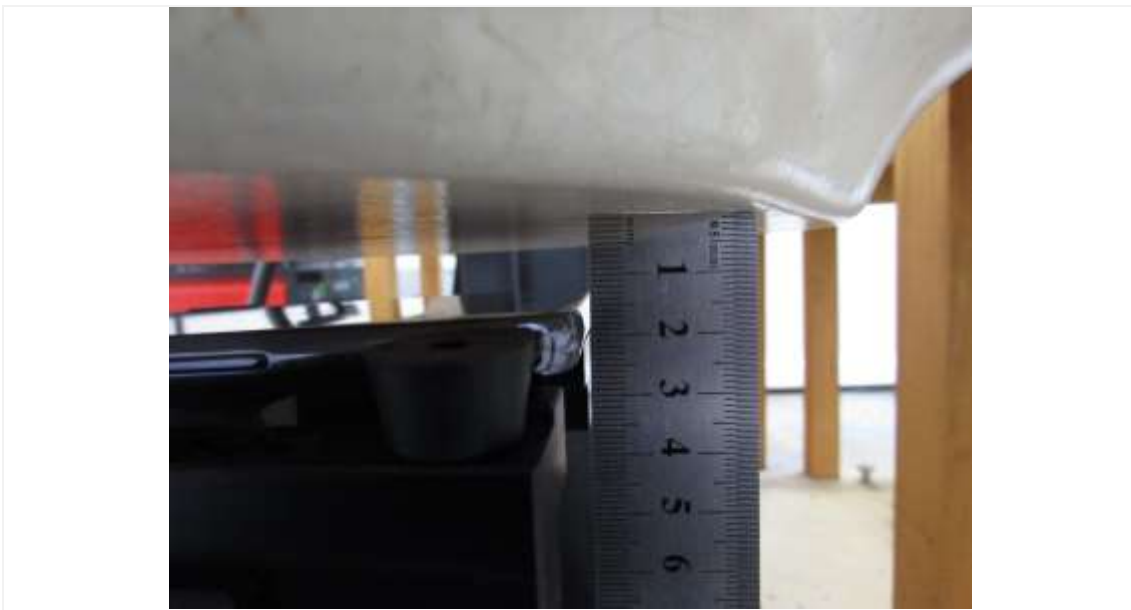
Distance of 15 mm from the EUT
