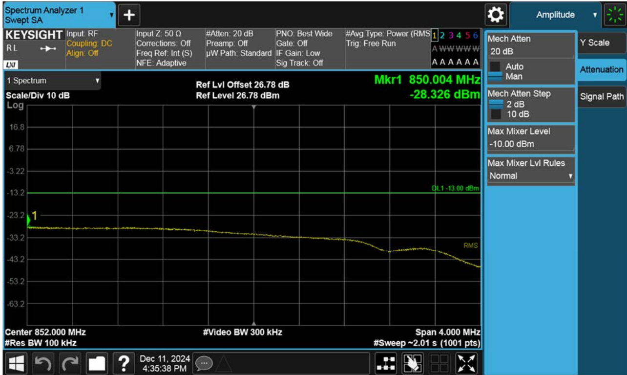
BAND 26. Upper Extended Band Edge Plot (10 M BW Ch.26990 QPSK_RB50_0)
