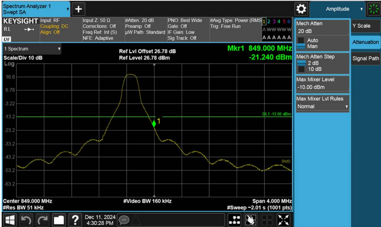
BAND 26. Upper Band Edge Plot (5 M BW Ch.27015 QPSK_RB1_Offset 24)
