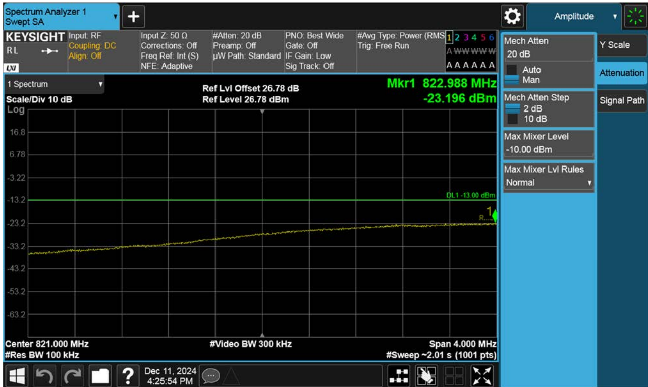
BAND 26. Lower Extended Band Edge Plot (5 M BW Ch.26815 QPSK_RB25_0)
