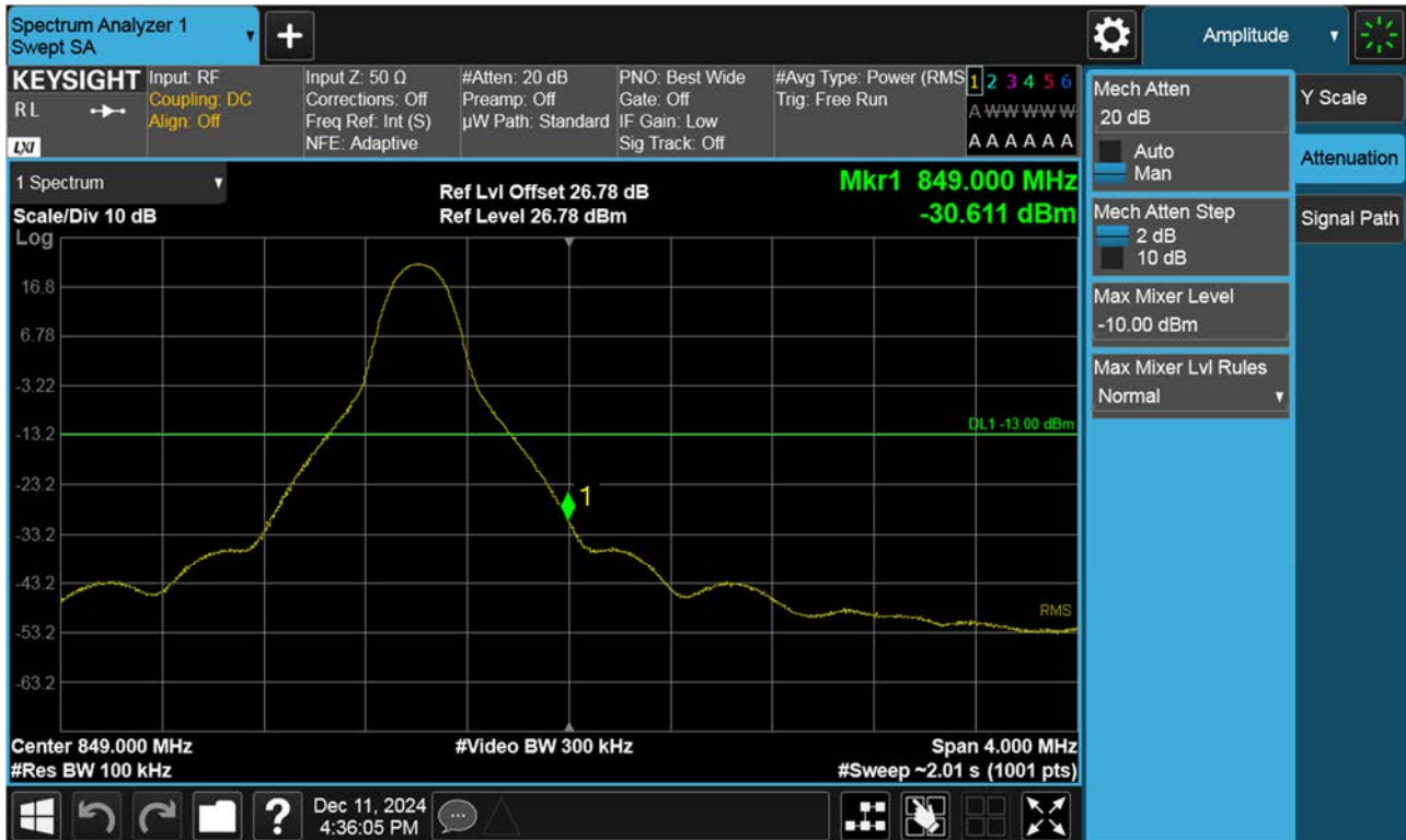
BAND 26. Upper Band Edge Plot (10 M BW Ch.26990 QPSK_RB1_Offset 49)
