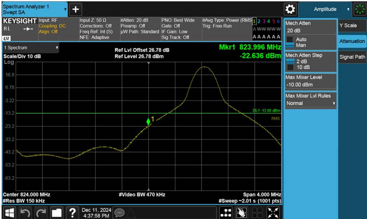
BAND 26. Lower Band Edge Plot (15 M BW Ch.26865 QPSK_RB1_Offset 0)
