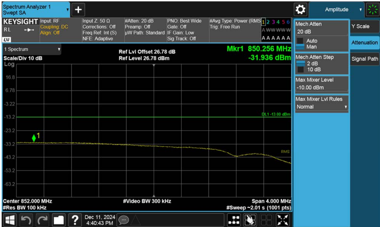
BAND 26. Upper Extended Band Edge Plot (15 M BW Ch.26965 QPSK_RB75_0)
