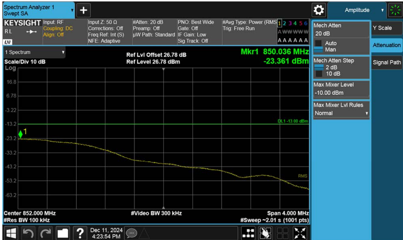
BAND 26. Upper Extended Band Edge Plot (3 M BW Ch.27025 QPSK_RB15_0)
