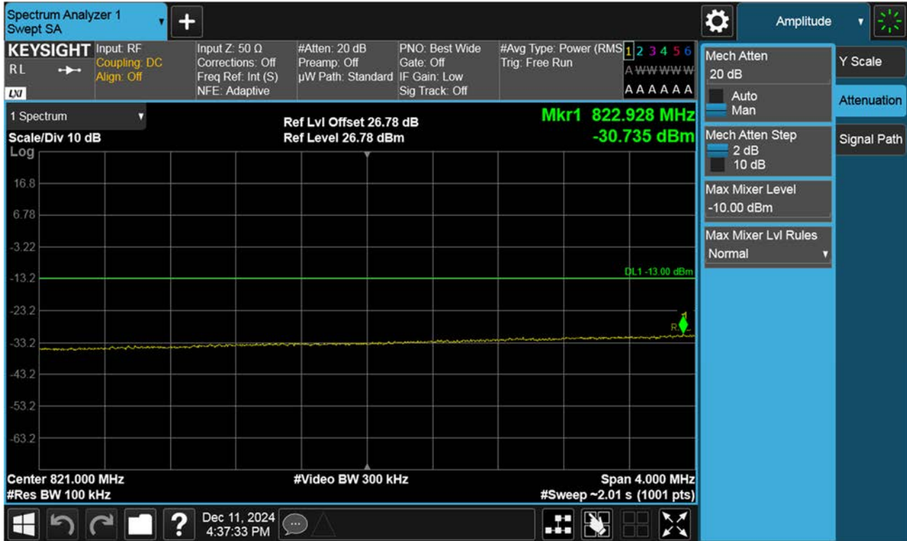
BAND 26. Lower Extended Band Edge Plot (15 M BW Ch.26865 QPSK_RB75_0)
