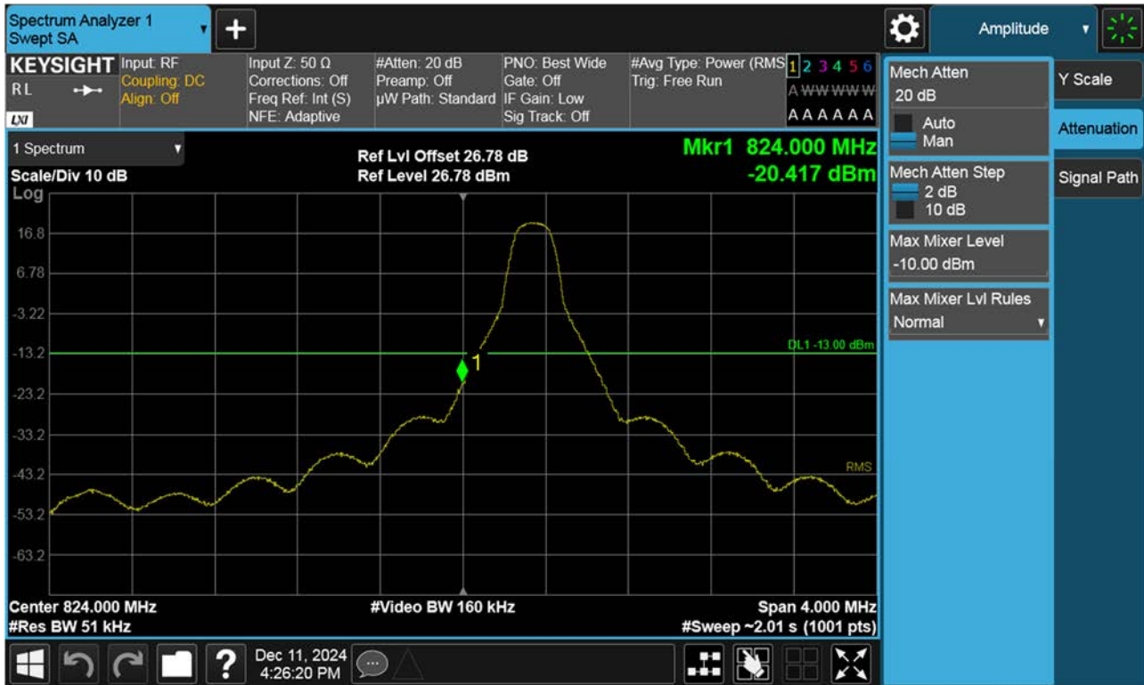
BAND 26. Lower Band Edge Plot (5 M BW Ch.26815 QPSK_RB1_Offset 0)
