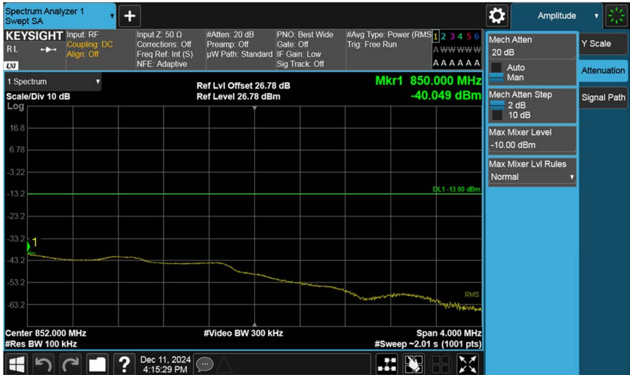
BAND 26. Upper Extended Band Edge Plot (1.4 M BW Ch.27033 QPSK_RB6_0)
