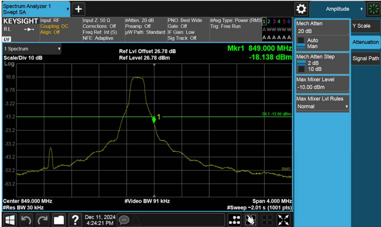
BAND 26. Upper Band Edge Plot (3 M BW Ch.27025 QPSK_RB1_Offset 14)
