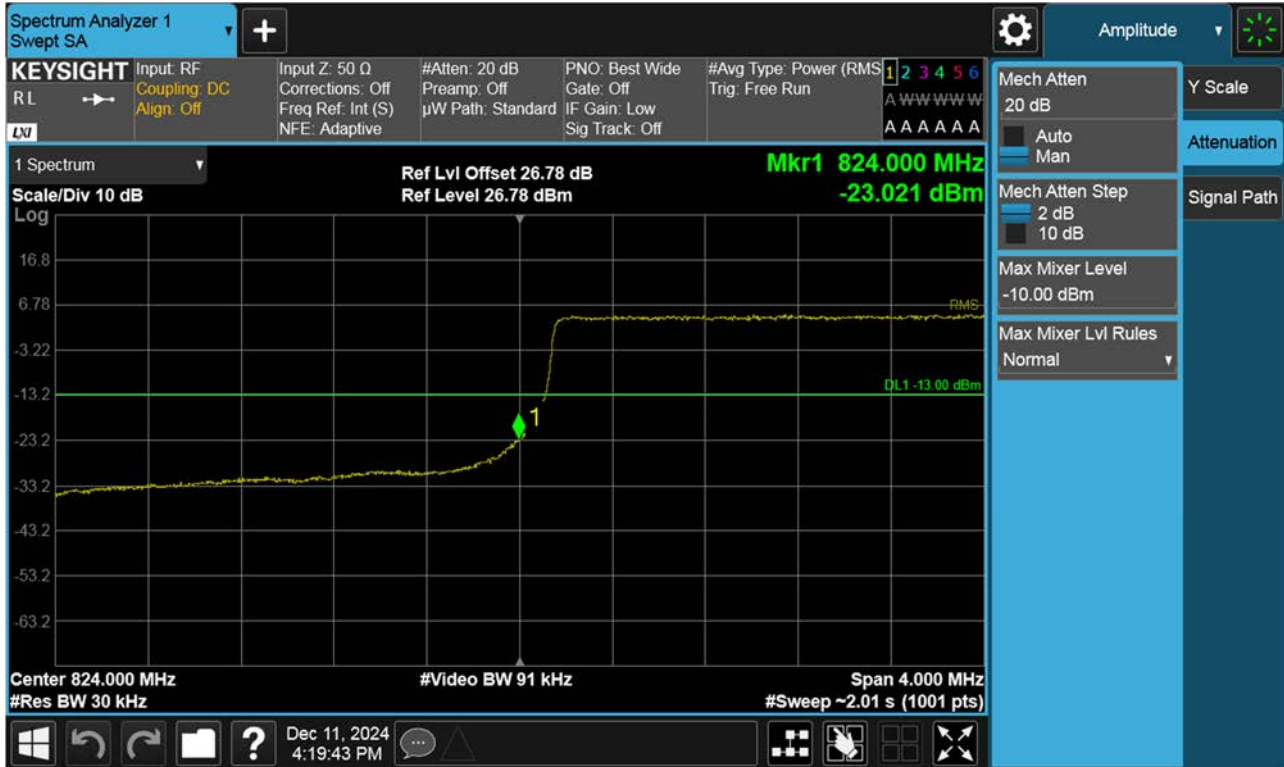
BAND 26. Lower Band Edge Plot (3 M BW Ch.26805 QPSK_RB15_Offset 0)
