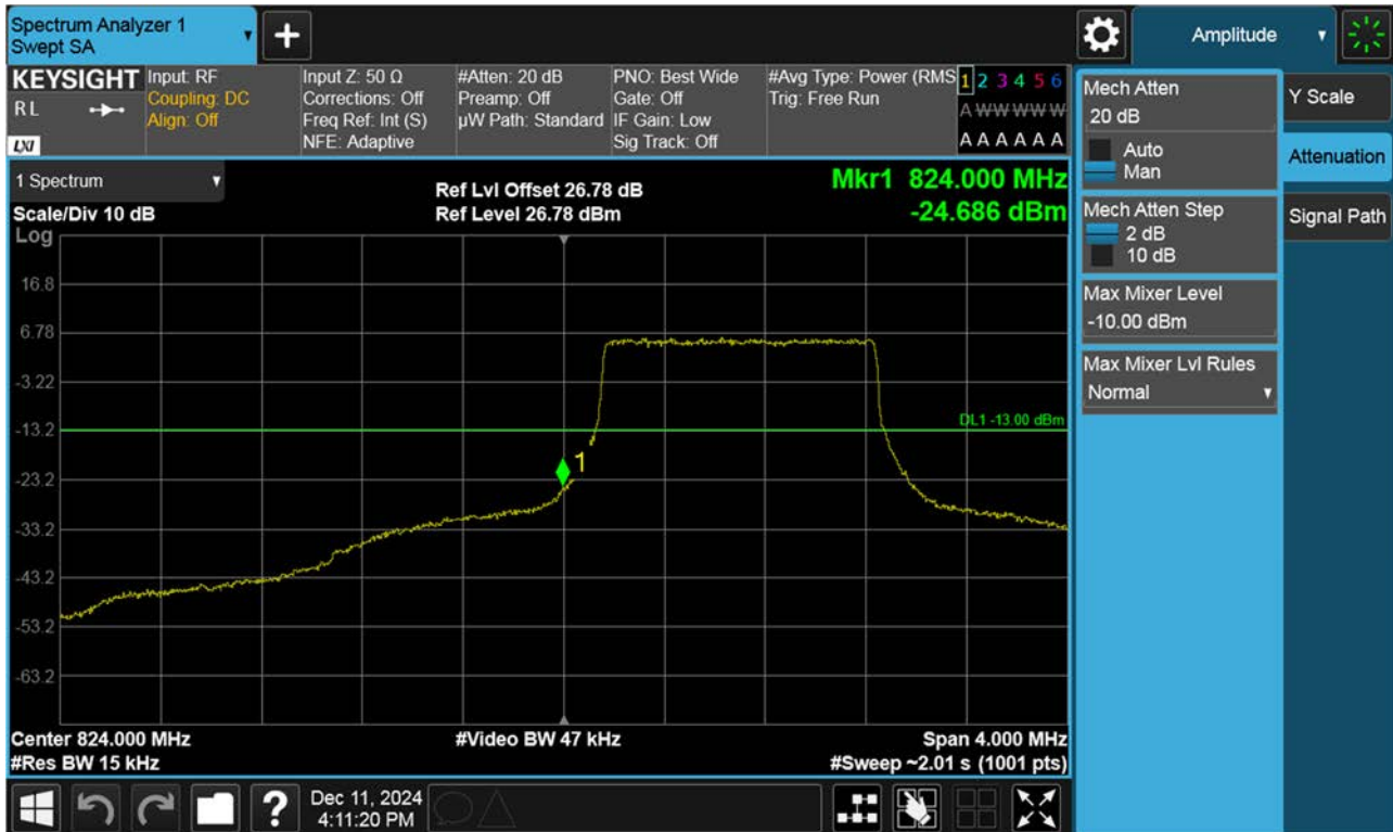
BAND 26. Lower Band Edge Plot (1.4 M BW Ch.26797 QPSK_RB6_Offset 0)
