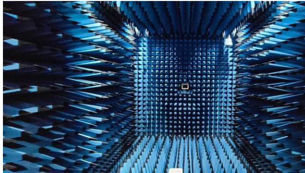
Figure 2: Geometry of Anechoic Chamber for Radiation patterns.
