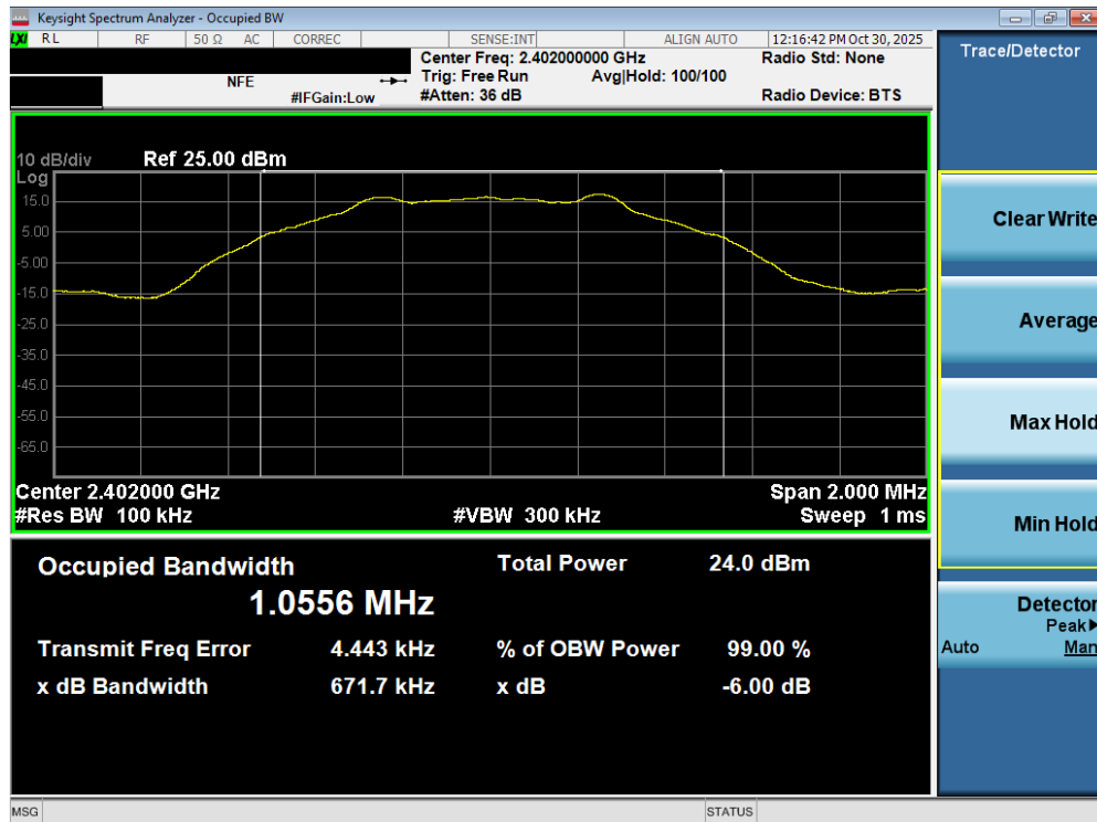
Plot 7-7. 6dB Bandwidth Plot (Bluetooth (LE), 1Mbps – Ch. 37)
