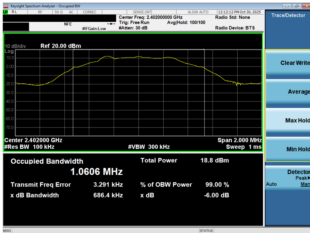
Plot 7-4. 6dB Bandwidth Plot (Bluetooth (LE), 500kbps – Ch. 37)
