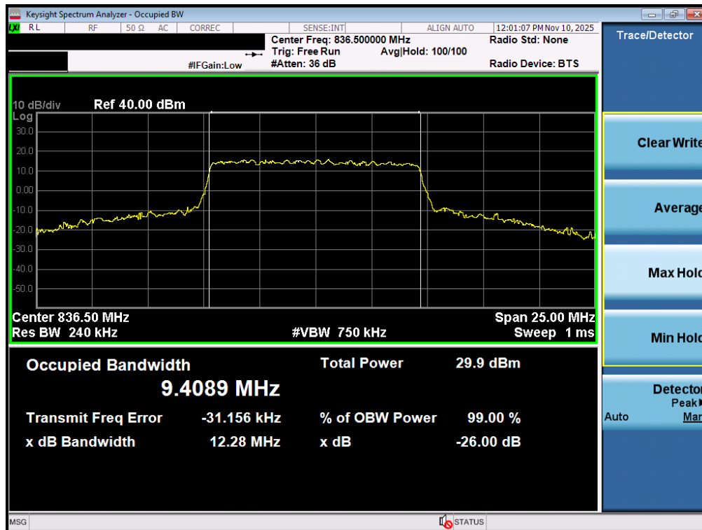
Plot 7-18. Occupied Bandwidth Plot (NR Band n5 - 10MHz QPSK - Full RB - Ant1)
