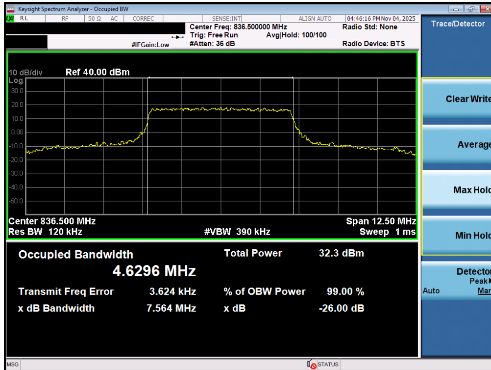
Plot 7-6. Occupied Bandwidth Plot (LTE Band 26/5 - 5MHz 16-QAM - Full RB - Ant1)
