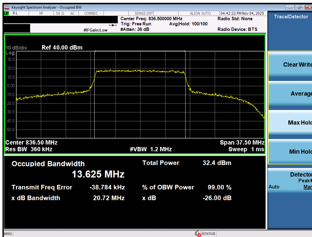
Plot 7-2. Occupied Bandwidth Plot (LTE Band 26 - 15MHz 16-QAM - Full RB - Ant1)
