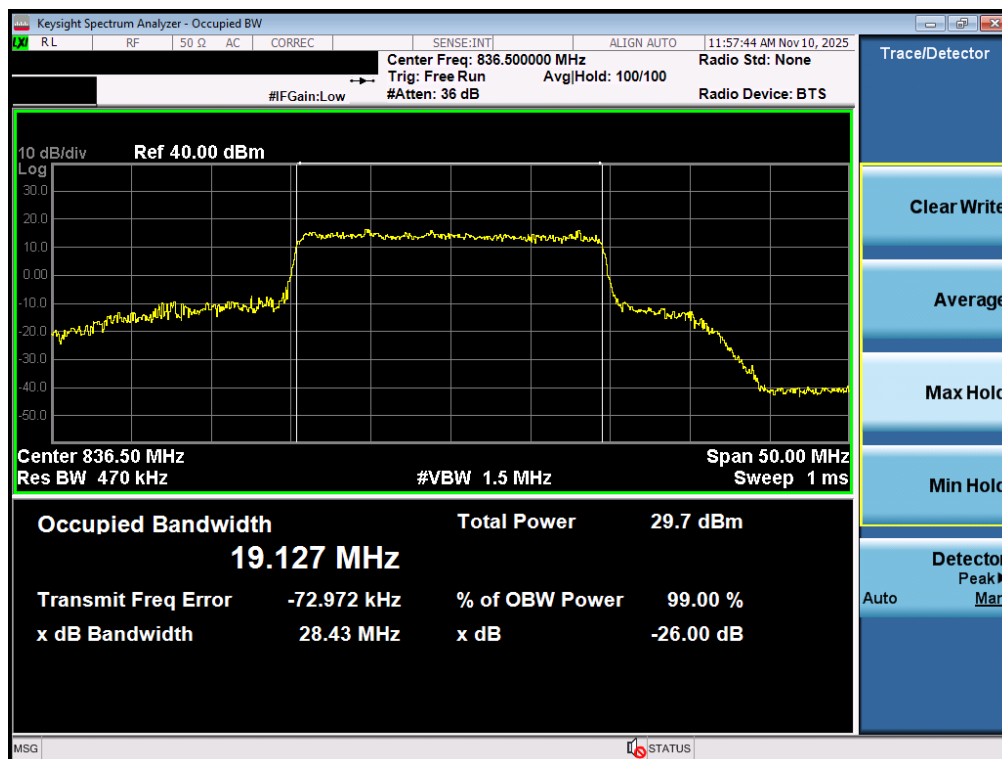
Plot 7-12. Occupied Bandwidth Plot (NR Band n5 - 20MHz QPSK - Full RB - Ant1)
