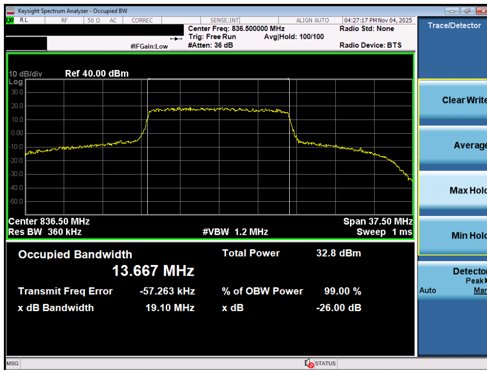
Plot 7-1. Occupied Bandwidth Plot (LTE Band 26 - 15MHz QPSK - Full RB - Ant1)
