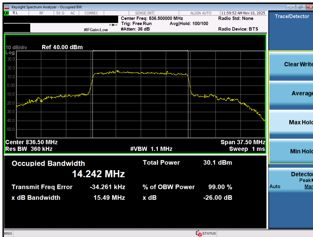
Plot 7-16. Occupied Bandwidth Plot (NR Band n5 - 15MHz 16-QAM - Full RB - Ant1)
