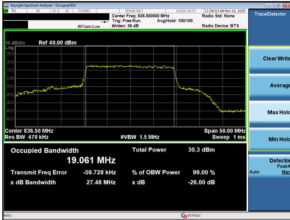
Plot 7-13. Occupied Bandwidth Plot (NR Band n5 - 20MHz 16-QAM - Full RB - Ant1)
