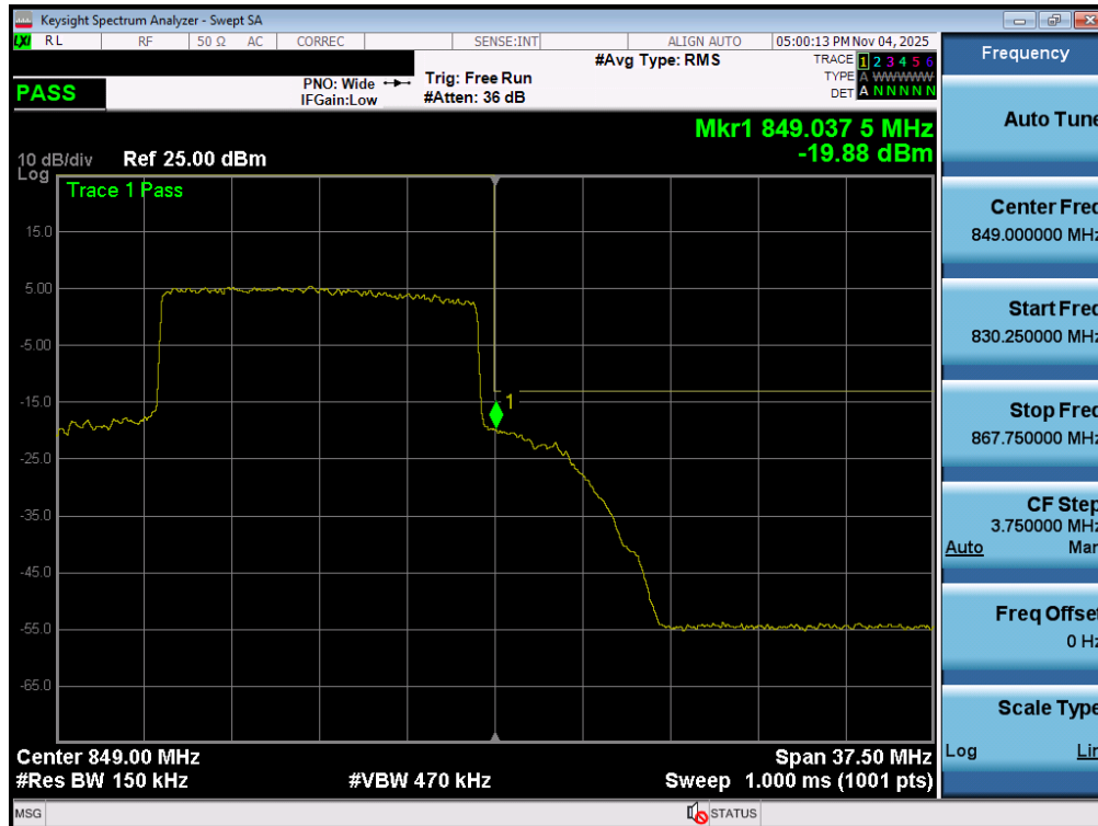
Plot 7-124. Upper Band Edge Plot (LTE Band 26 - 15MHz QPSK – Full RB - Ant1)
