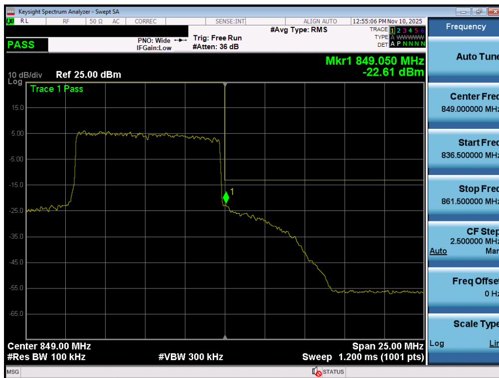
Plot 7-138. Upper Band Edge Plot (NR Band n5 - 10.0MHz - Full RB - Ant1)
