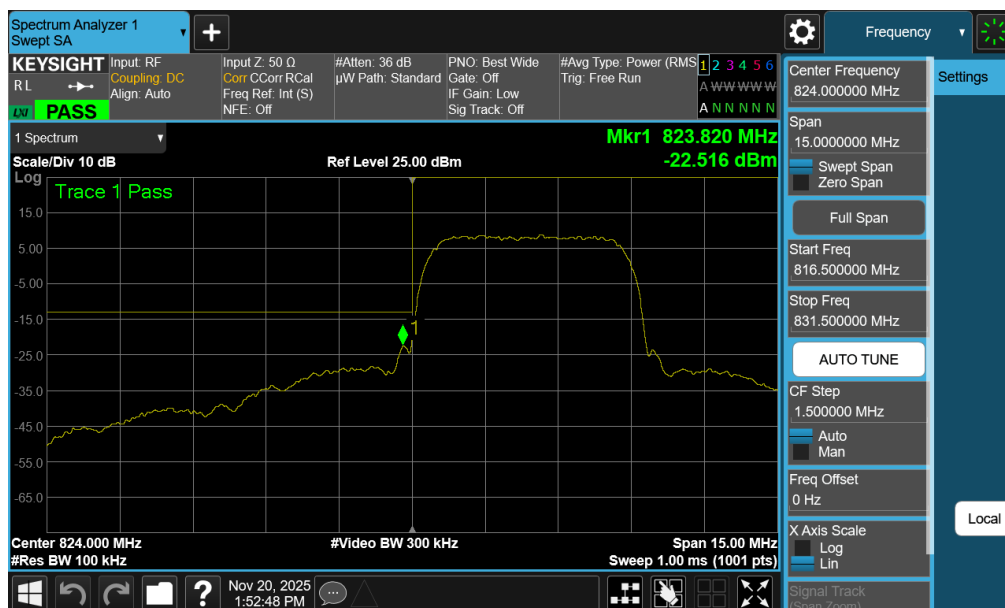
Plot 7-143. Lower Band Edge Plot (WCDMA Cell – Ch. 4132 – Ant1)
