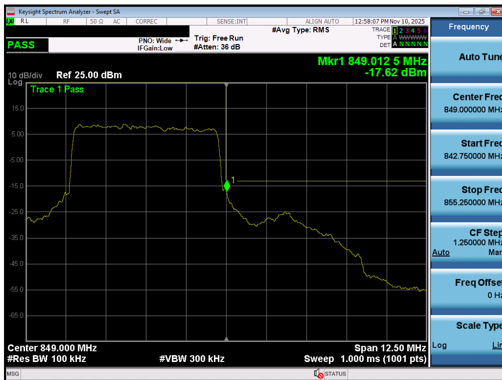
Plot 7-140. Upper Band Edge Plot (NR Band n5 – 5.0MHz - Full RB
