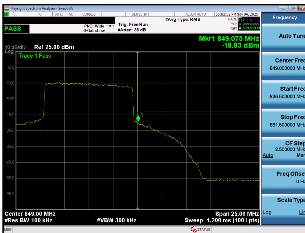
Plot 7-126. Upper Band Edge Plot (LTE Band 26/5 - 10MHz QPSK – Full RB - Ant1)
