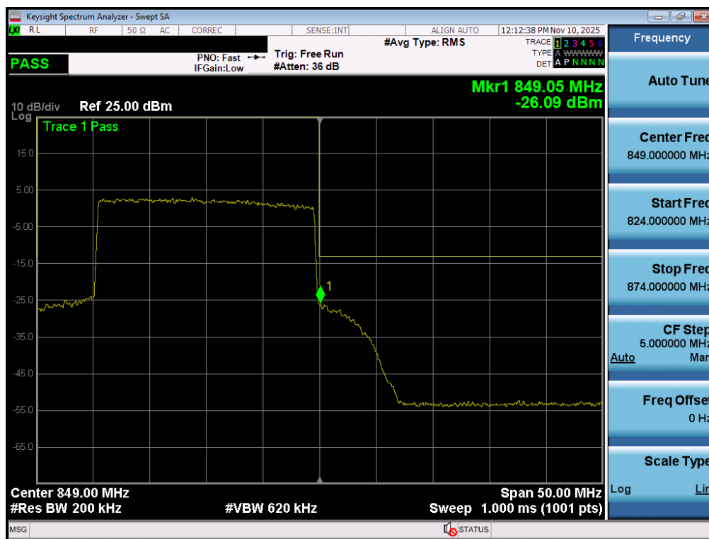
Plot 7-134. Upper Band Edge Plot (NR Band n5 – 20.0MHz - Full RB - Ant1)
