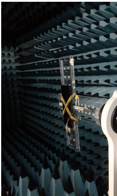
Figure 1: Geometry for SM-A576B/DS for Radiation patterns.
