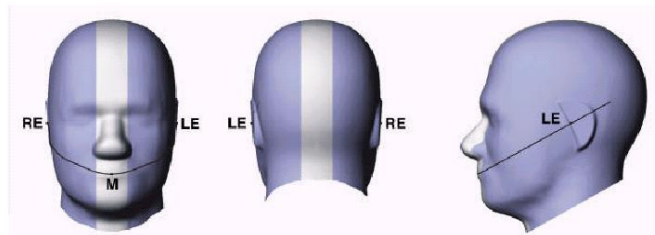
Figure 6-2 Front, back and side view of SAM Twin Phantom
