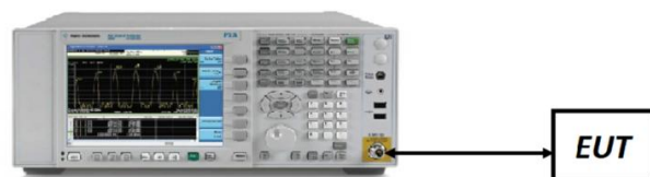
Figure 7-1. Test Instrument & Measurement Setup
