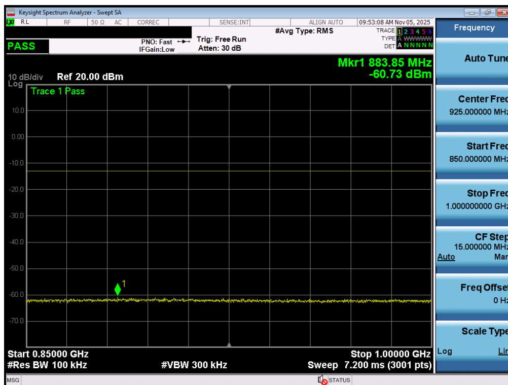
Plot 7-58. Conducted Spurious Plot (LTE Band 26 - 15MHz QPSK - 1 RB - High Channel – Ant1)
