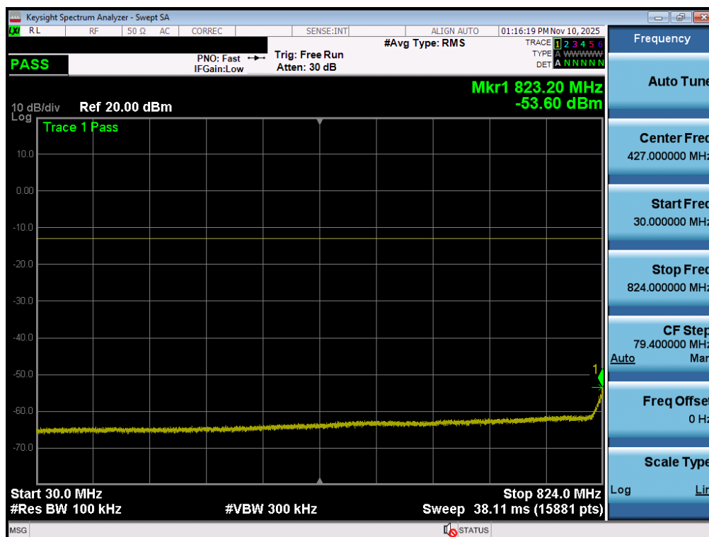
Plot 7-66. Conducted Spurious Plot (NR Band n5 - 20.0MHz - 1 RB - High Channel - Ant1)
