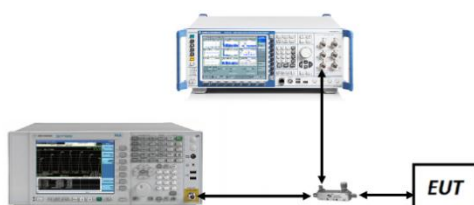
Figure 7-5. Test Instrument & Measurement Setup
