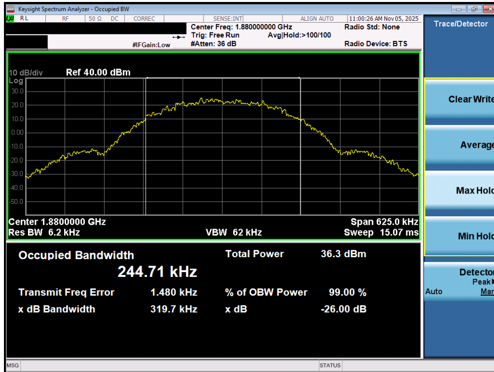
Plot 7-1. Occupied Bandwidth Plot (GPRS, Ch. 661 - Ant1)
