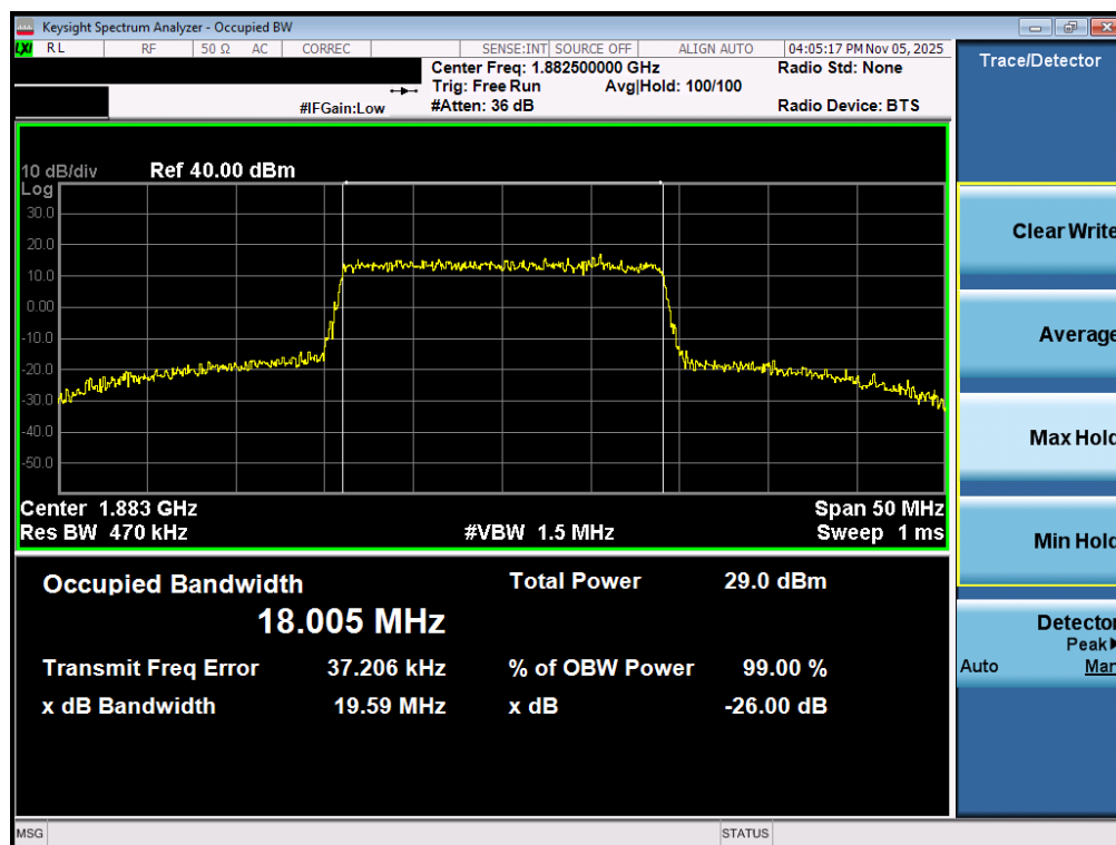
Plot 7-16. Occupied Bandwidth Plot (LTE Band 2 - 20MHz 16-QAM - Full RB - Ant2)
