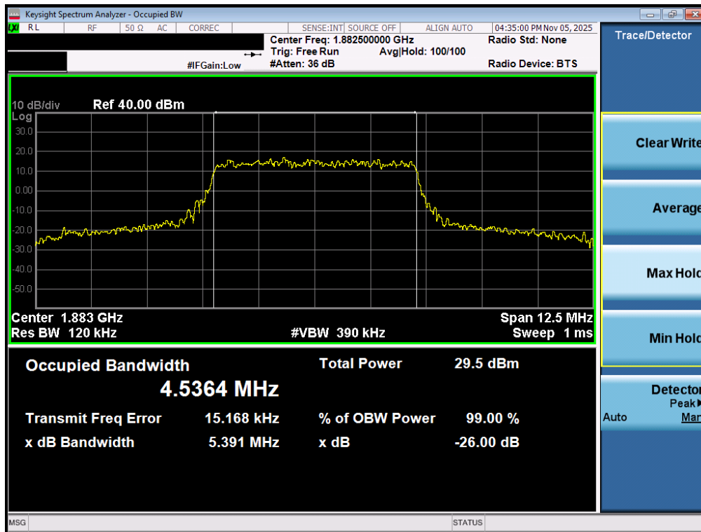
Plot 7-21. Occupied Bandwidth Plot (LTE Band 2 - 5MHz QPSK - Full RB - Ant2)
