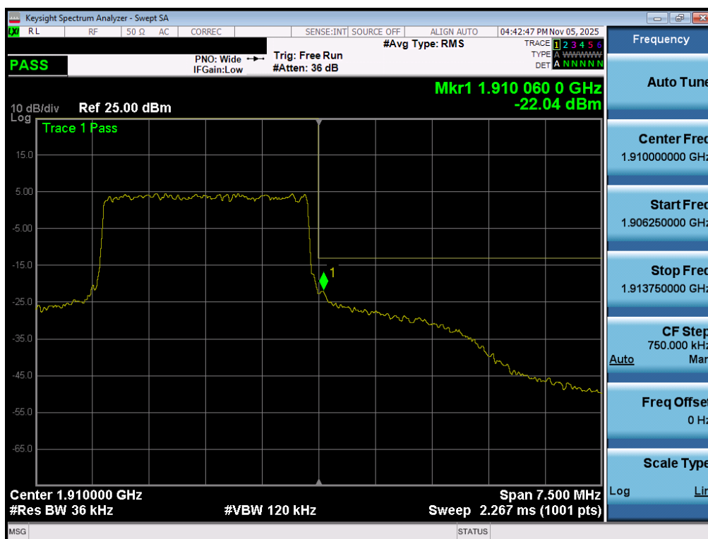
Plot 7-46. Upper Band Edge Plot (LTE Band 2 - 3MHz QPSK – Full RB – Ant2)
