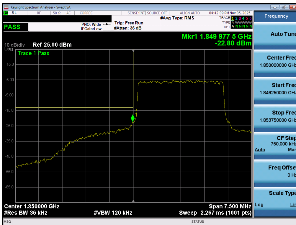
Plot 7-44. Lower Band Edge Plot (LTE Band 2 - 3MHz QPSK – Full RB – Ant2)
