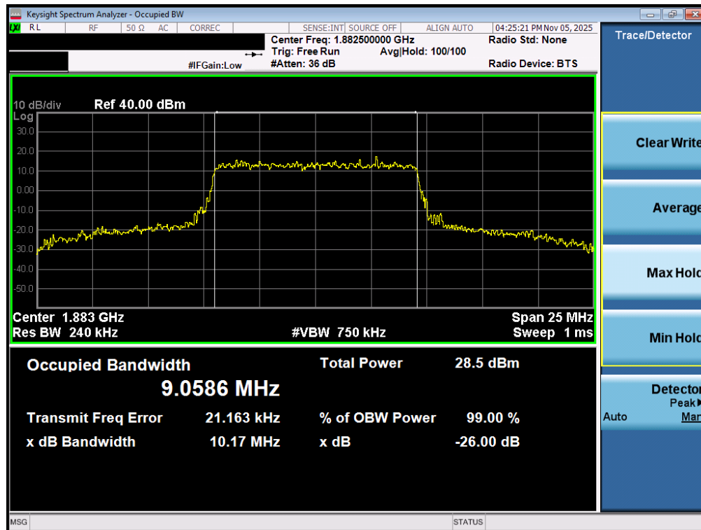
Plot 7-20. Occupied Bandwidth Plot (LTE Band 2 - 10MHz 16-QAM - Full RB - Ant2)
