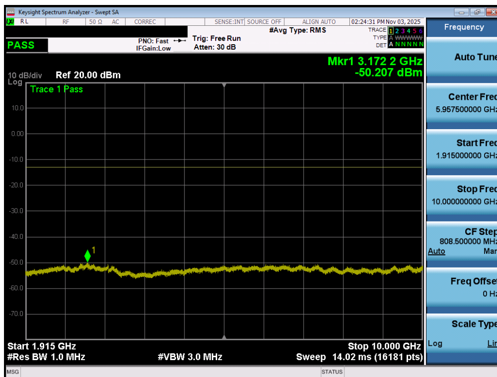
Plot 7-31. Conducted Spurious Plot (LTE Band 2 - 20MHz QPSK - 1RB - Low Channel - Ant1)
