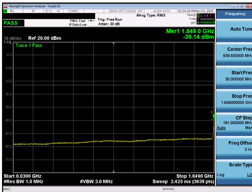
Plot 7-30. Conducted Spurious Plot (LTE Band 2 - 20MHz QPSK - 1RB - Low Channel - Ant1)
