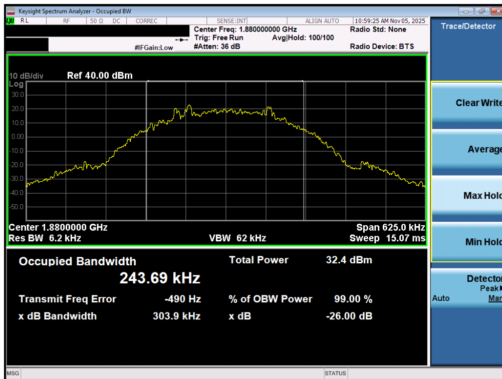
Plot 7-2. Occupied Bandwidth Plot (EDGE, Ch. 661 - Ant1)
