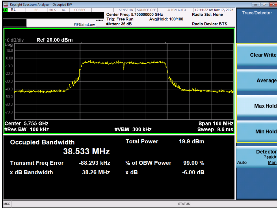
Plot 7-19. 6dB Bandwidth Plot MIMO ANT1 (40MHz BW 802.11ax (UNII Band 3) – Ch. 151)
