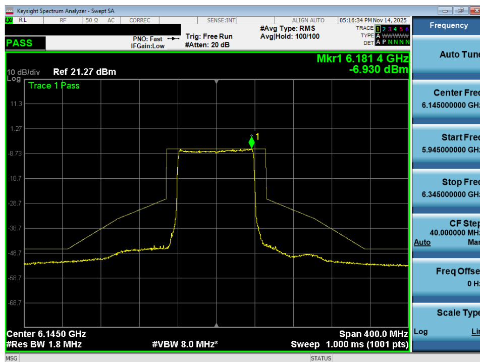
Plot 7-24. In Band Emissions Plot MIMO ANT2 (80MHz 802.11ax (UNII Band 5) – Ch. 39) – LPI/SP
