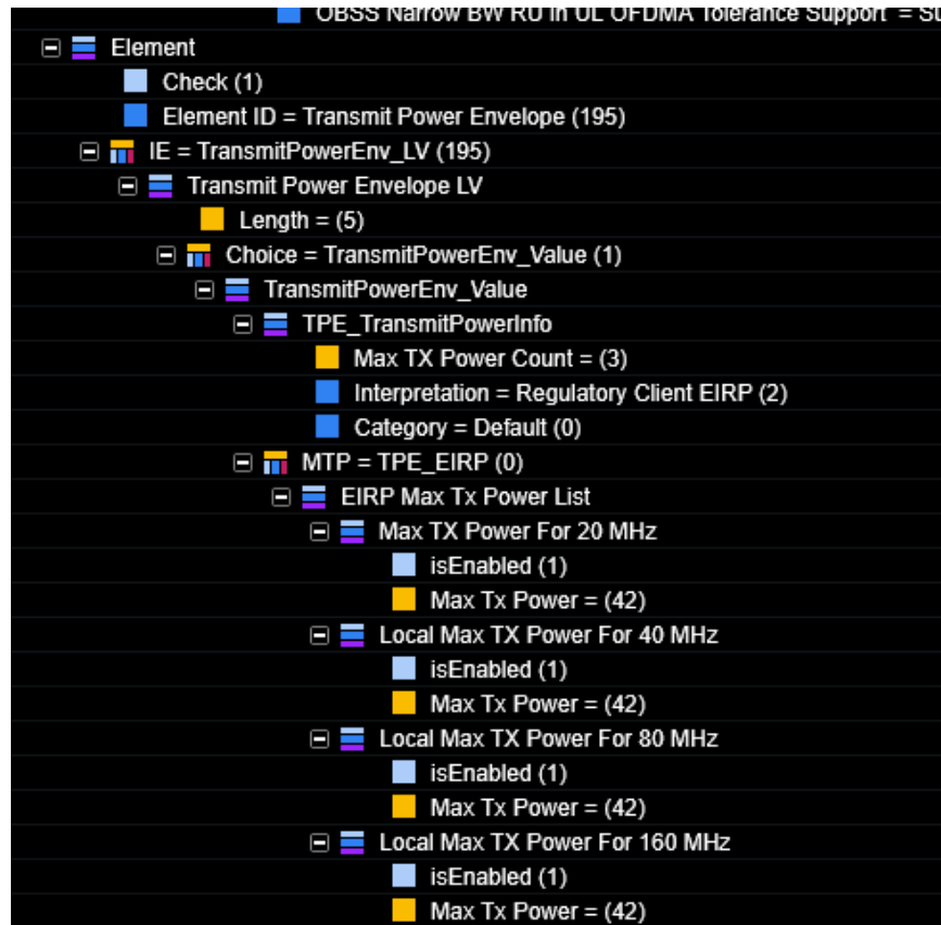
Figure 7-9. Callbox Power Authorization – 21.00 dBm
