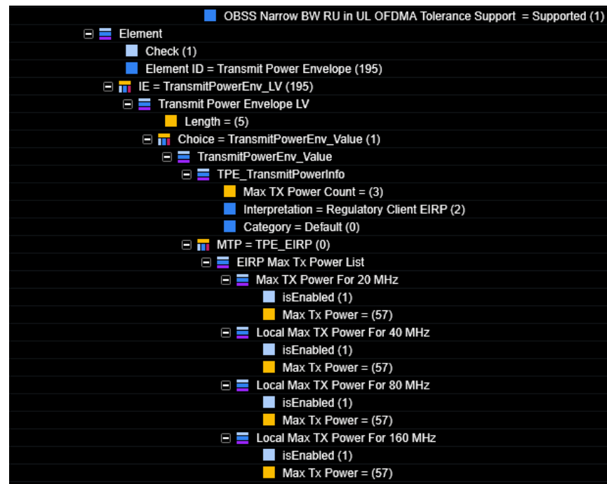
Figure 7-8. Callbox Power Authorization – 28.50 dBm
