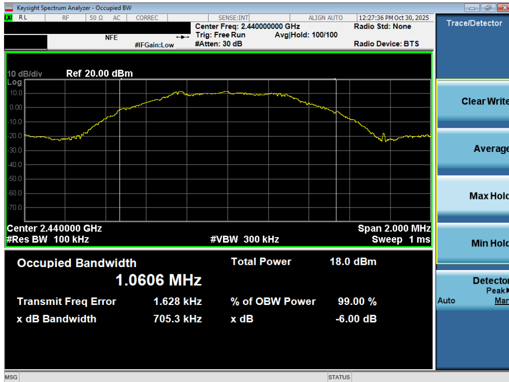
Plot 7-5. 6dB Bandwidth Plot (Bluetooth (LE), 500kbps – Ch. 17)
