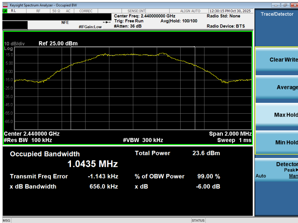
Plot 7-8. 6dB Bandwidth Plot (Bluetooth (LE), 1Mbps – Ch. 17)
