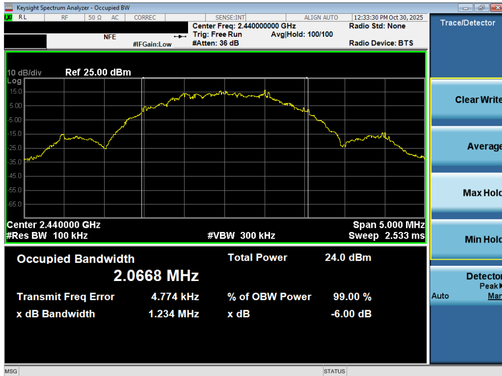
Plot 7-11. 6dB Bandwidth Plot (Bluetooth (LE), 2Mbps – Ch. 17)
