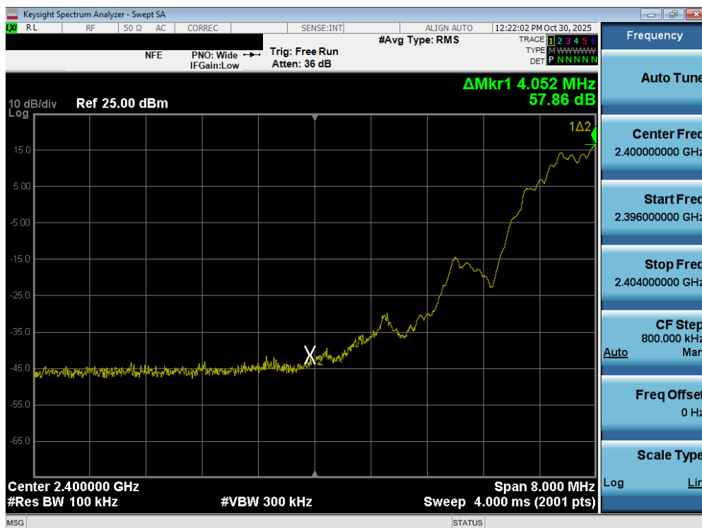
Plot 7-55. Band Edge Plot (Bluetooth (LE), 2Mbps – Ch. 0)
