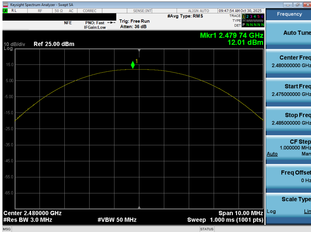
Plot 7-27. Peak Power Plot (Bluetooth (LE), 125kbps – Ch. 39)
