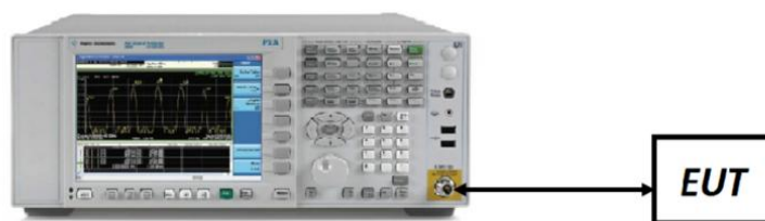
Figure 7-3. Test Instrument & Measurement Setup
