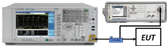
Figure 7-2. Test Instrument & Measurement Setup
