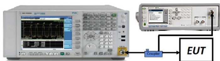
Figure 7-1. Test Instrument & Measurement Setup
