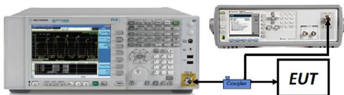
Figure 7-3. Test Instrument & Measurement Setup
