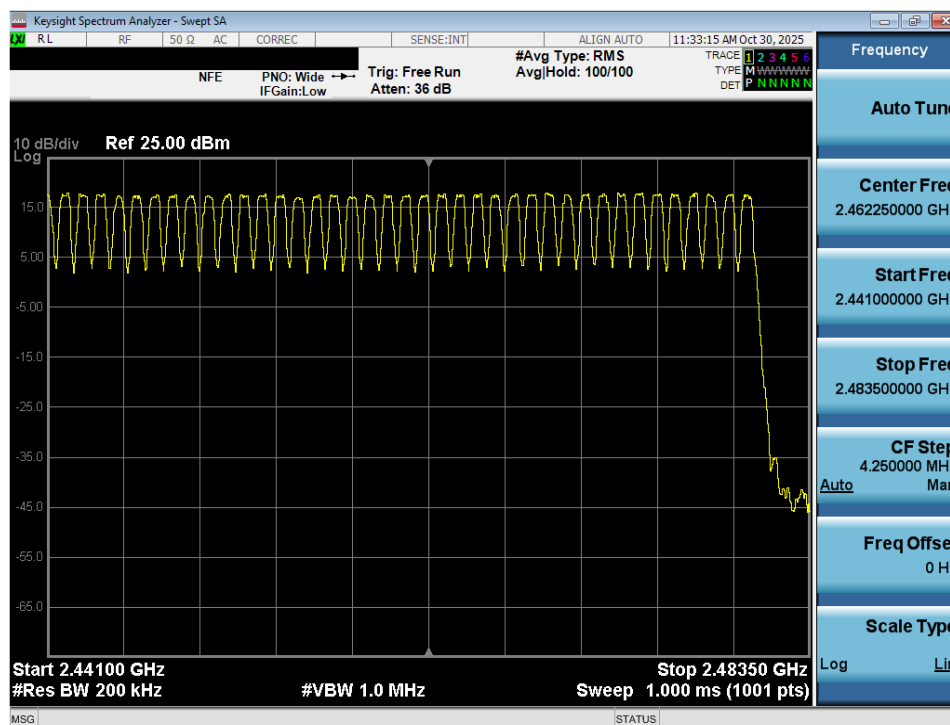
Plot 7-35. High End Spectrum Channel Hopping Plot (Bluetooth) – Ant 1
